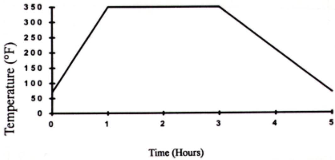
Figure 5.2 Cure cycle for composites [98].
