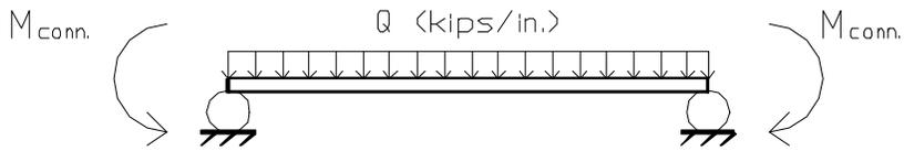
(b) Configuration of an Idealized Double Angle Connection
