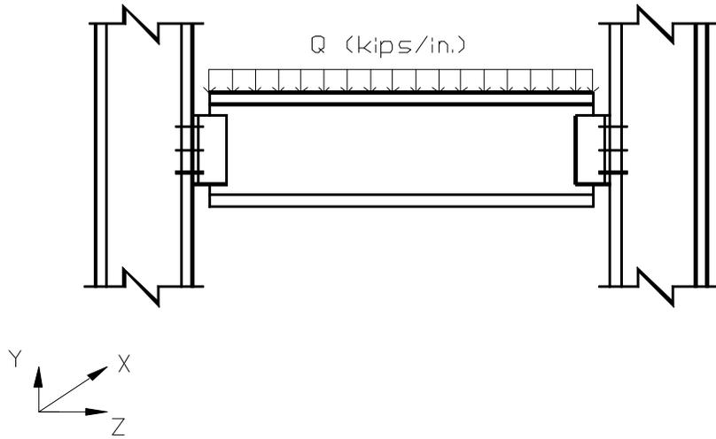
(a) Configuration of a Double Angle Connection
