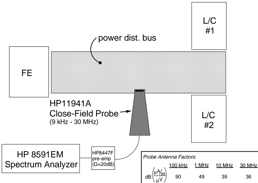
**Fig. 6.8 Experimental B-field measurement setup.**
