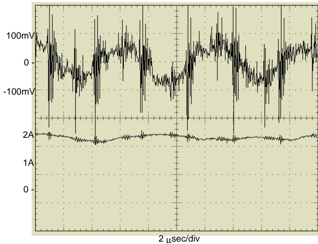
**Fig. 6.11** DC DPS bus voltage and current. The bus voltage is AC coupled.
