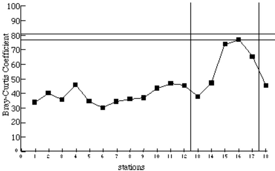
FIG. 17. Comparison of Bray-Curtis Coefficient along Peak Creek Stations 1-18 with the reference condition for each method (PIBS top panel, KSS bottom panel). Horizontal lines denote 95% confidence interval calculated from the 5 PIBS or KSS samples taken from the Peak Creek Reference Station. Vertical lines separate impaired stations (1-12,18) from relatively unimpaired stations (13-17).
