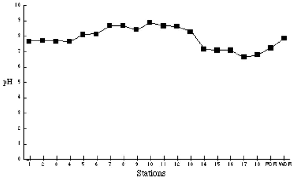
FIG. 3. Alkalinity (mg/L CaCO<sub>3</sub>) and pH at Peak Creek Stations 1-18, Peak Creek Reference Station (PCR), and Wolf Creek Reference Station (WCR).
