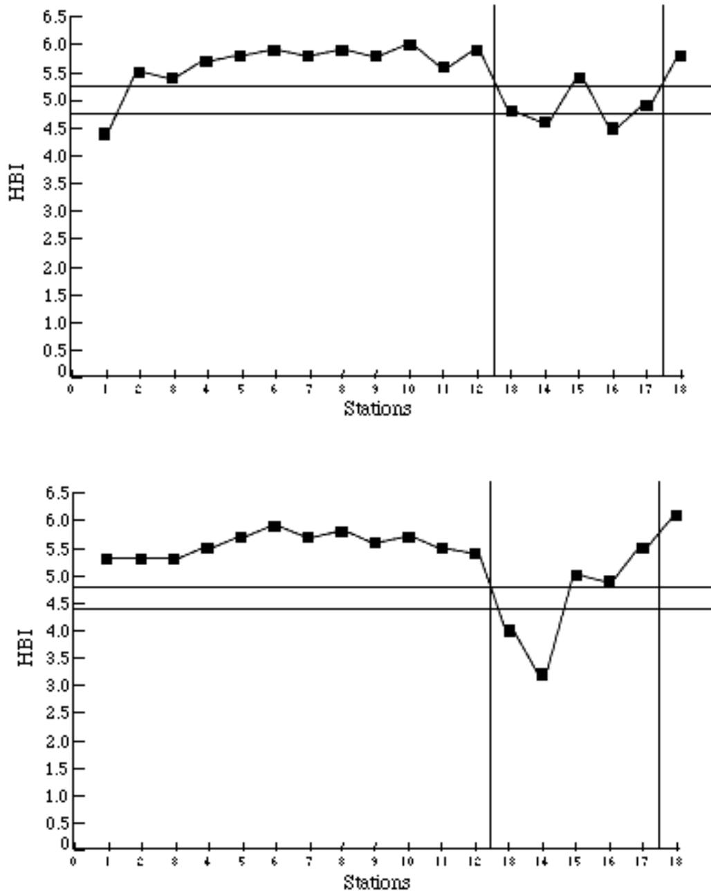
FIG. 12. Comparison of HBI along Peak Creek Stations 1-18 with the reference condition for each method (PIBS top panel, KSS bottom panel). Horizontal lines denote 95% confidence interval calculated from the 5 PIBS or KSS samples taken from the Peak Creek Reference Station. Vertical lines separate impaired stations (1-12,18) from relatively unimpaired stations (13-17).
