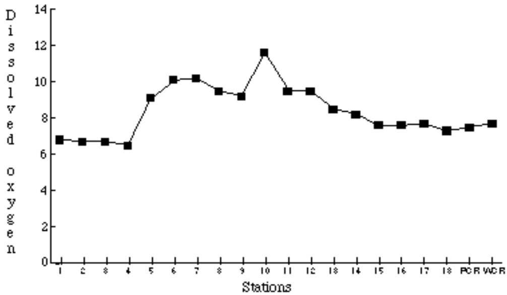
FIG. 2. Temperature (°C) and dissolved oxygen (mg/L) at Peak Creek Stations 1-18, Peak Creek Reference Station (PCR), and Wolf Creek Reference Station (WCR).
