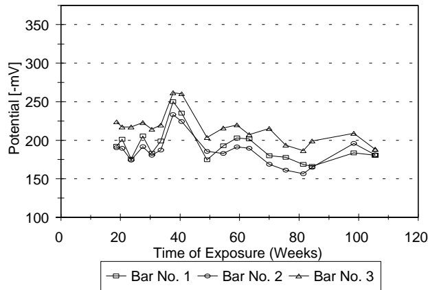
i. SF Specimen - Left Leg (Reinforcing Steel Electrically Connected).
