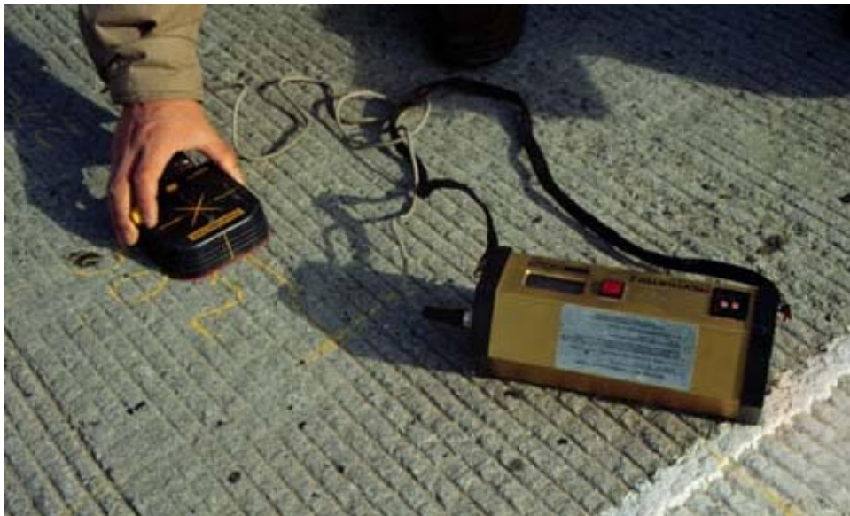
FIGURE 16. Cover Depth Measurement – Profometer III Device.
