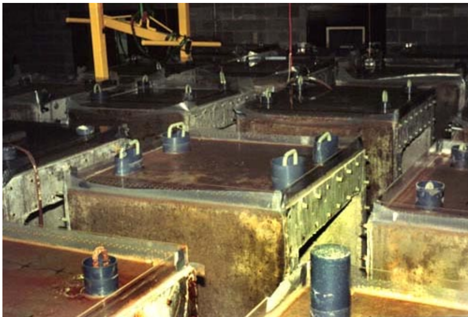
FIGURE 14. Experiment in Progress – Exposure to Wet / Dry Cycles.
