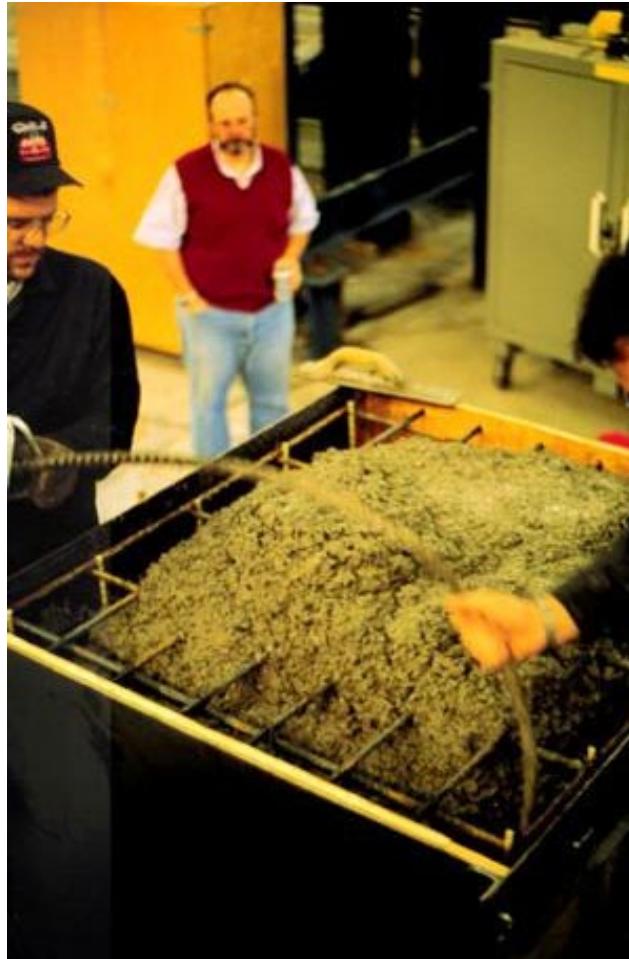
FIGURE 11. Concrete Placement and Vibration – Typical Specimen.
