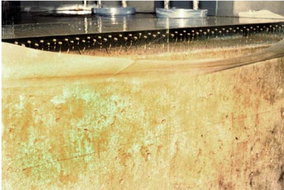
FIGURE 13. Plexiglass Dike: Horizontal / Vertical Exposure Zones.
