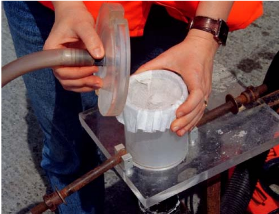
FIGURE 7. Powder Concrete Collection Unit.
