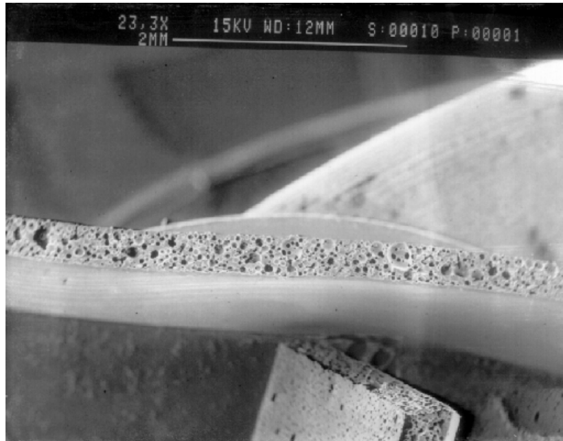
Figure 3-33 SEM of cellular material produced by the mixing technique showing edge view perspective.
