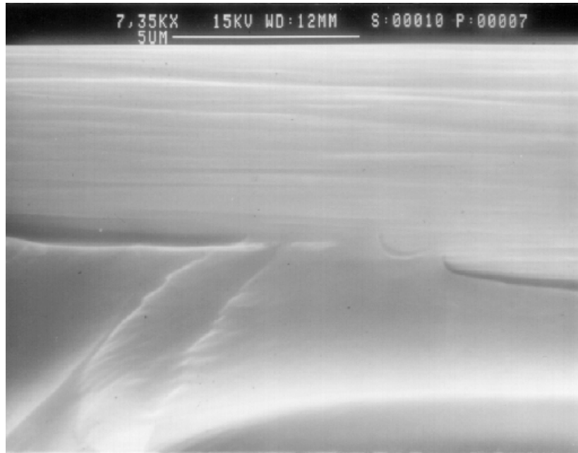
Figure 3-72 SEM of carbon fiber containing cellular materials showing the general poor adhesion between the carbon fiber and acrylated urethane oligomer.
