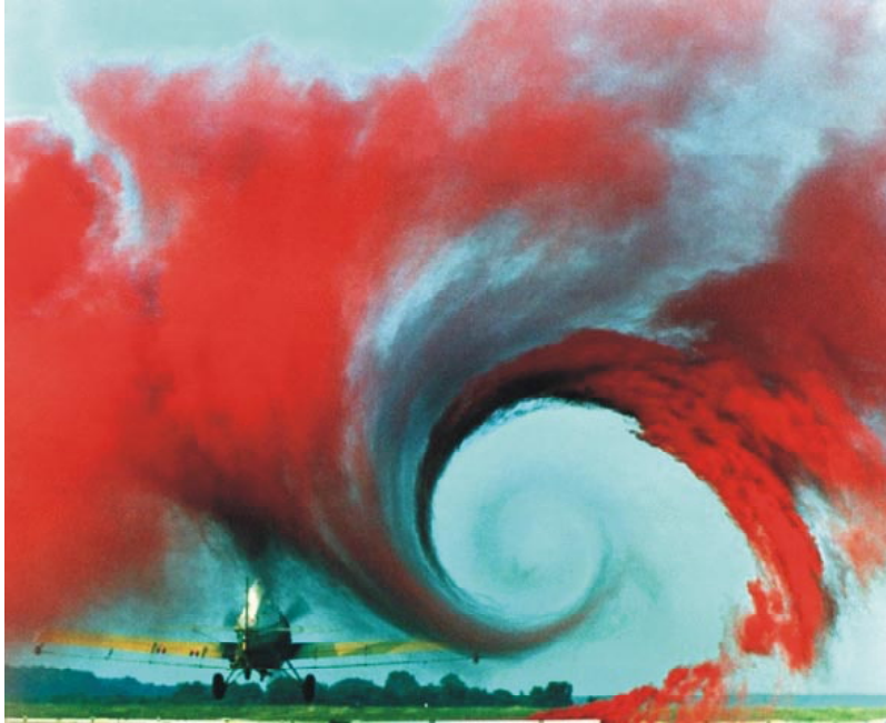
Figure 2-26: A photograph showing the wing-tip-vortex flowfield.
