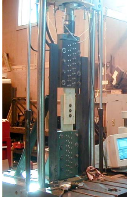
Figure 3.5: Photograph of single shear connection test and fixture.
