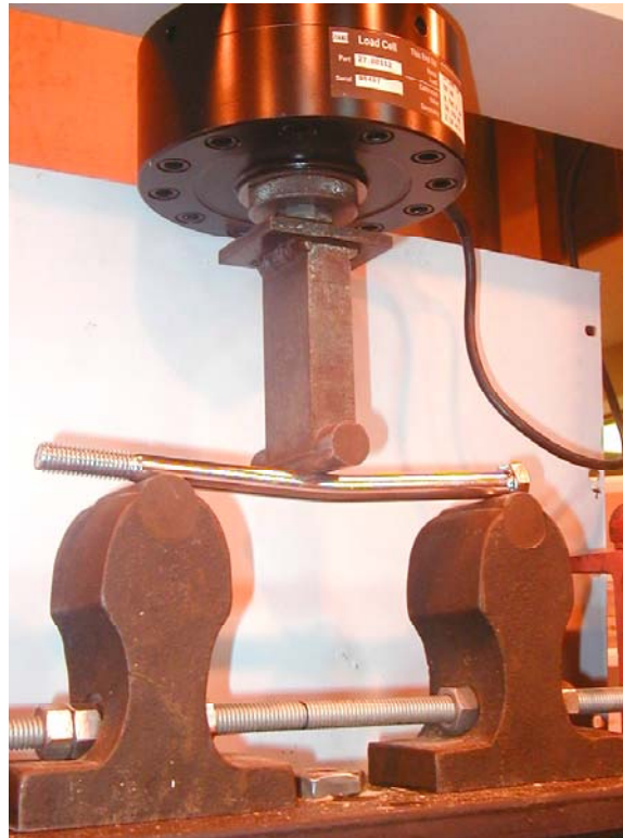
Figure 3.11: Photograph of bolt bending test: three-point loading.
