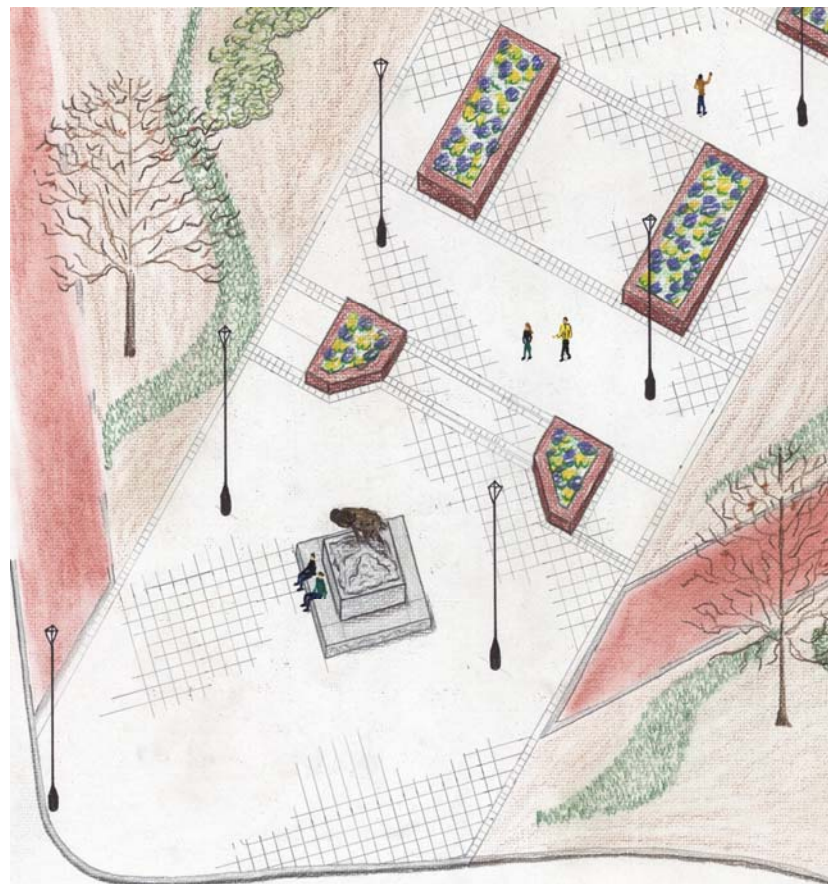
Axonometric drawing of the upper section of the central walk. Raised planters divide the broad expanse of the walk. The central section is ramped, while the outer sections employ stairs allowing for a smooth transition to the terraced lawns.
