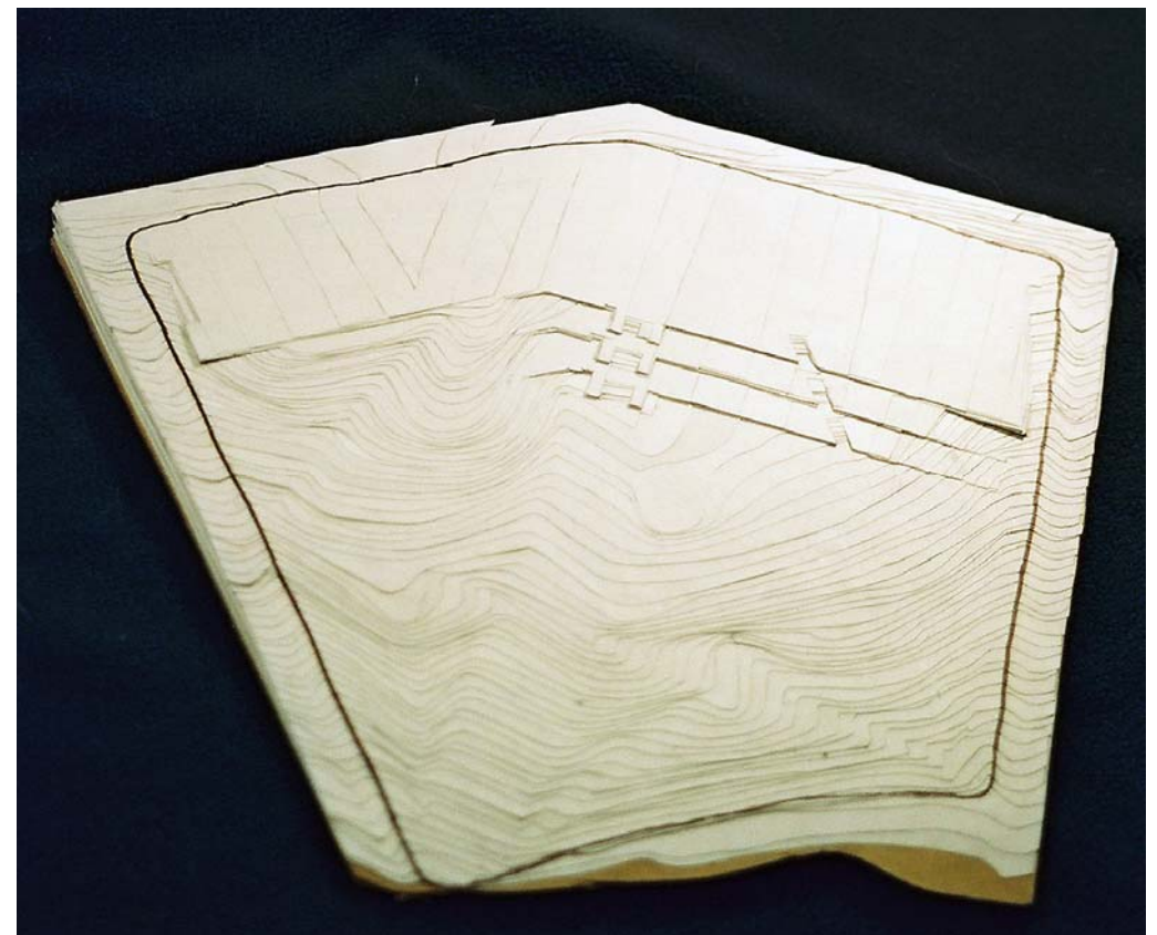
Right, model of proposed grading for Monroe Park. Subtle manipulation of the topography helps emphasize transitions and create stronger connections to surroundings.
