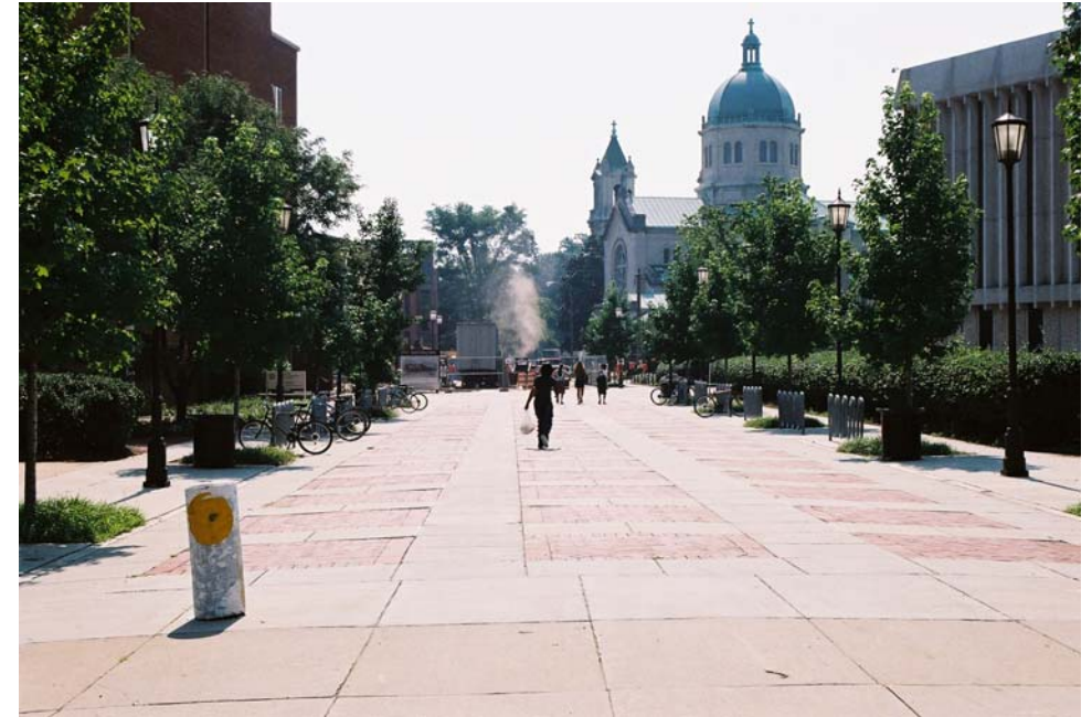
The paving for the plaza draws on the combination of brick and larger concrete pavers found throughout the VCU campus. Unlike the paving at VCU, which combines the materials into a single pattern, the paving for the plaza contrasts the grid of concrete pavers and the pattern of existing paths paved in brick.
