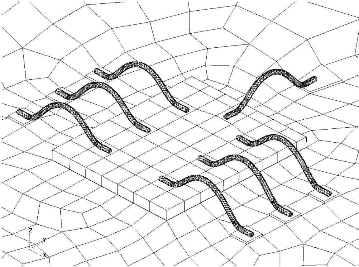
**Figure III-2** Close-up View of Wire Bond Model
