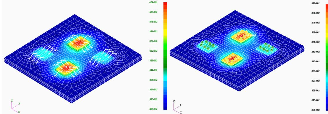
**Figure III-7** Comparison of Temperature Distribution Between the Wire Bond Model and the MPIPPS Model
