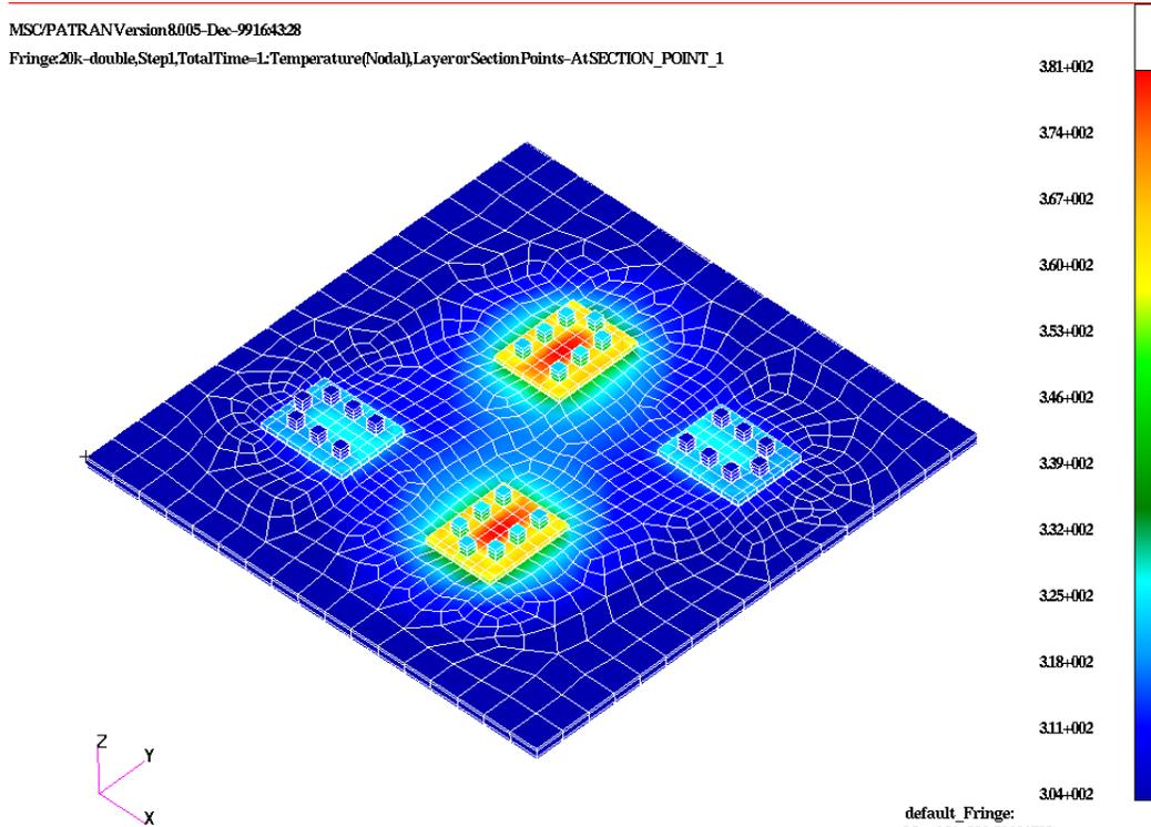
**Figure III-10** Temperature Distribution of Double-sided Cooled MPIPPS Model
