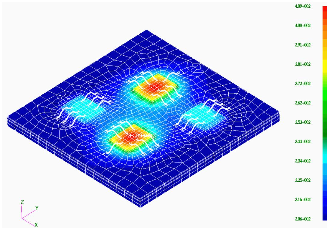
**Figure III-3** Temperature Distribution in Wire Bond Model
