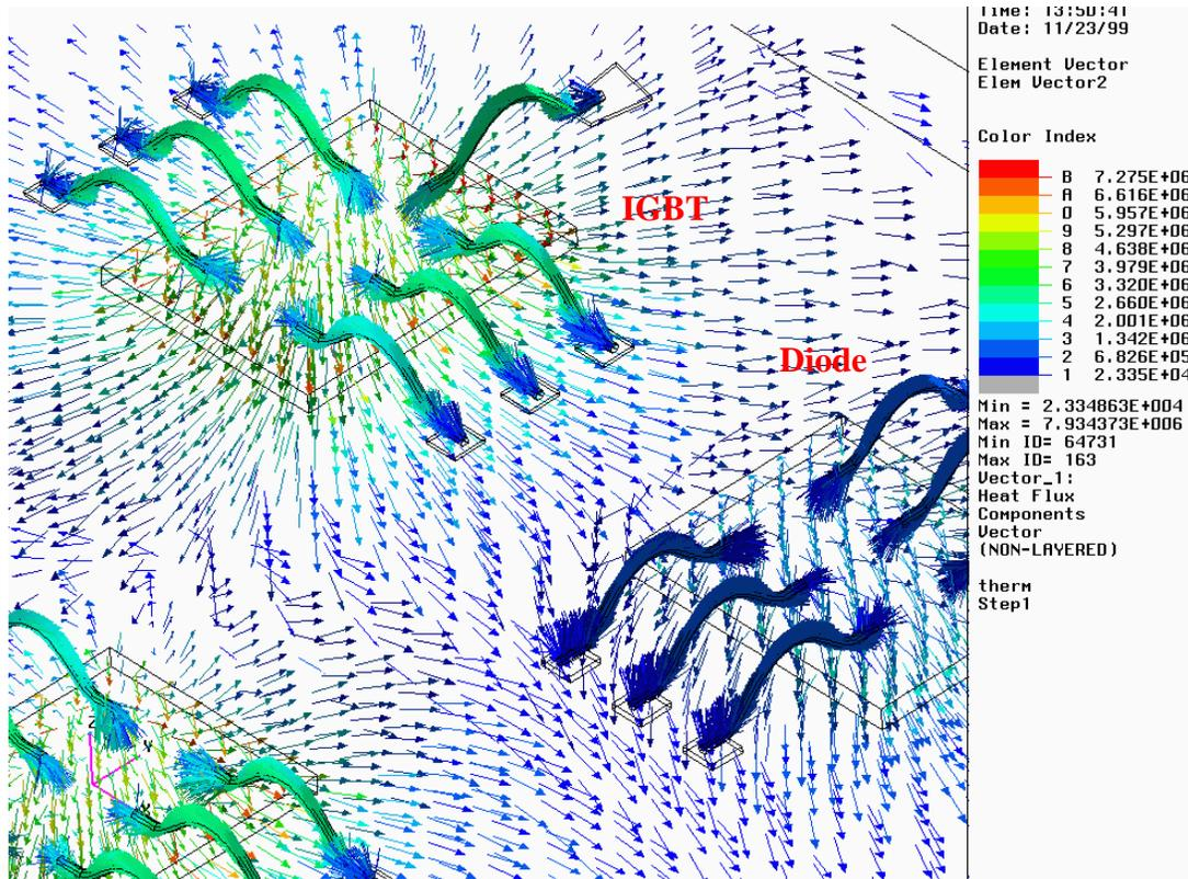
**Figure III-8** Heat Flux Vector Plot in Wire Bond Model
