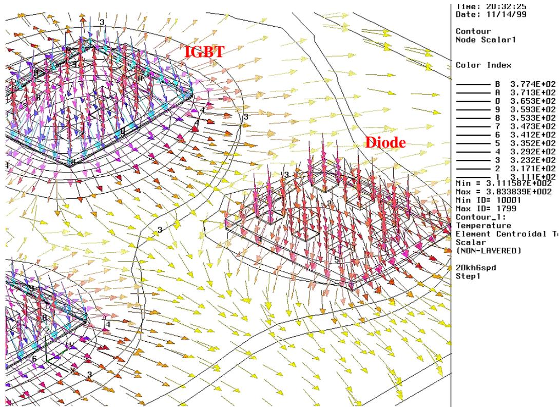
**Figure III-9** Heat Flux Vector Plot in MPIPPS Model
