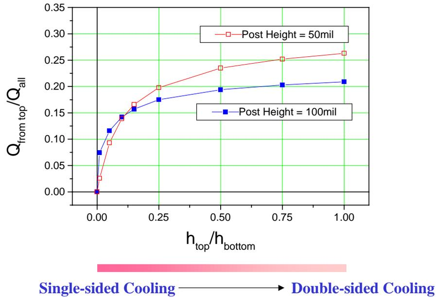
**Figure III-11** Double-sided Cooling and Post Height Effects
