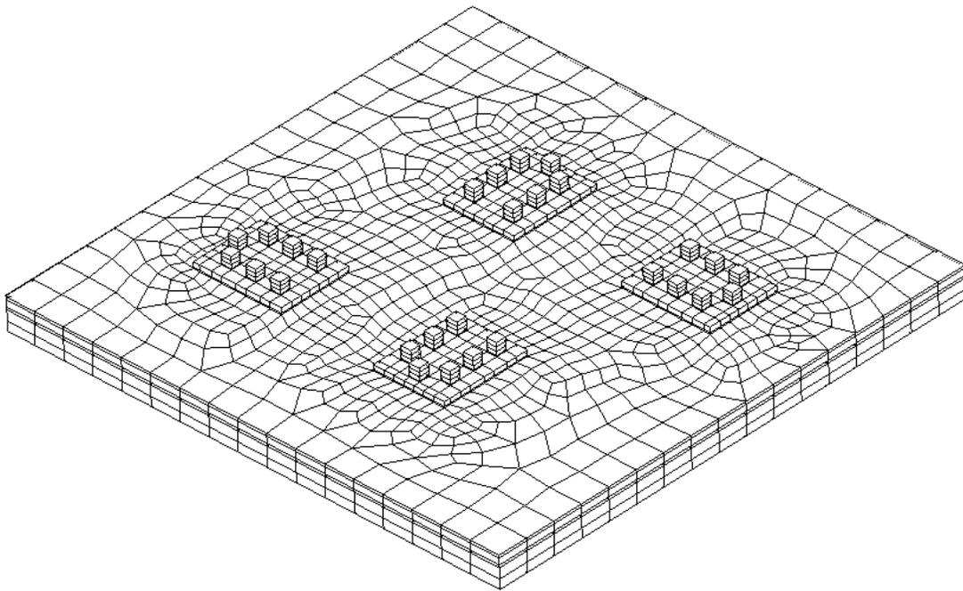
**Figure III-4** FEM Model of MPIPSS Module
