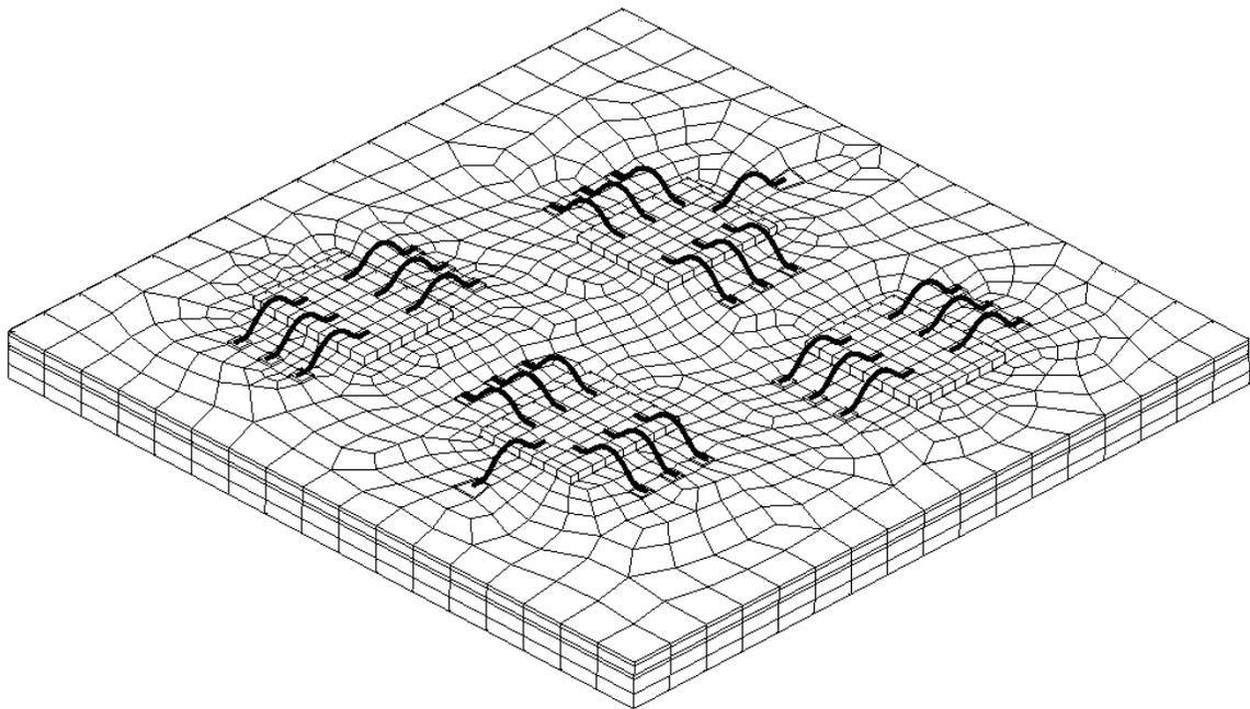
**Figure III-1** FEM Model of the Wire Bond Module
