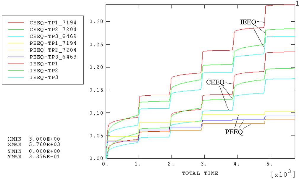
**Figure IV-30** CEEQ, PEEQ and IEEQ Histories for Element 7194,7204 and 6469 under Temperature Cycling Condition
