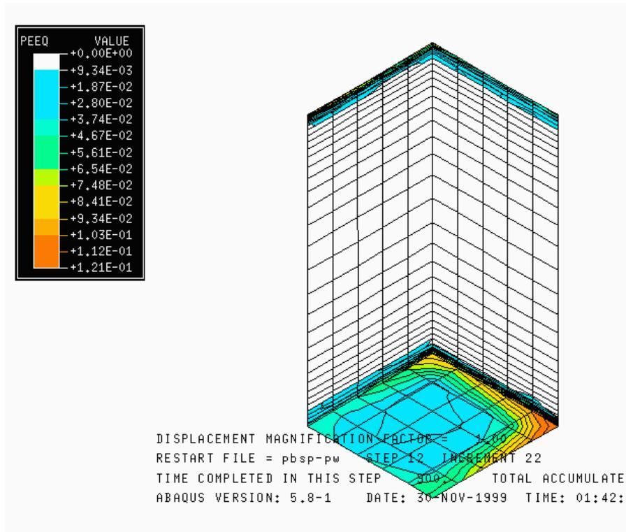
**Figure IV-26** PEEQ Contour under Power Cycling
