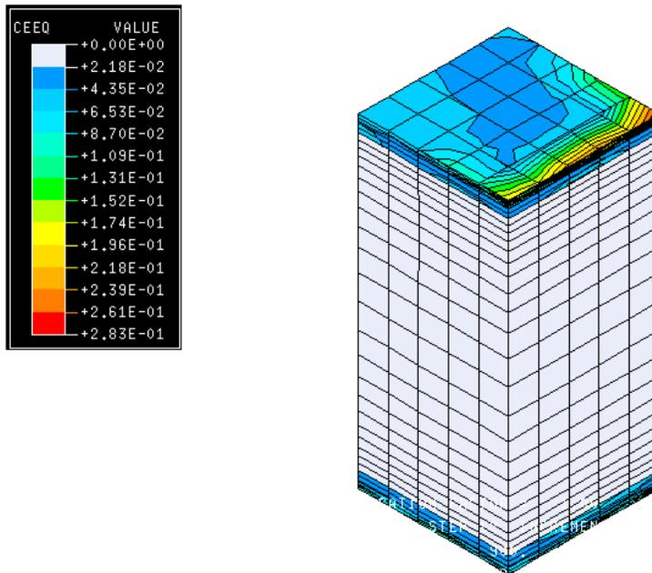
**Figure IV-18** CEEQ Contour under Temperature Cycling
