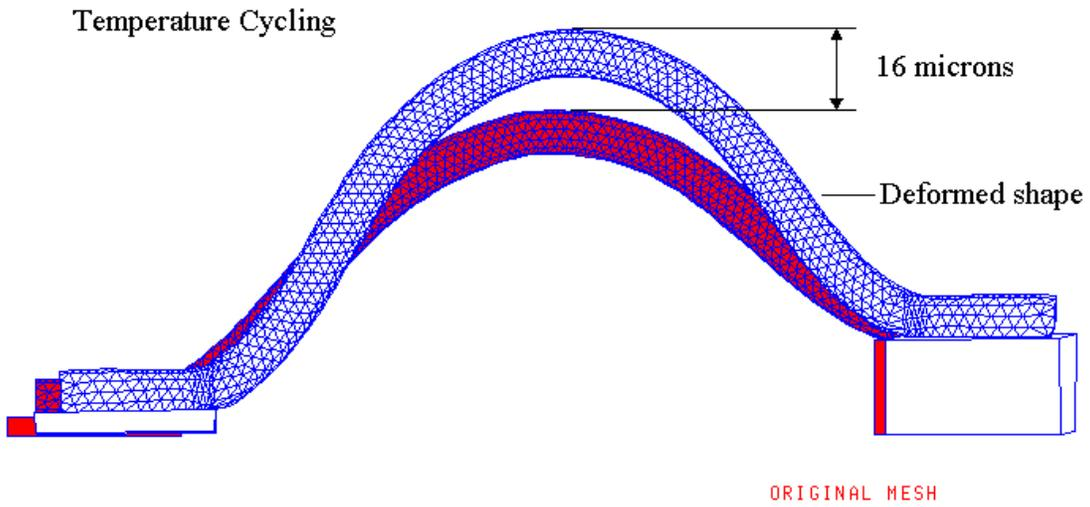
**Figure IV-11** Deformation Plot of the Wire Bond under Temperature Cycling,
