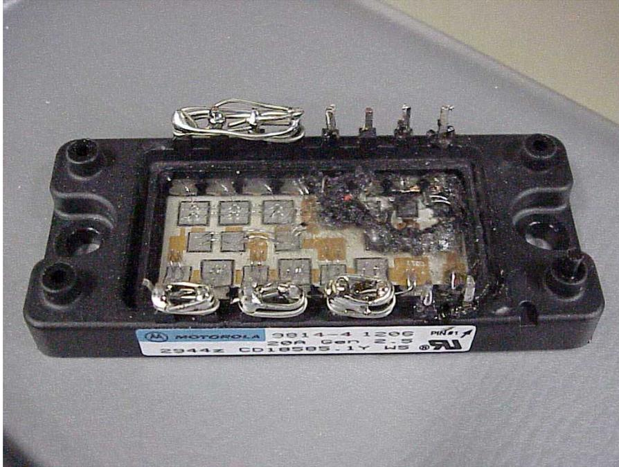
**Figure IV-32** A Burnt-out Wire Bond Module Shows the Wire Debonding
