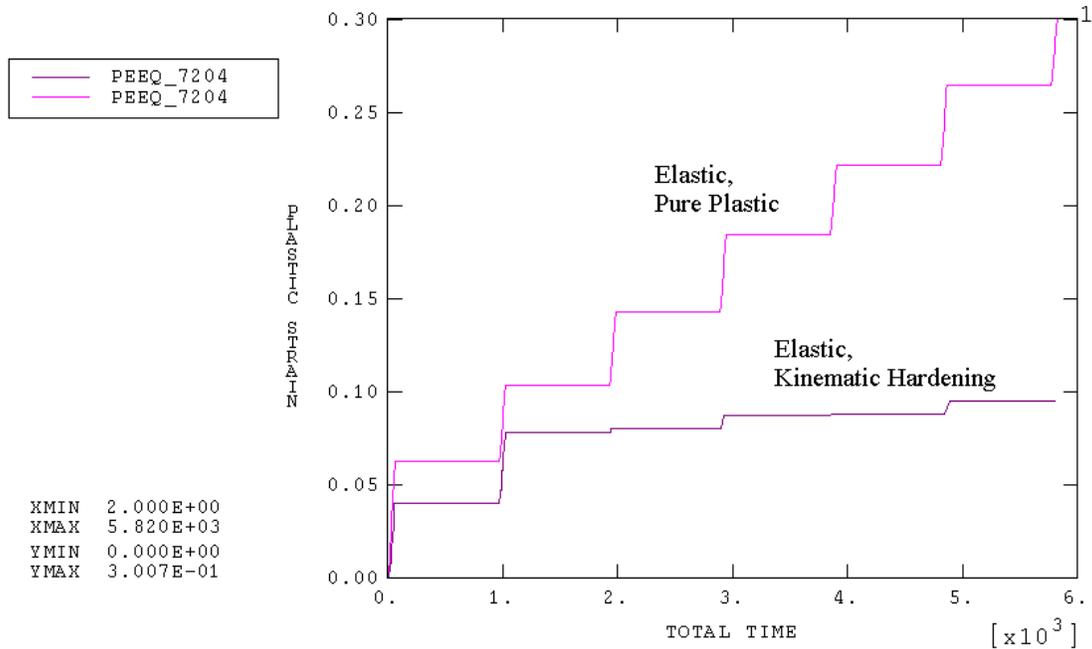
**Figure IV-15** Comparison Between Pure Plasticity and Kinematic Hardening Plasticity for Modeling Eutectic Solder Material
