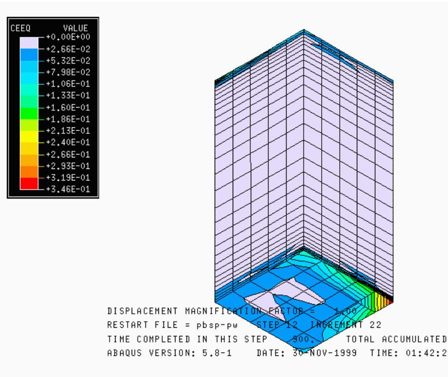
**Figure IV-25** CEEQ Contour under Power Cycling
