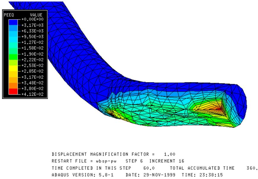
**Figure IV-5** PEEQ Contour for Device-side Wire Bond, Power Cycling,
