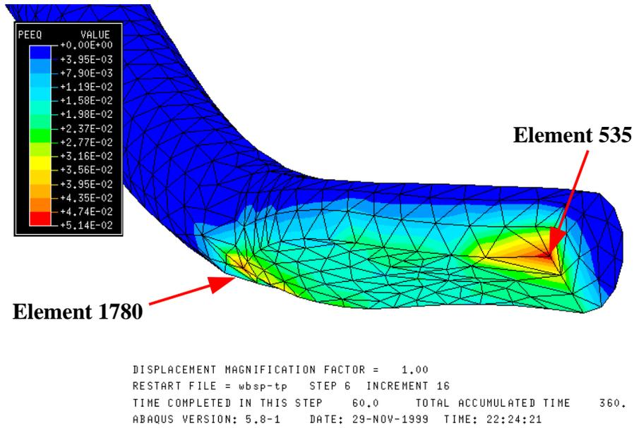
**Figure IV-4** PEEQ Contour for Device-side Wire Bond, Temperature Cycling,
