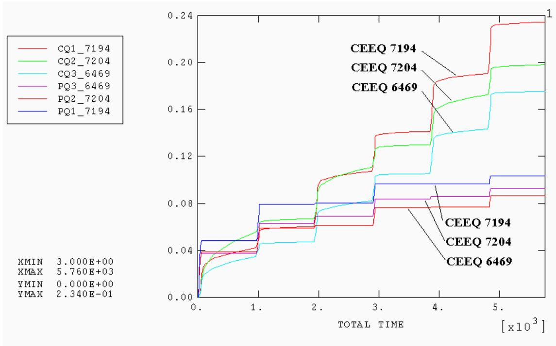
**Figure IV-16** Average CEEQ and PEEQ in Element 7194, 7204 and 6469 under Temperature Cycling
