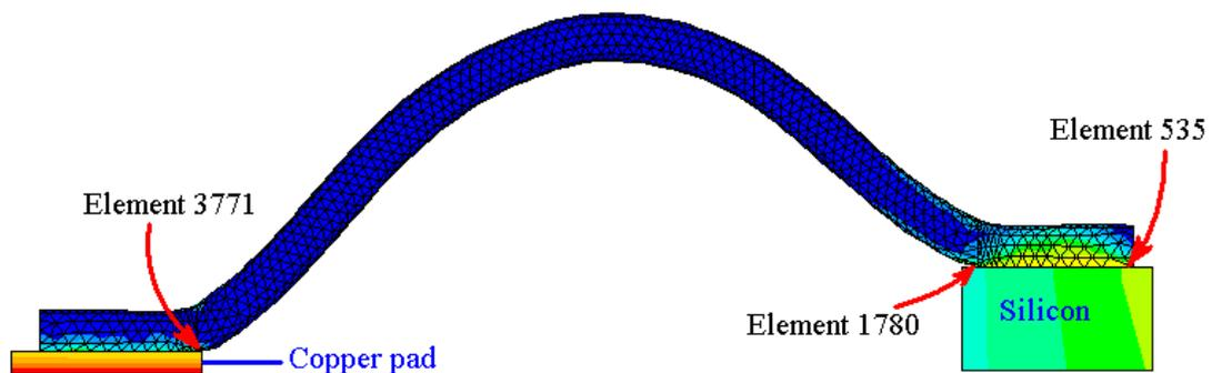
Figure IV-1 Critical Locations in the Wire Bond Model
