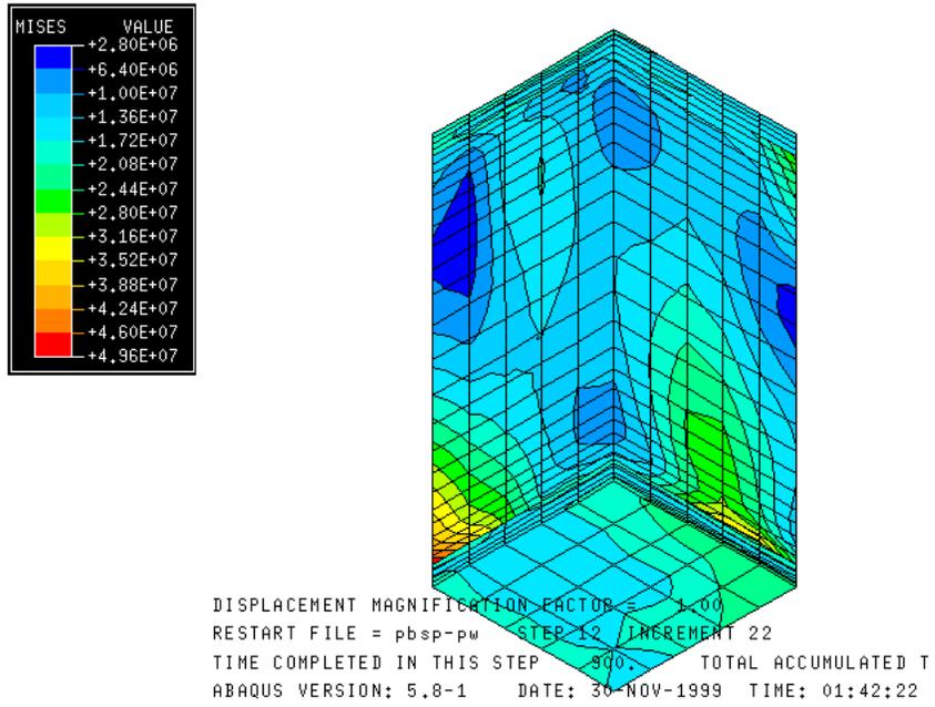
**Figure IV-24** Von Mises Stress Contour under Power Cycling
