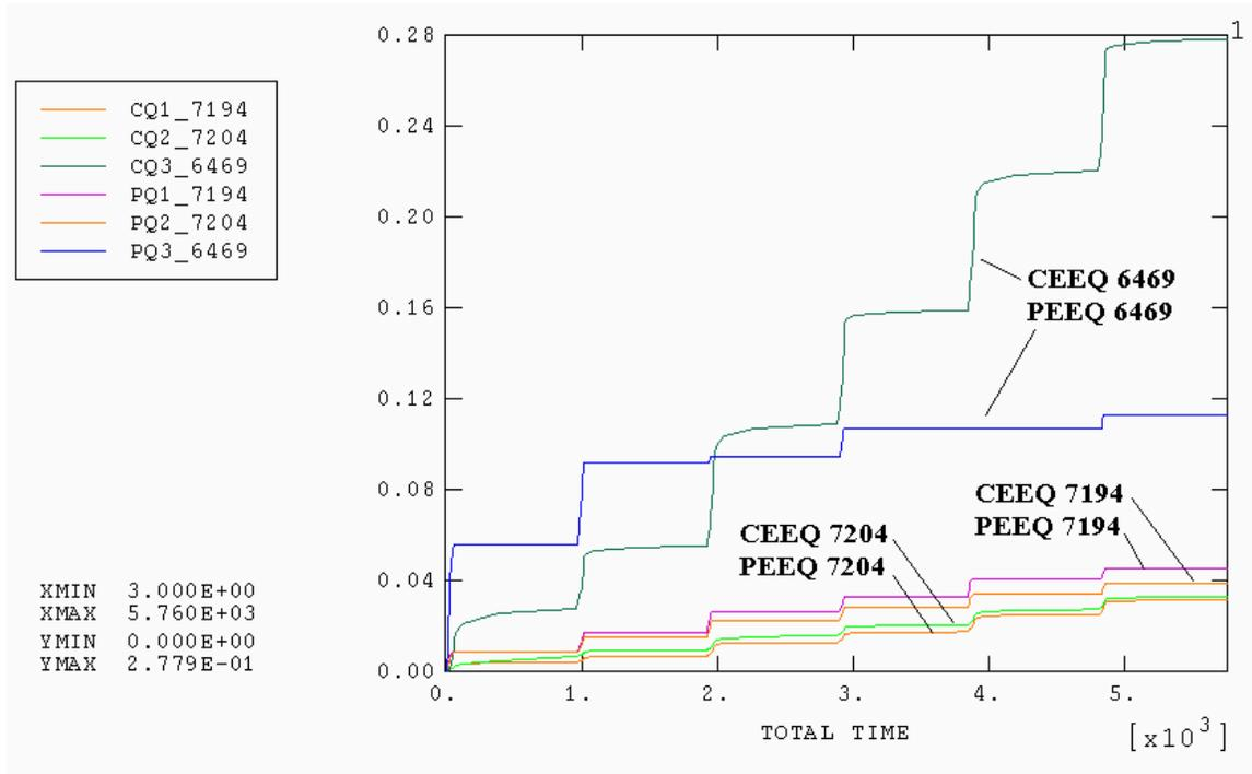
**Figure IV-23** Average CEEQ and PEEQ in Element 7194, 7204 and 6469 under Power Cycling
