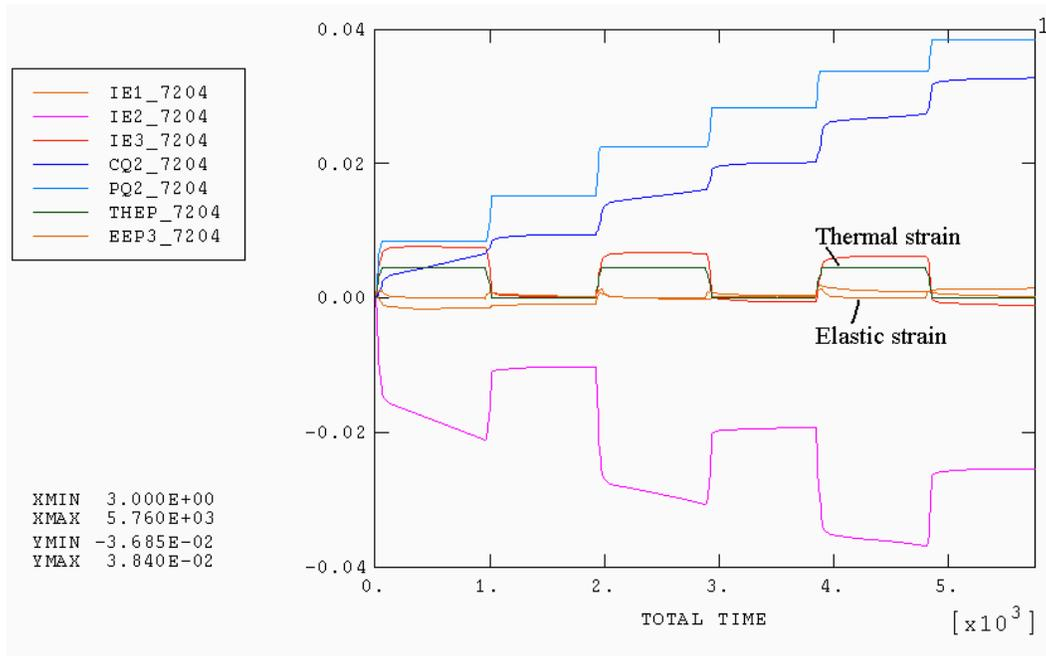
**Figure IV-14** Total Strain Components for Element 7204 under Temperature Cycling
