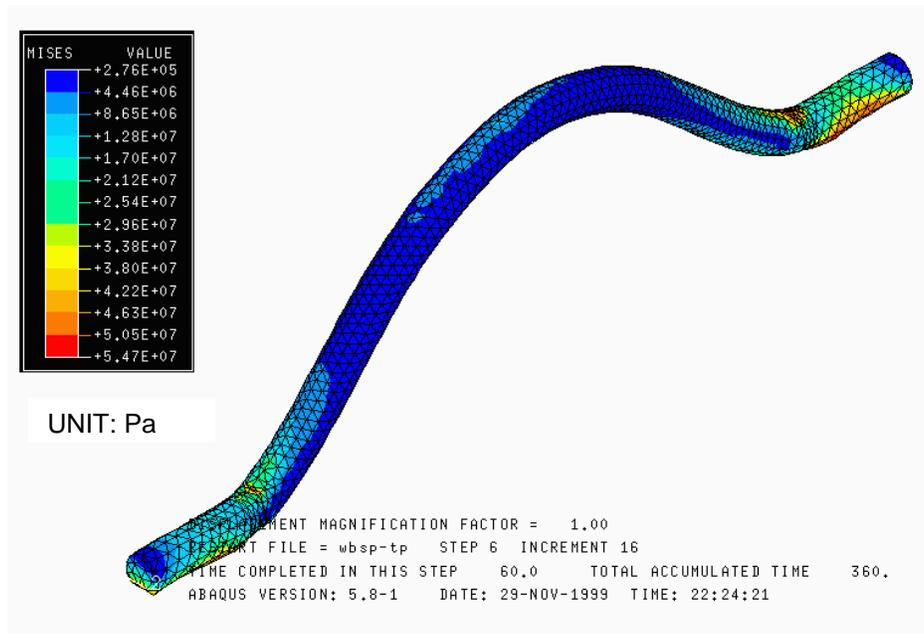
**Figure IV-2** Von Mises Contour of the Wire Bond under Temperature Cycling, at the End of the 3<sup>rd</sup> Cooling Stage
