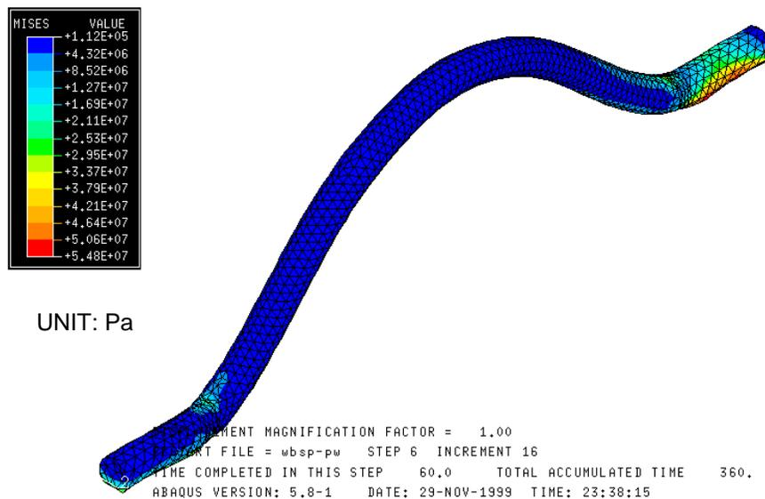
**Figure IV-3** Von Mises Contour of the Wire Bond under Power Cycling, at the end of the 3<sup>rd</sup> Cooling Stage
