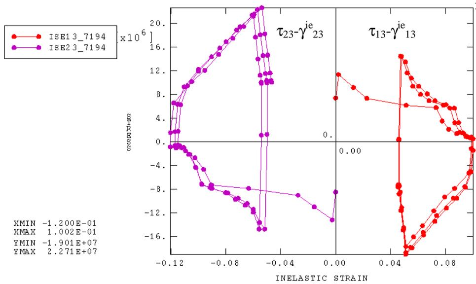
**Figure IV-22** Hysteresis Loops of Shear Stress-Inelastic Shear Strain of Element 7194
