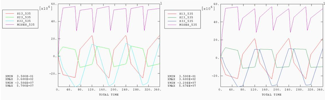
**Figure IV-8** Stress Histories for Element 535 at Temperature Cycling (left) and Power Cycling (right)
