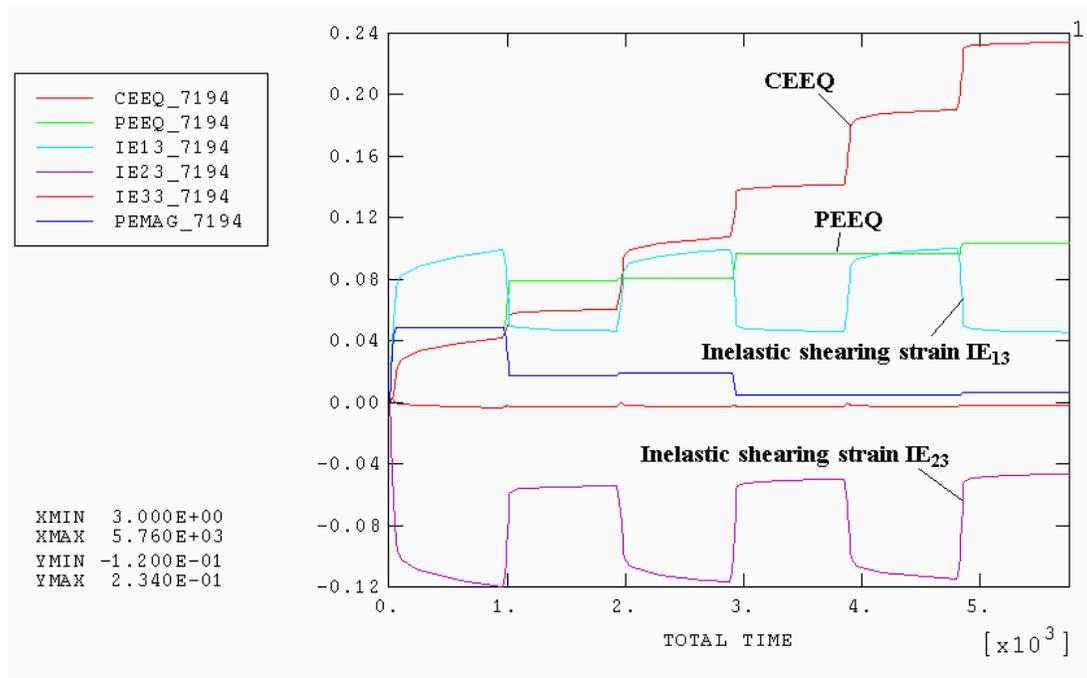
**Figure IV-21** Inelastic Strain History for Element 7194 under Temperature Cycling
