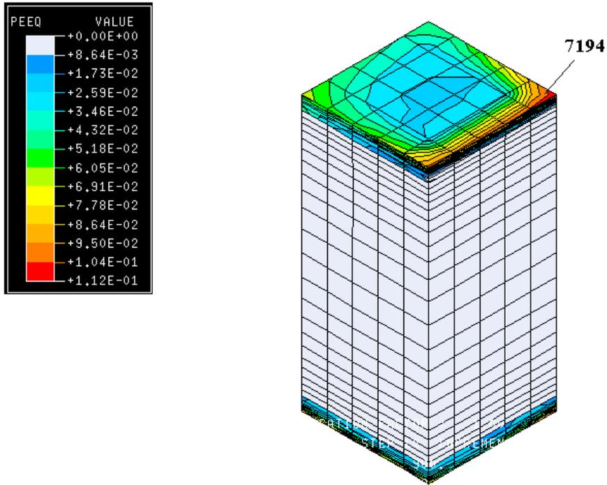
**Figure IV-19** PEEQ Contour under Temperature Cycling
