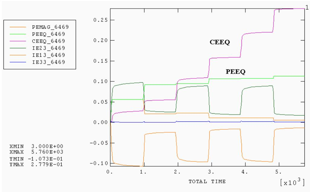
**Figure IV-28** Inelastic Strain history for Element 6469 under Power Cycling
