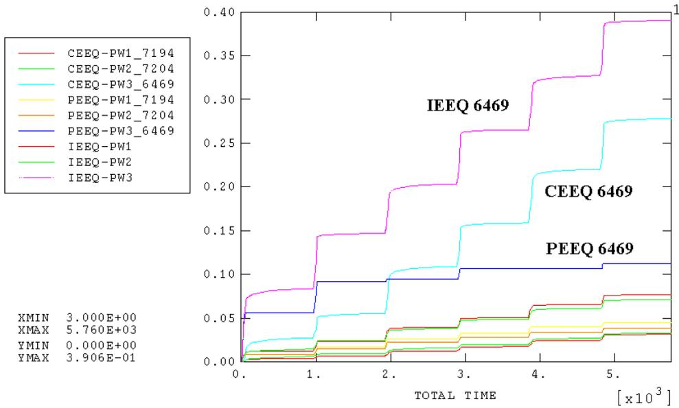
**Figure IV-31** CEEQ, PEEQ and IEEQ Histories for Element 7194,7204 and 6469 under Power Cycling Condition
