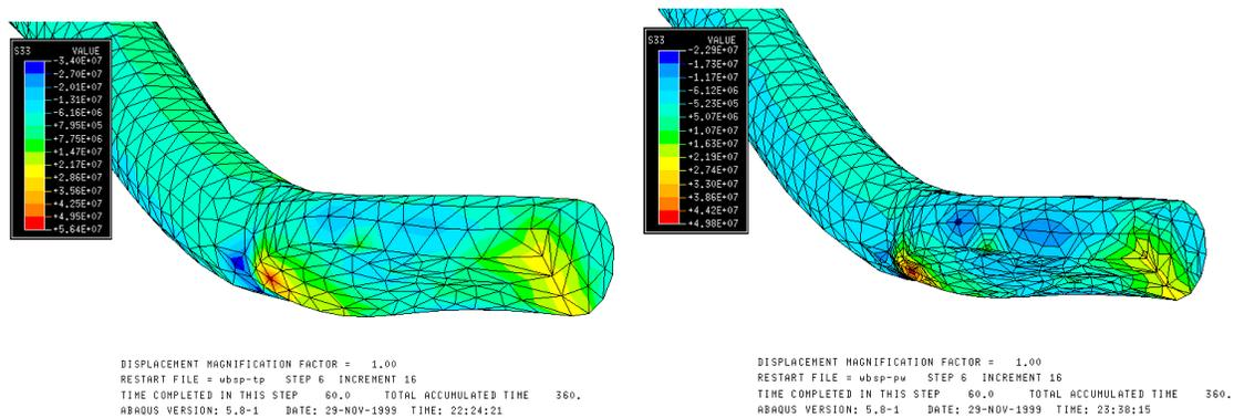
**Figure IV-10** Normal Stress  $\sigma_3$  Contour in Device-side Wire Bond Under Temperature Cycling (left) and Power Cycling (right)
