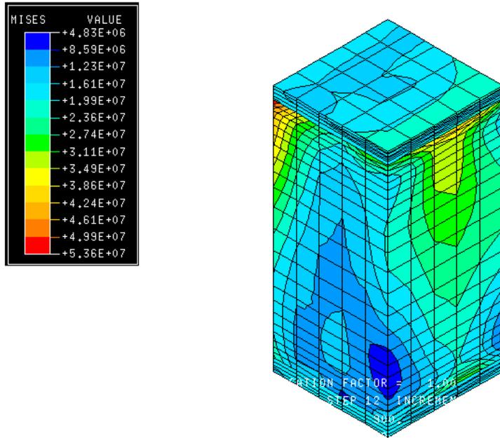
**Figure IV-17** Von Mises Stress Contour under Temperature Cycling
