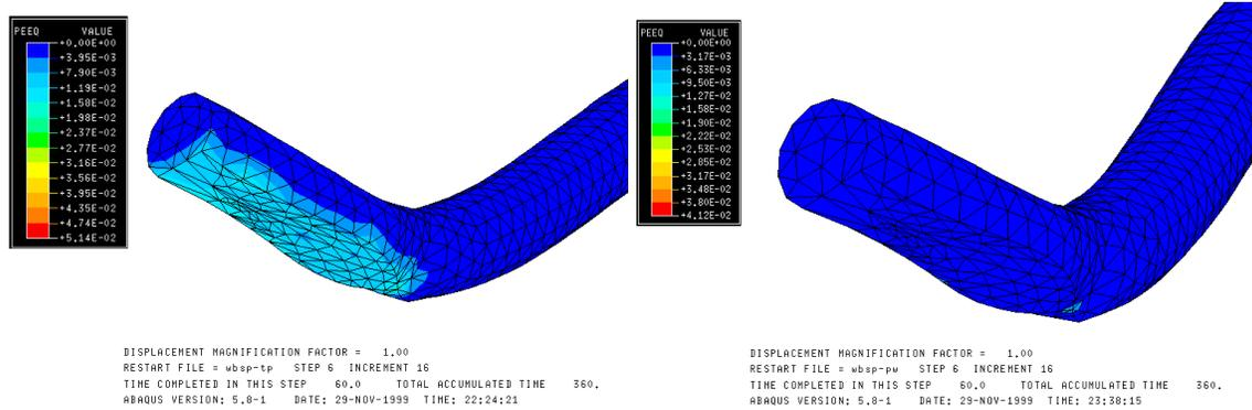
**Figure IV-6** PEEQ Contour for Pad-side Wire Bond, Temperature Cycling (left), Power Cycling (right), At the End of the 3<sup>rd</sup> Cooling Stage
