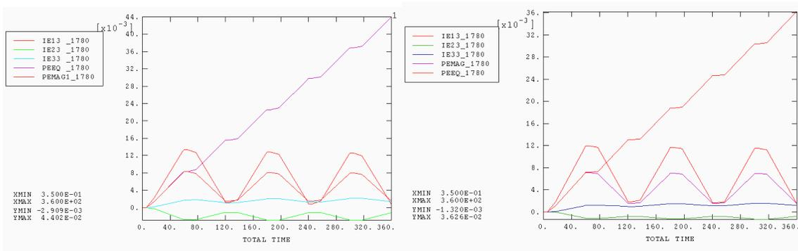
**Figure IV-9** Inelastic Strain Histories for Element 1780 at Temperature Cycling (left) and Power Cycling (right)
