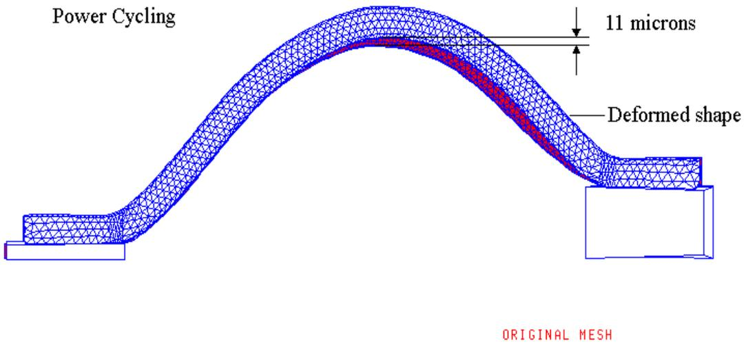
**Figure IV-12** Deformation Plot of Wire Bond under Power Cycling,
