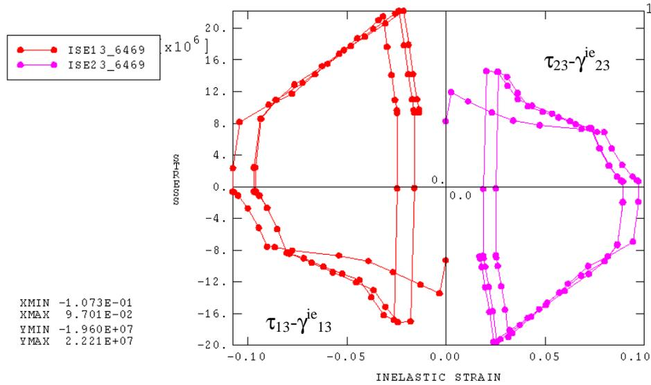
**Figure IV-29** Hysteresis Loops of Shear Stress-Inelastic Shear Strain of Element 6460
