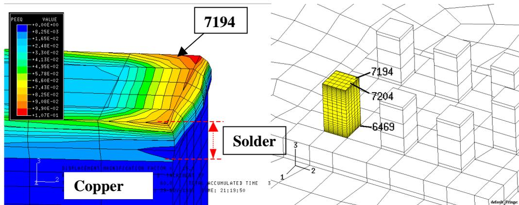
**Figure IV-13** Determination of Critical Locations in MPIPPS Model
