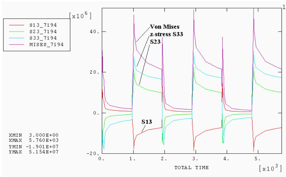
**Figure IV-20** Stress History for Element 7194 under Temperature Cycling
