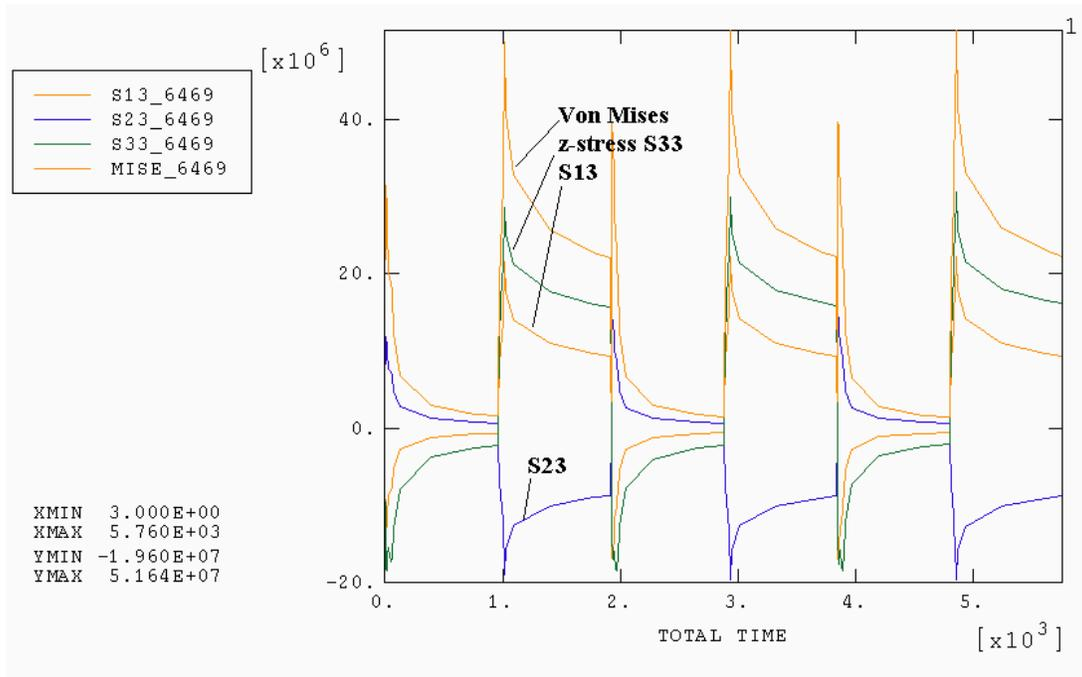
**Figure IV-27** Stress History for Element 6469 under Power Cycling
