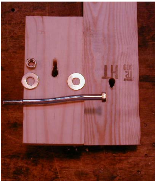
Figure 4.18: Typical post-test condition of bolted connections yielding by Mode IV.
