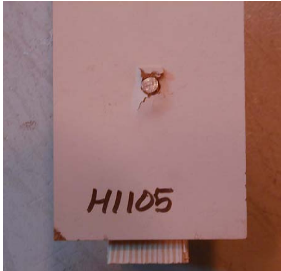
Figure 4.9: Crushed material at bearing interface in hardboard connection.
