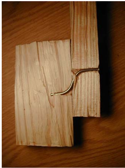
Figure 4.13: Mode IV yield observed in solid wood nailed connections.
