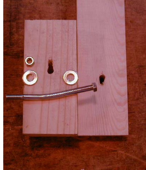
Figure 4.17: Typical post-test condition of bolted connections yielding by Mode III.
