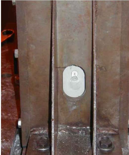
Figure 4.1: Gypsum wallboard connection test in progress; nail head exhibiting the onset of mode shift.
