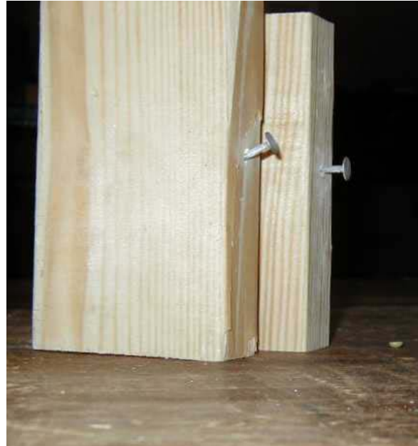
Figure 4.2: Typical post-test fastener condition in connections that exhibited mode shift (left), and those that did not (right).
