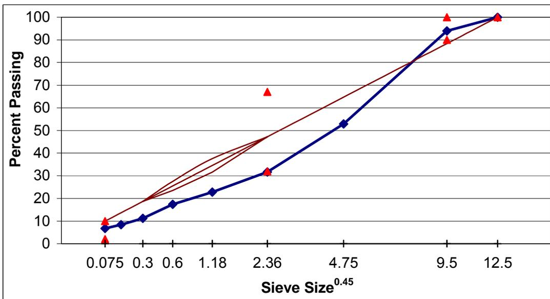
Figure A. 40 Mixture designs for SM-12.5A, section L.
