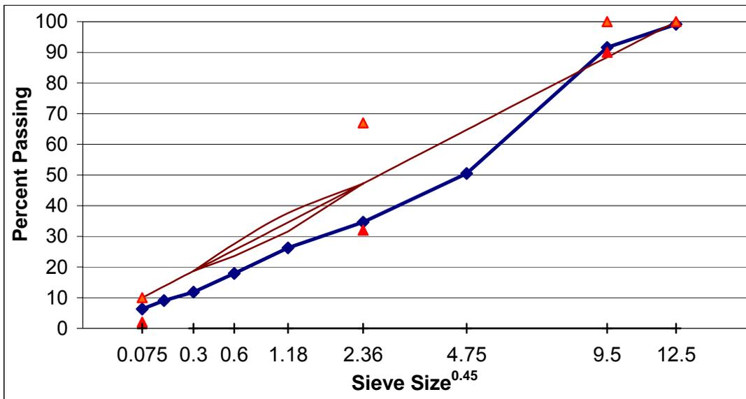
Figure A. 39 Gradation of SM-9.5D, lab-lab mixture, section J.
