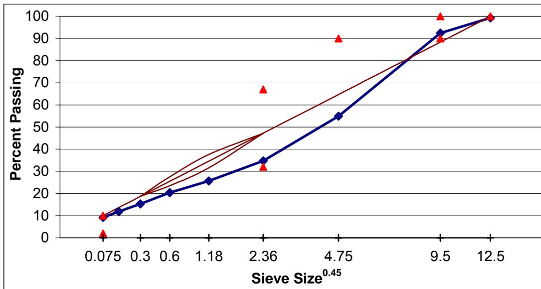
Figure A. 18 Gradation of SM-9.5A, field-lab mixture, section D.
