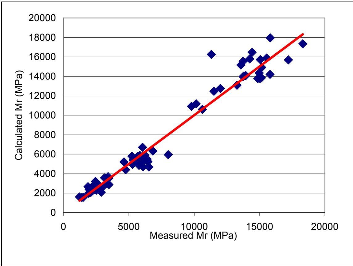
Figure 4-6 Calculated vs. Measured  $M_r$
