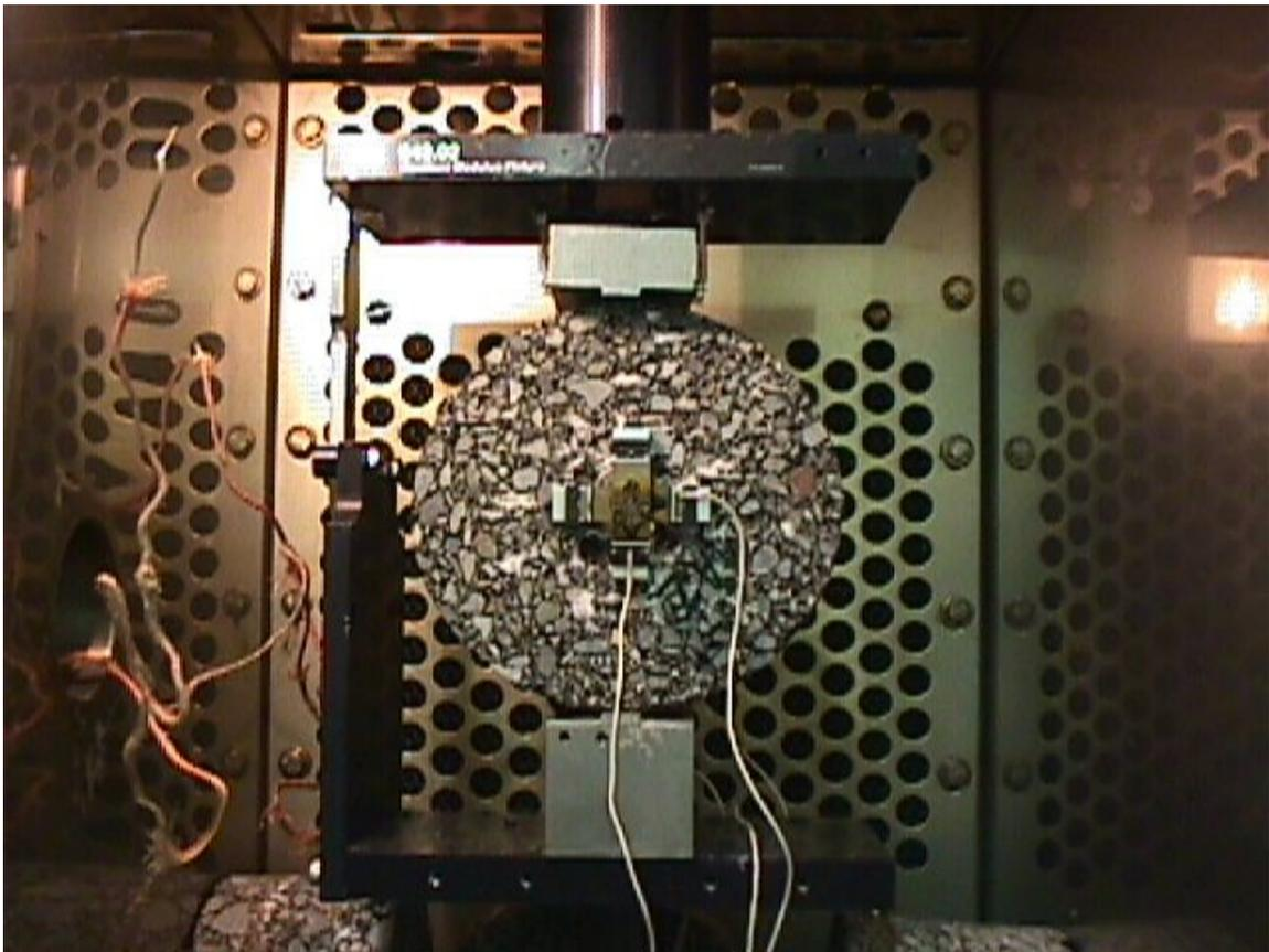
Figure 3-4 Test configuration of the Indirect Tension Test
