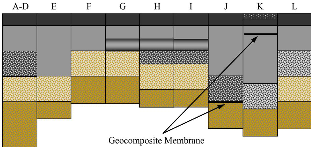
Figure 3-1 Structural configuration of Virginia Smart Road.
