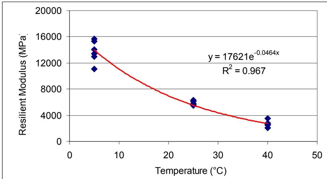
Figure 4-5 Resilient Modulus Variation with Temperature (Specimen A1-4in D/L)
