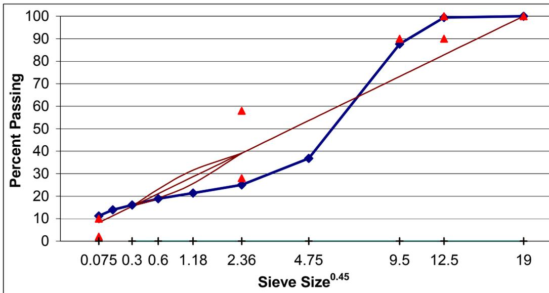
Figure A. 43 Gradation of SM-12.5A, lab-lab mixture, section L.
