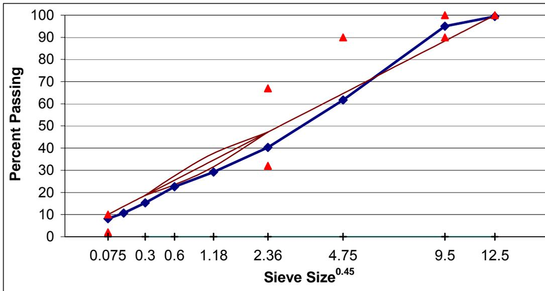
Figure A. 13 Gradation of SM-9.5E, field-lab mixture, section C.
