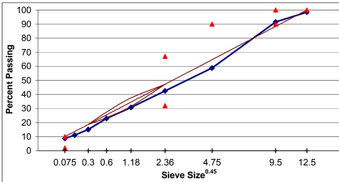
Figure A. 10 Gradation of SM-9.5D, design-lab mixture, section B.
