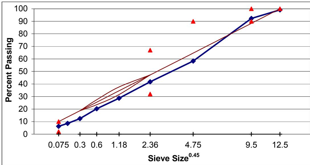
Figure A. 21 Mixture designs for SM9.5D, sections E, F, G, and H.
