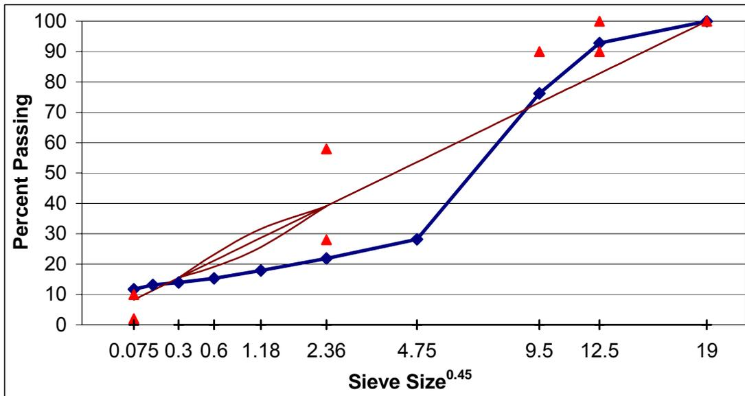
Figure A. 44 Gradation of SM-12.5A, design-lab mixture, section L.
