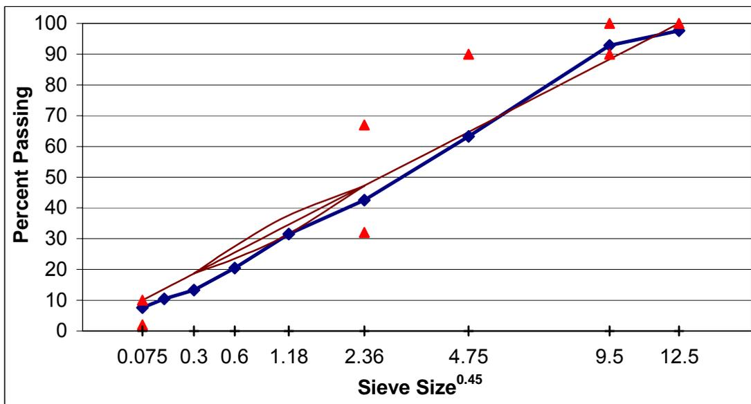
Figure A. 26 Gradation of SM-9.5D, field-lab mixture, section F.
