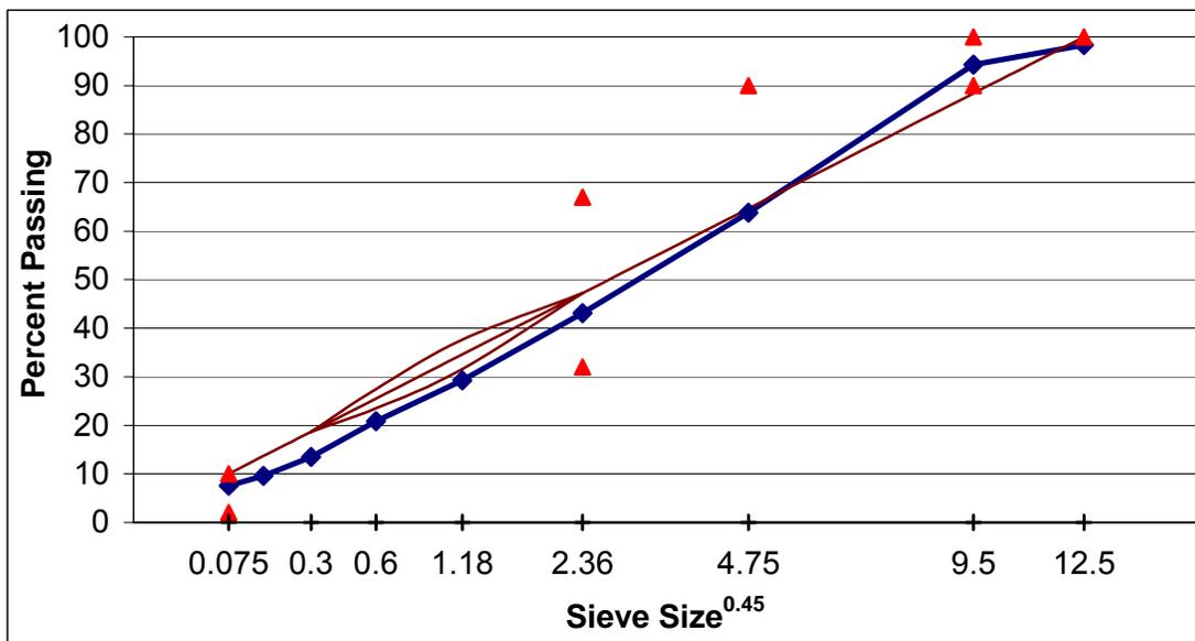
Figure A. 30 Gradation of SM-9.5D, field-lab mixture, section H.
