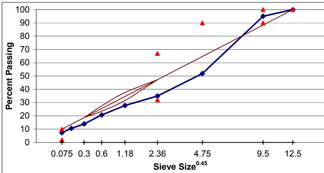
Figure A. 34 Gradation of SM-9.5A, lab-lab mixture, section I.
