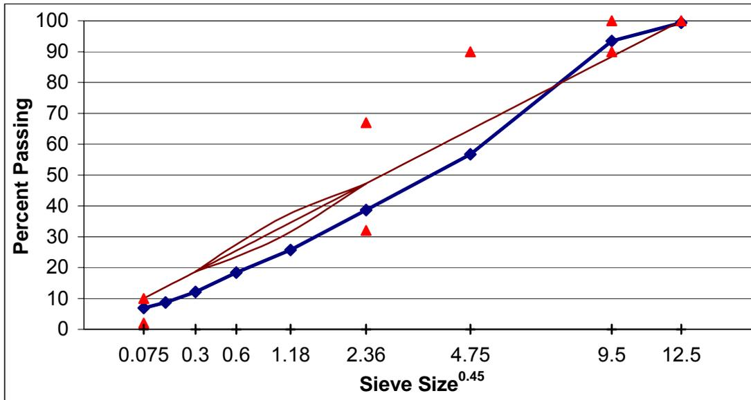
Figure A. 27 Gradation of SM-9.5D, field-field mixture, section G.
