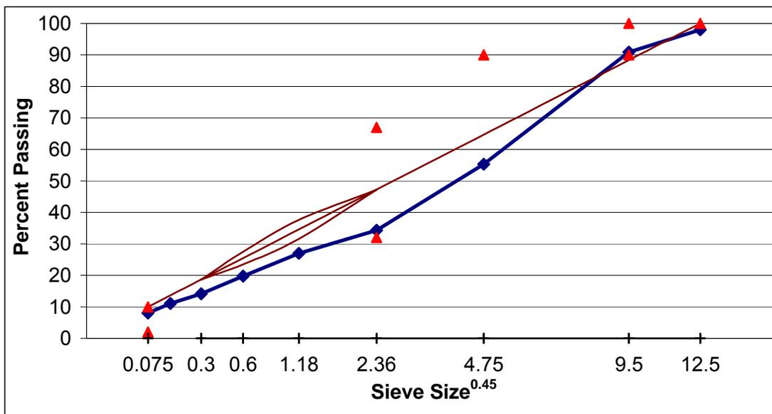
Figure A. 14 Gradation of SM-9.5E, lab-lab mixture, section C.
