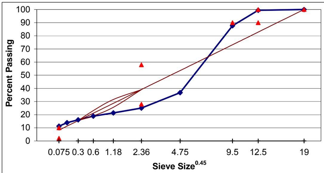
Figure A. 42 Gradation of SM-12.5A, field-lab mixture, section L.
