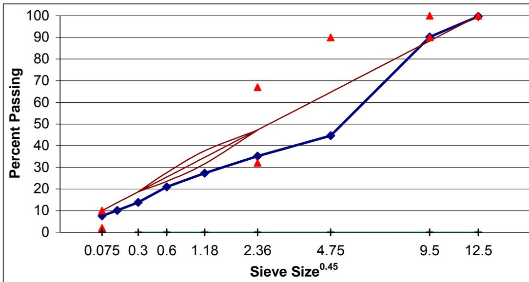
Figure A. 15 Gradation of SM-9.5E, design-lab mixture, section C.
