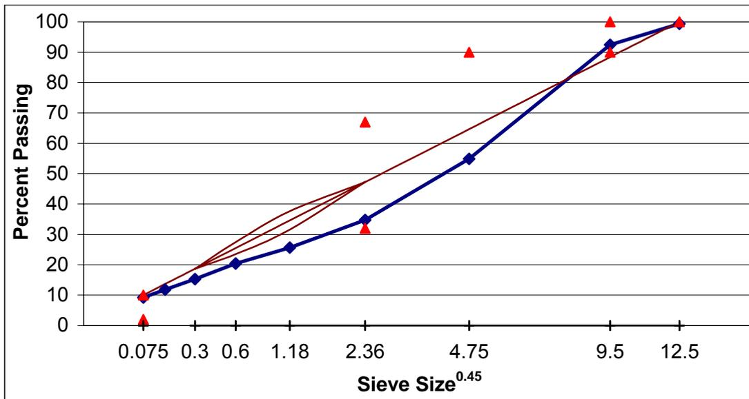
Figure A.19 Gradation of SM-9.5A, lab-lab mixture, section D.
