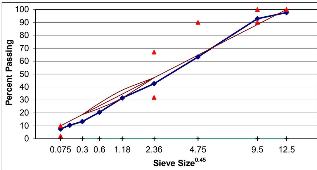
Figure A. 24 Gradation of SM-9.5D, lab-lab mixture, section E.
