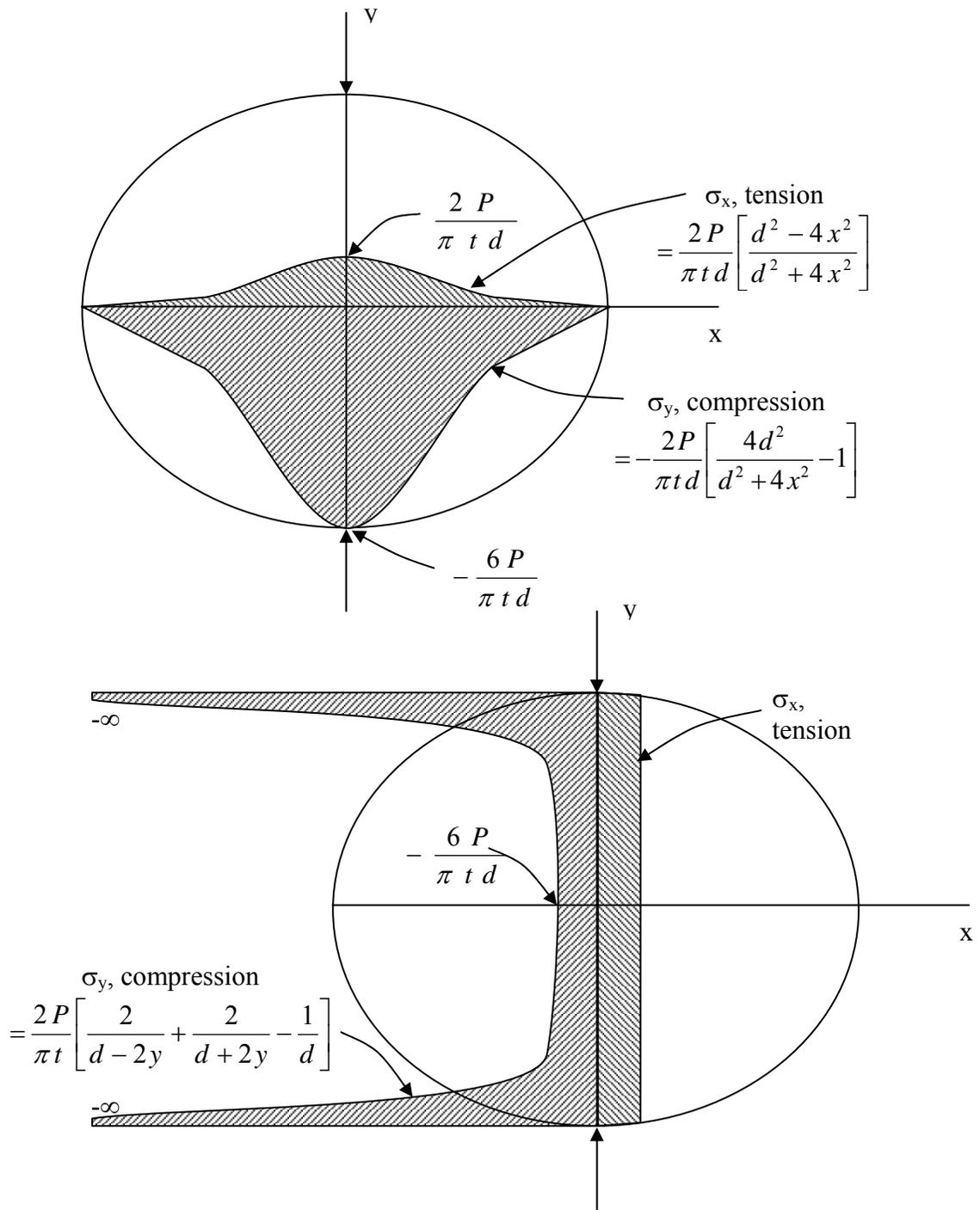
Figure 2-1 Elastic stress distribution in indirect tension specimen.
