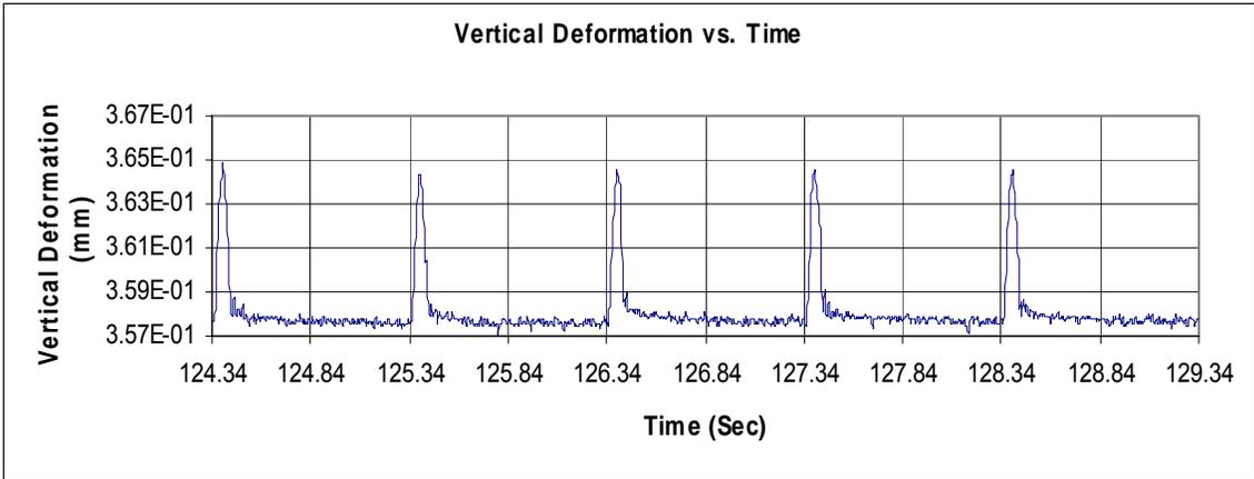
(b) Measured Vertical Deformation
