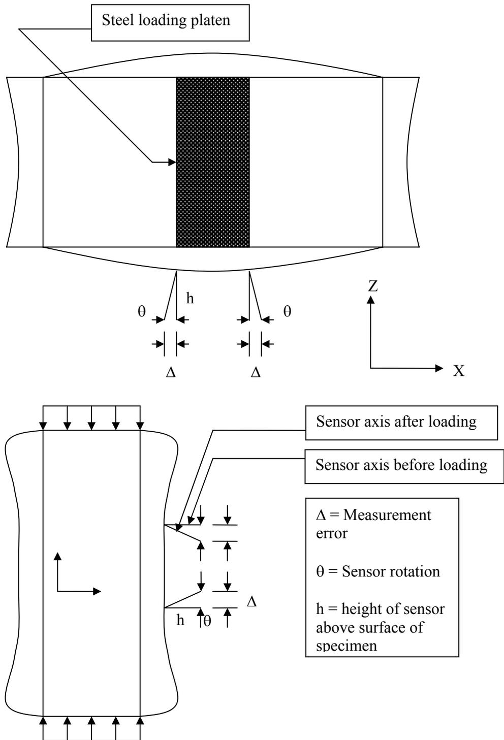
Figure 2-2 Illustration of Bulging Effects
