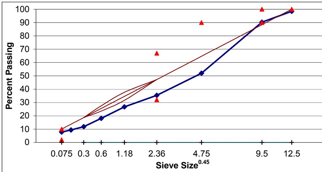
Figure A. 8 Gradation of SM-9.5D, field-lab mixture, section B.
