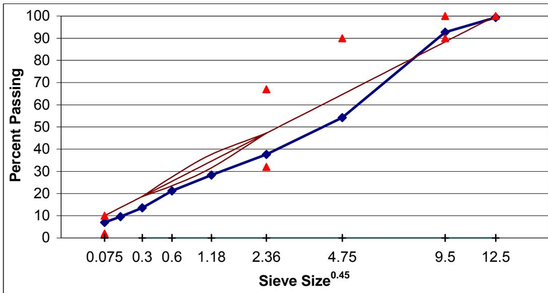
Figure A. 35 Gradation of SM-9.5A, design-lab mixture, section I.
