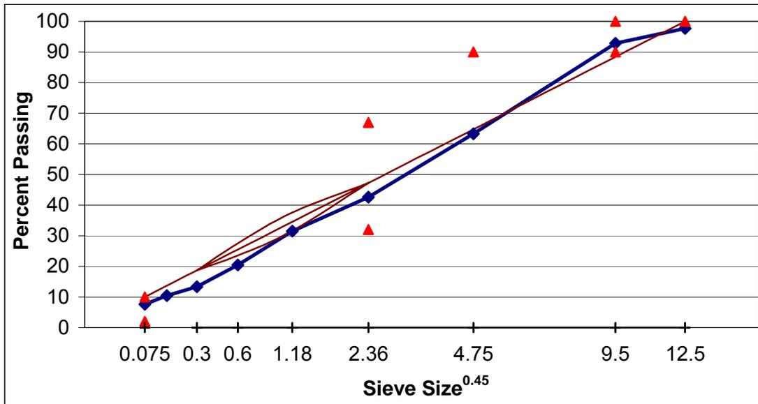
Figure A. 23 Gradation of SM-9.5D, field-lab mixture, section E.
