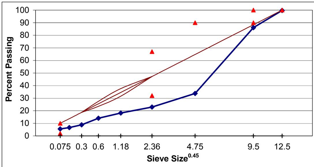
Figure A. 11 Mixture designs for SM9.5E, section C.
