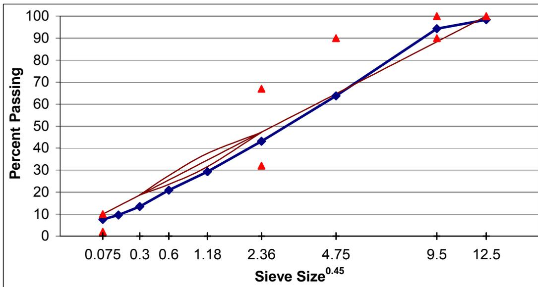
Figure A. 31 Mixture design for SM-9.5A, section I.
