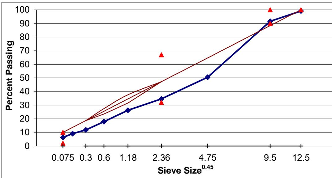
Figure A. 38 Gradation of SM-9.5D, field-lab mixture, section J.
