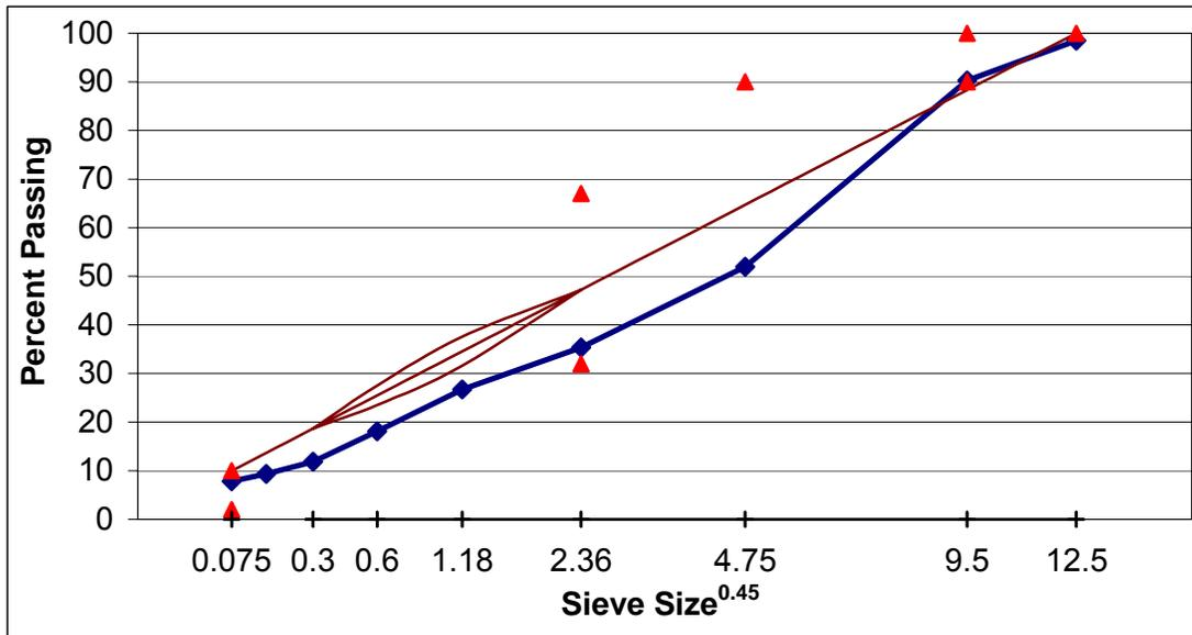
Figure A. 9 Gradation of SM-9.5D, lab-lab mixture, section B.
