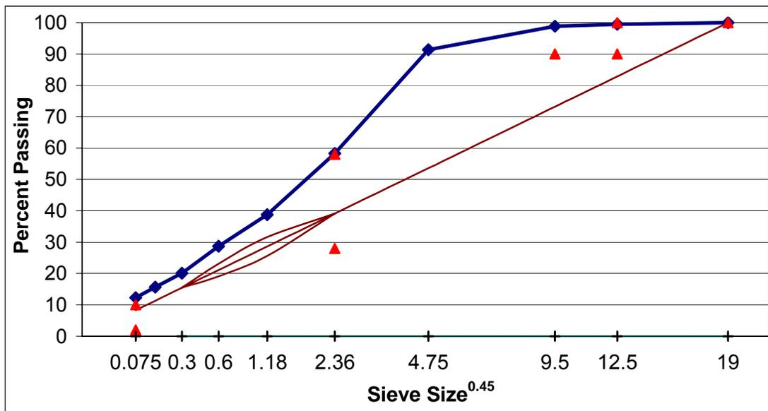
Figure A. 5 Gradation of SM-12.5D, design-lab mixture, section A.
