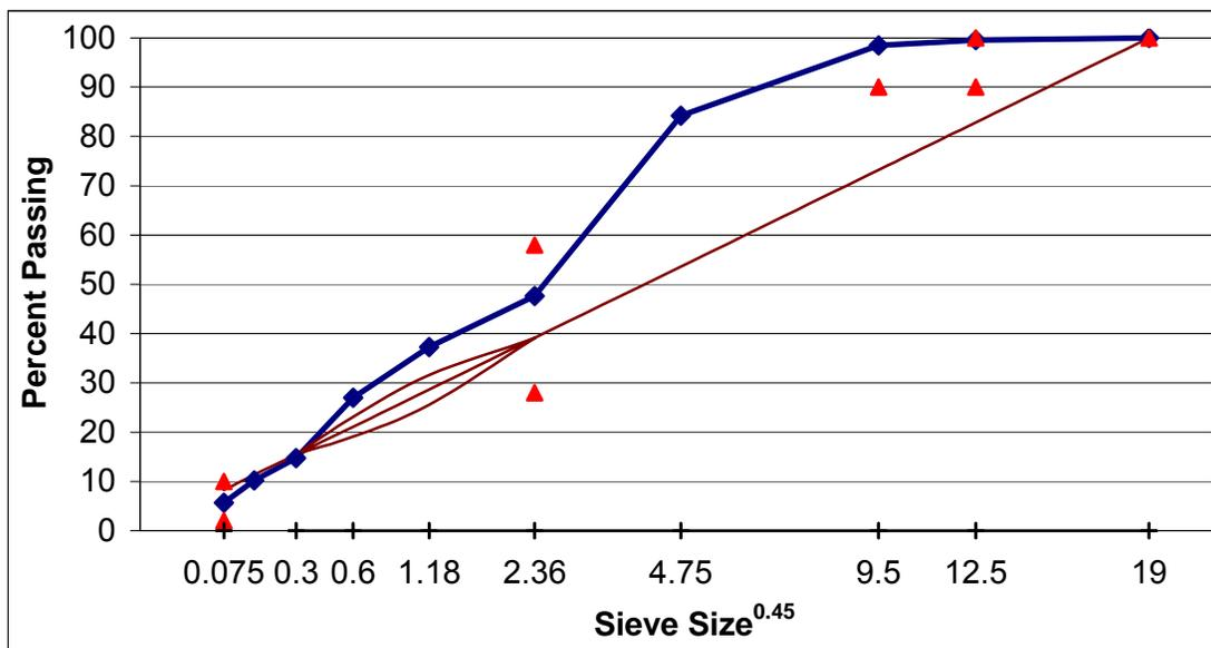
Figure A. 4 Gradation of SM-12.5D, lab-lab mixture, section A.
