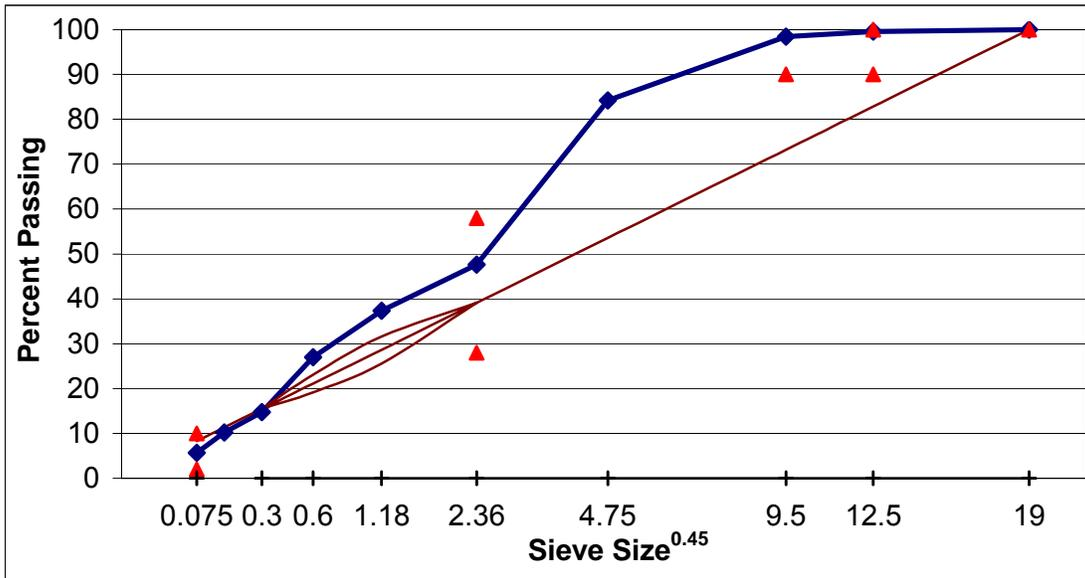
Figure A. 3 Gradation of SM-12.5D, field-lab mixture, section A.
