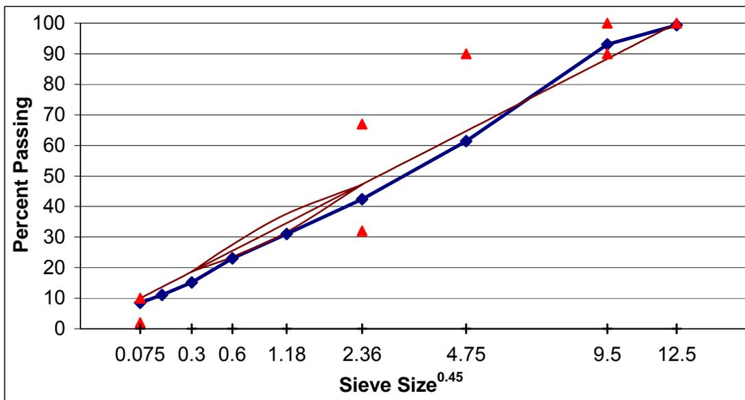
Figure A. 25 Gradation of SM-9.5D, field-field mixture, section F.
