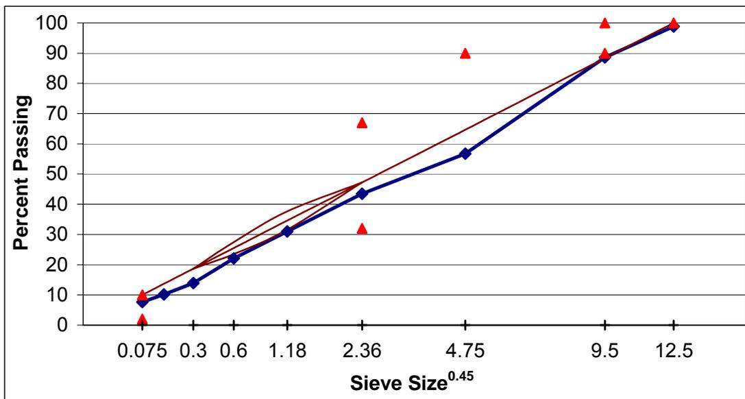
Figure A. 36 Mixture design for SM-9.5D, section J.
