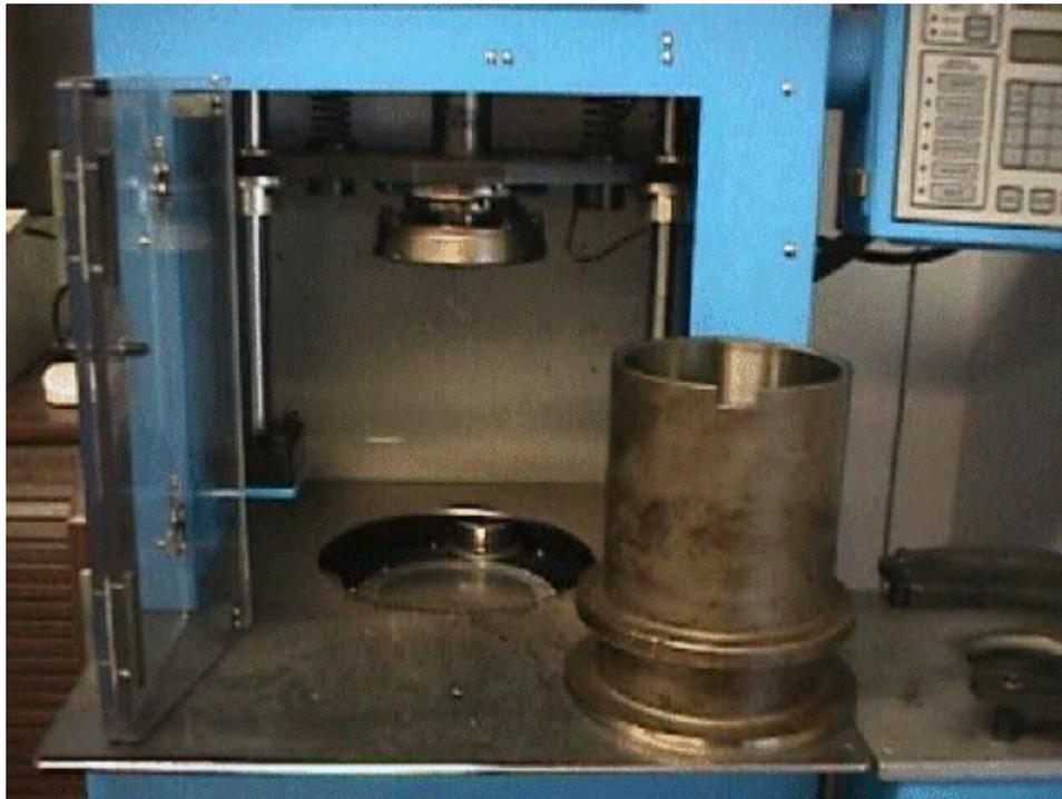
Figure 3-2 Troxler Gyratory Compactor.
