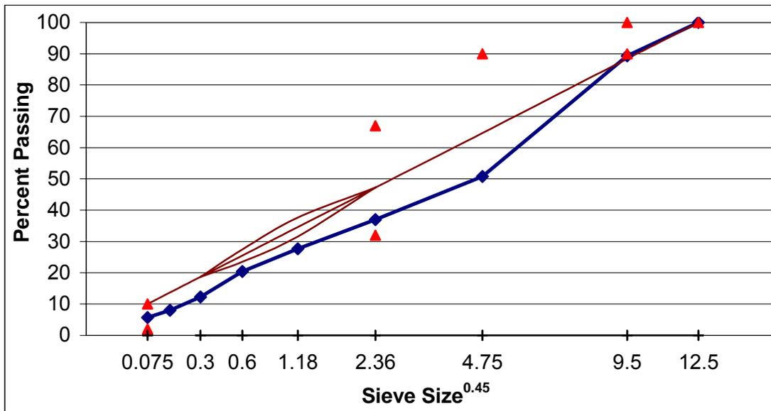
Figure A. 20 Gradation of SM-9.5A, design-lab mixture, section D.
