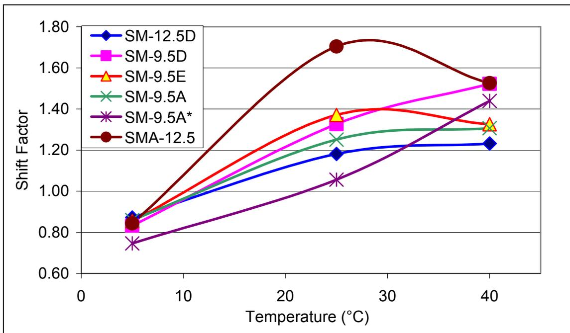
Figure 4-4 Load Duration Shift Factor
