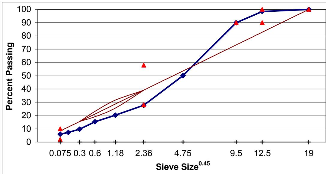
. Figure A. 6 Mixture designs for SM9.5D, section B.
