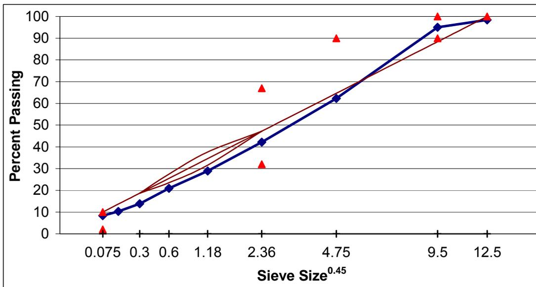
Figure A. 29 Gradation of SM-9.5D, field-field mixture, section H.
