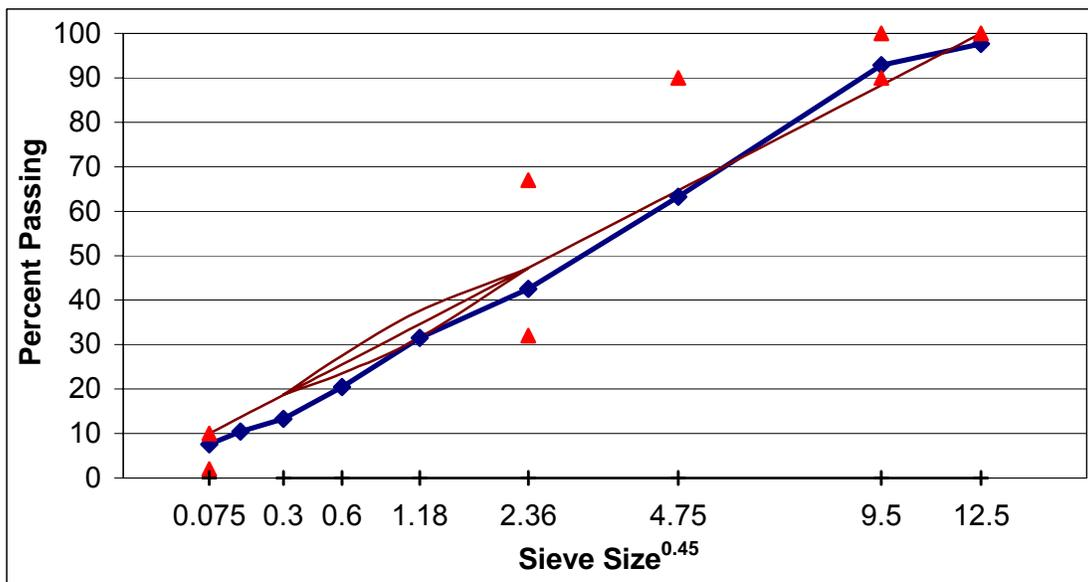
Figure A. 28 Gradation of SM-9.5D, field-lab mixture, section G.
