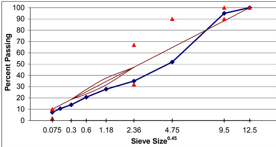
Figure A. 33 Gradation of SM-9.5A, field-lab mixture, section I.
