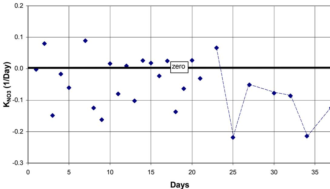
Figure 4-10. Time series of first-order denitrification-rate constants ( $K_{NO_3}$ ) in the fifth experiment.
