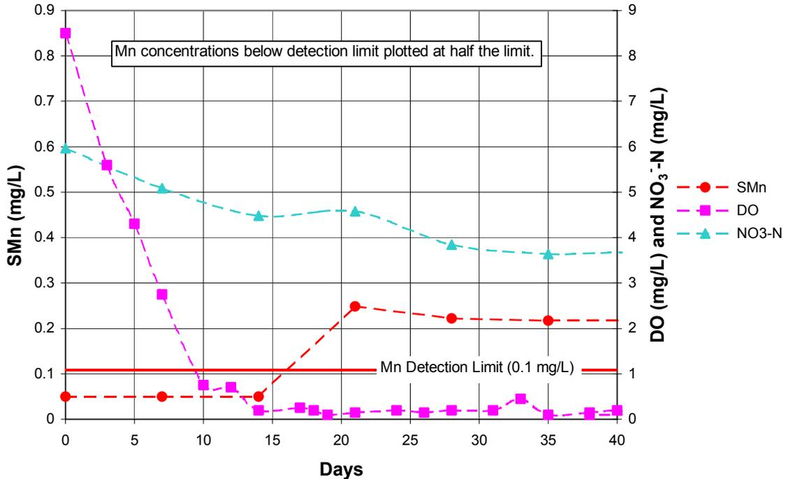
Figure 4-16. Time series of the sixth experiment soluble manganese (SMn), dissolved oxygen (DO), and nitrate (NO<sub>3</sub><sup>-</sup>) in Reactor 1.
