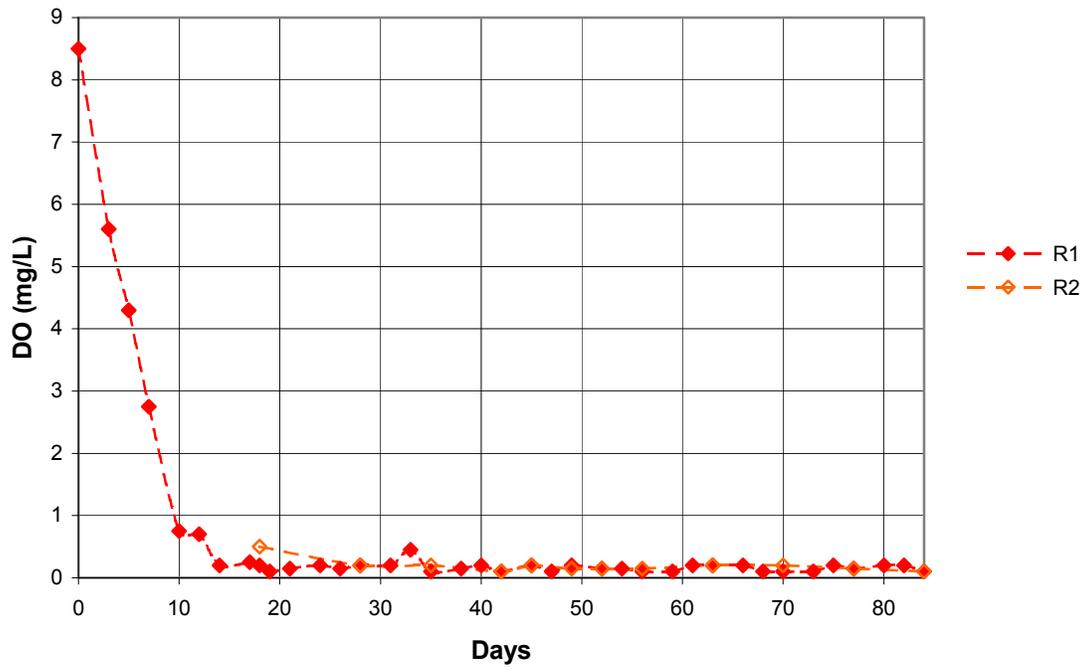
Figure 4-11. Time series of sixth experiment dissolved oxygen concentrations in the solution of the first (R1) and second (R2) reactors.
