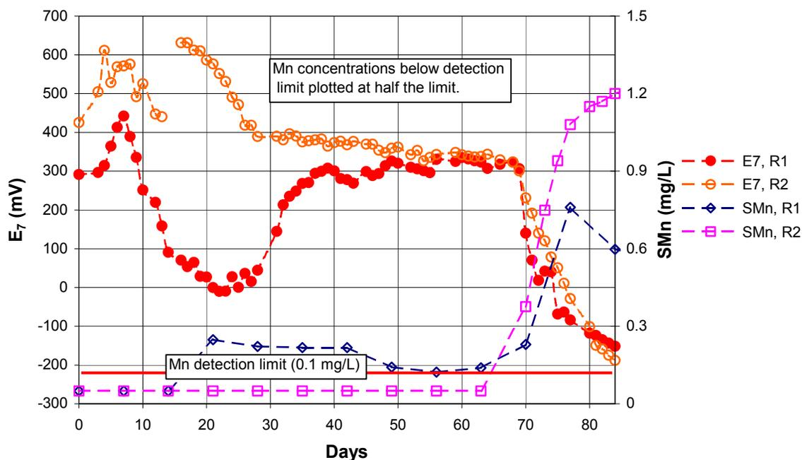
Figure 4-20. Time series of Experiment 6  $E_7$  and soluble manganese (SMn) in the water column of the first (R1) and second (R2) reactors.
