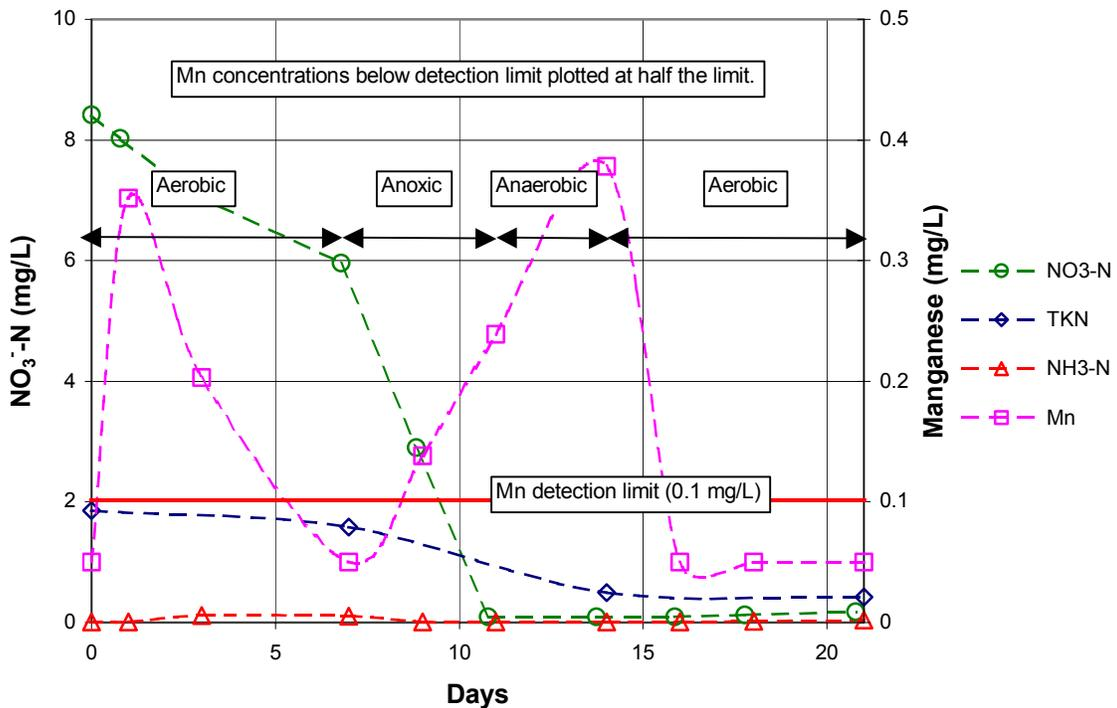
Figure 4-17. Time series of Experiment 7 nitrate (NO<sub>3</sub>), total Kjeldahl nitrogen (TKN), ammonia (NH<sub>3</sub>), and manganese (Mn) in the seventh experiment.
