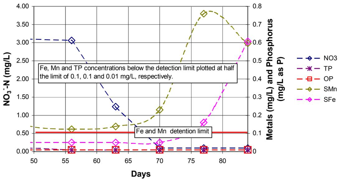
Figure 4-24. Time series of nitrate ( $\text{NO}_3^-$ -N), total phosphorus (TP), orthophosphate phosphorus (OP), soluble manganese (SMn), and soluble iron (SFe) in Reactor 1 of Experiment 6.
