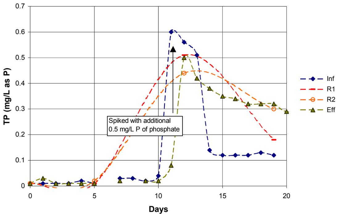
Figure 4-6. Time series of fourth experiment total phosphorus concentrations in feed water (Inf), Reactor 1 (R1), Reactor 2 (R2), and the effluent (Eff).
