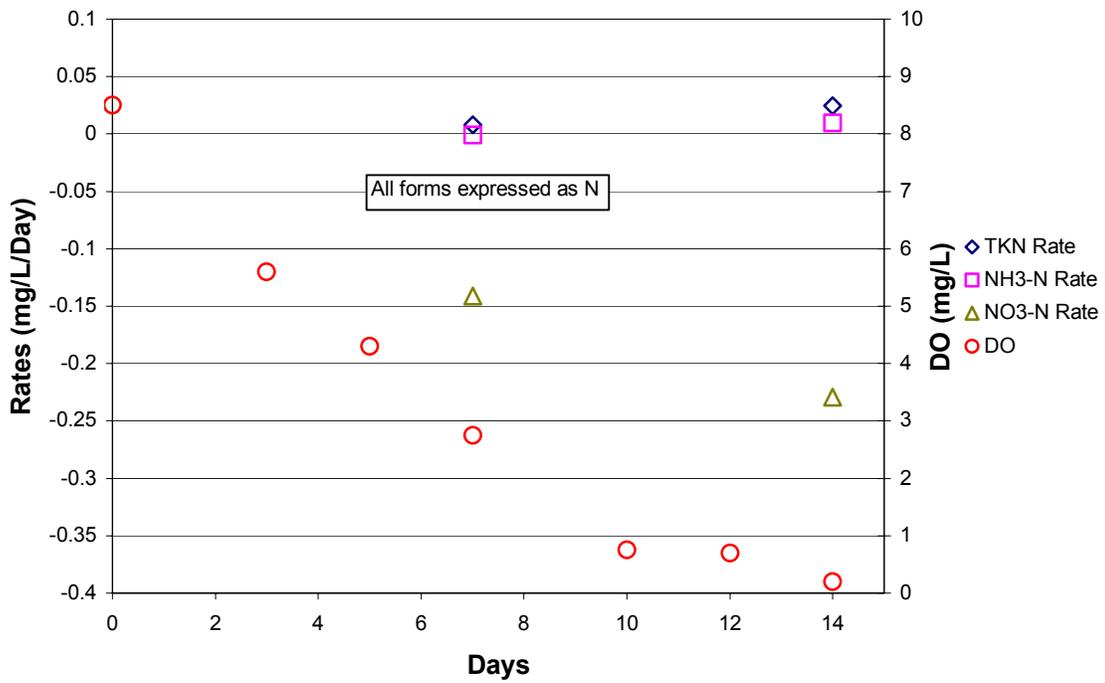
Figure 4-14. Time series of the rates of nitrogen transformations and dissolved oxygen depletion in the first reactor of Experiment 6.
