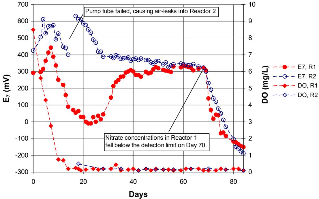
Figure 4-19. Time series of sixth experiment dissolved oxygen (DO) concentrations and  $E_7$  in the water column of the first (R1) and second (R2) reactors.
