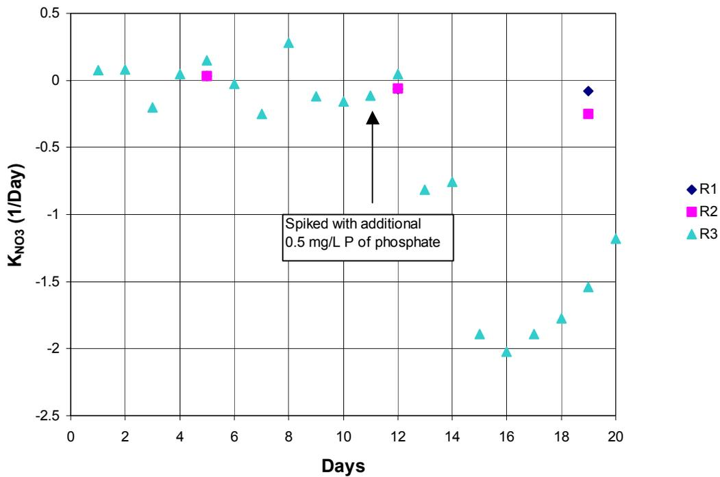
Figure 4-7. Time series of the first-order denitrification-rate constants ( $K_{NO_3}$ ) in Reactor 1, 2, and 3 of Experiment Four.
