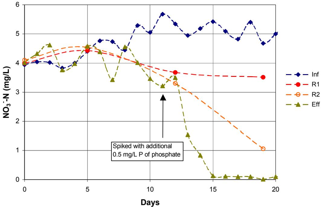
Figure 4-5. Time series of fourth experiment nitrate concentrations in feed water (Inf), Reactor 1 (R1), Reactor 2 (R2), and the effluent (Eff).
