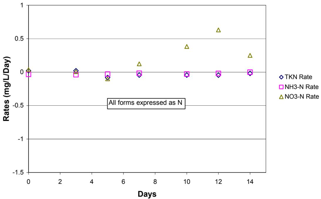
Figure 4-15. Time series of the rates of nitrogen transformations in the second reactor of Experiment 6.
