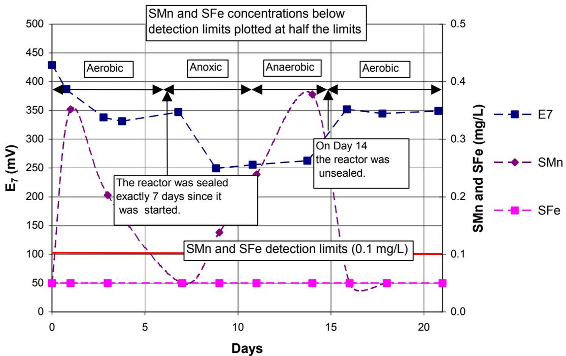
Figure 4-23. Time series of Experiment 7  $E_7$ , soluble manganese (SMn), and soluble iron (SFe) in the reactor solution.
