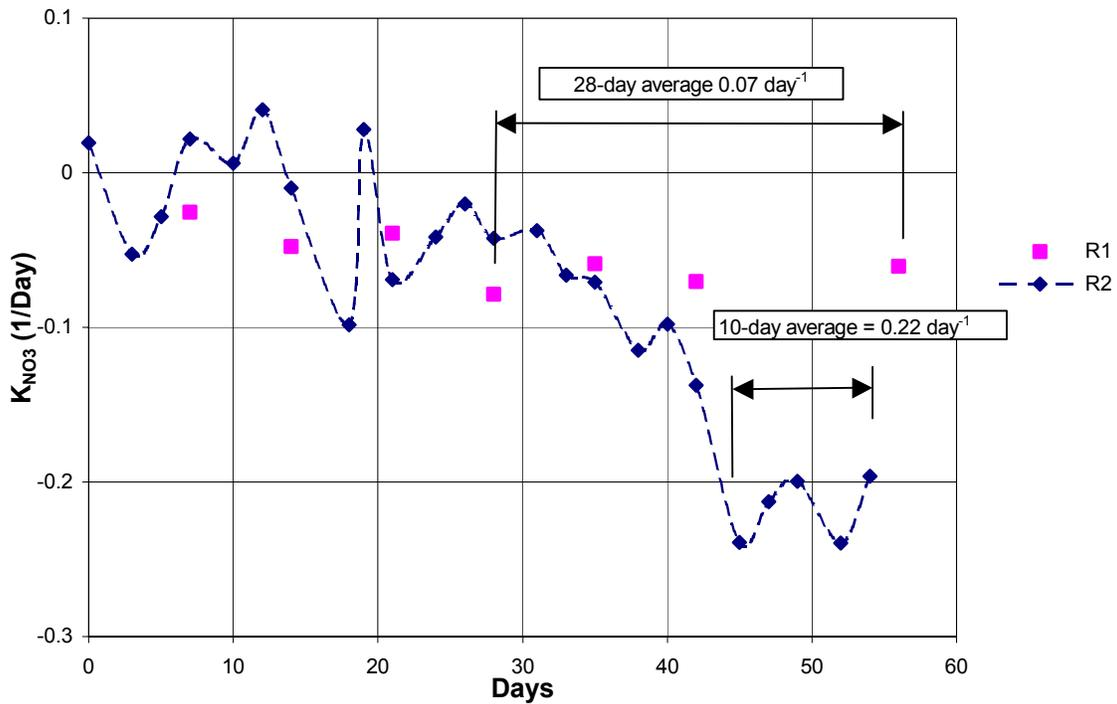
Figure 4-13. Time series of sixth experiment denitrification-rate constants ( $K_{NO_3}$ ) in the first (R1) and second (R2) reactors.
