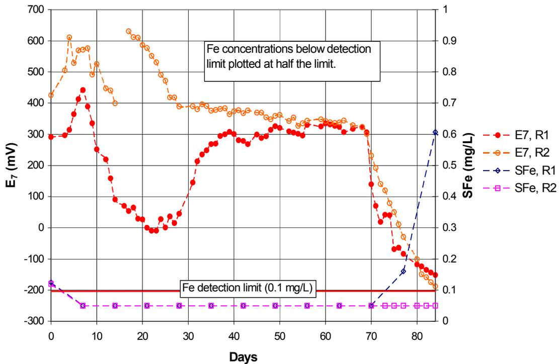
Figure 4-21. Time series of Experiment 6 E<sub>7</sub> and soluble iron (SFe) in the solution of first reactor (R1), and second (R2) reactors.
