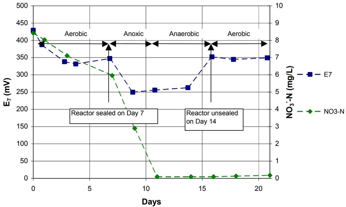
Figure 4-22. Time series of Experiment 7  $E_7$  and nitrate ( $\text{NO}_3^-$ ) concentrations in the solution.
