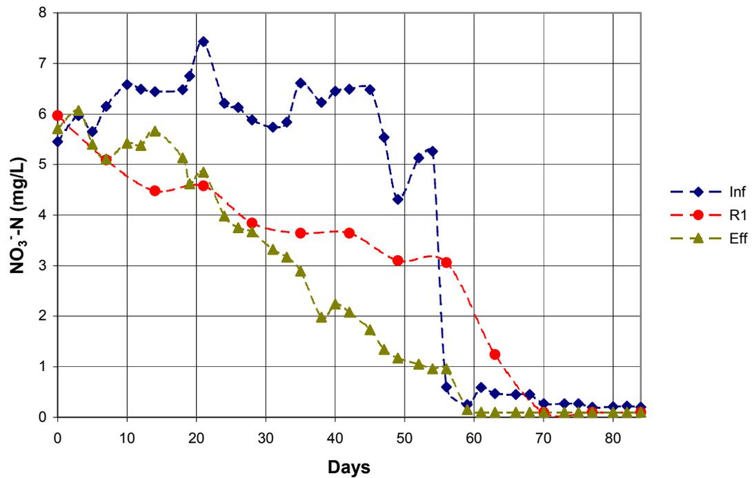
Figure 4-12. Time series of sixth experiment nitrate concentrations in the influent (Inf), first reactor (R1) and effluent (Eff).
