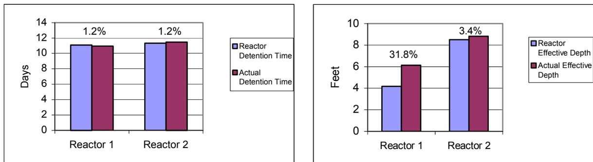
Figure D-1. Comparison between the actual reservoir and the sixth-run reactors
