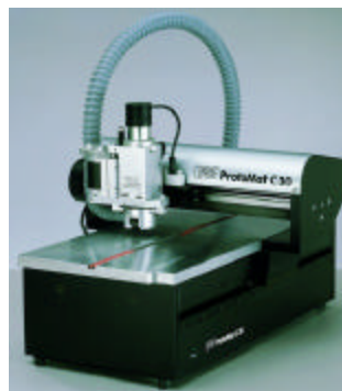
Figure 24. LPKF milling station used to fabricate patch antennas
