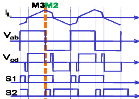
Figure 3-31 key waveforms of steady state operation mode: M3M2M4M8M7M9
