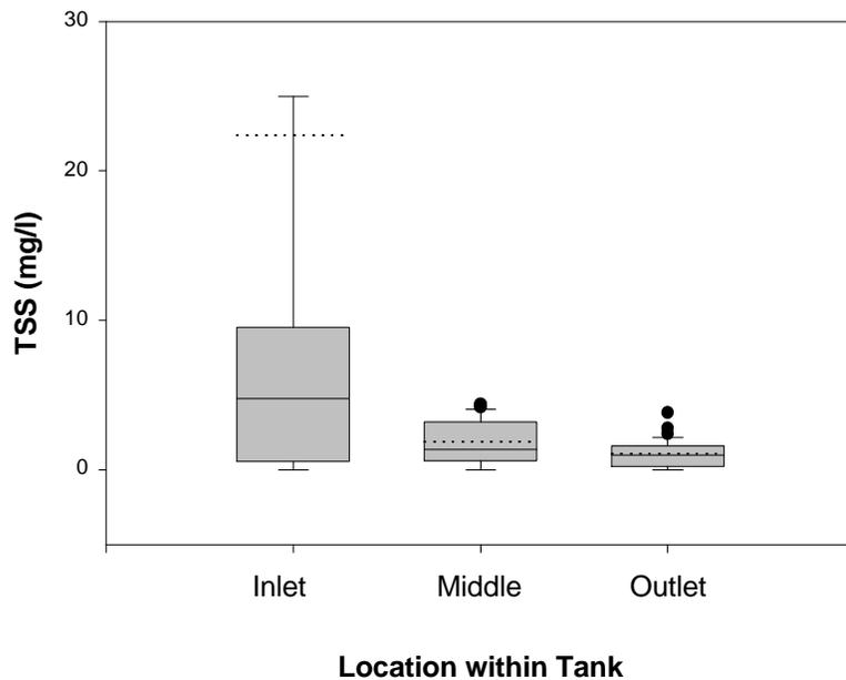
Figure 5. Pilot TSS data during 20-minute detention time trial. Note: Two inlet samples are off the scale (106 and 326 mg/l).
