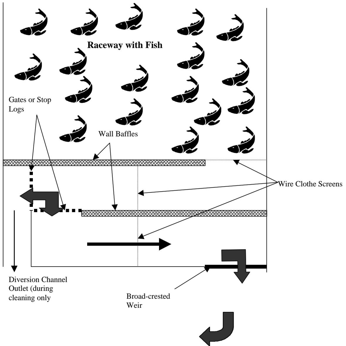
**Fig. 1.** Sample schematic of proposed treatment scheme (two baffles).
