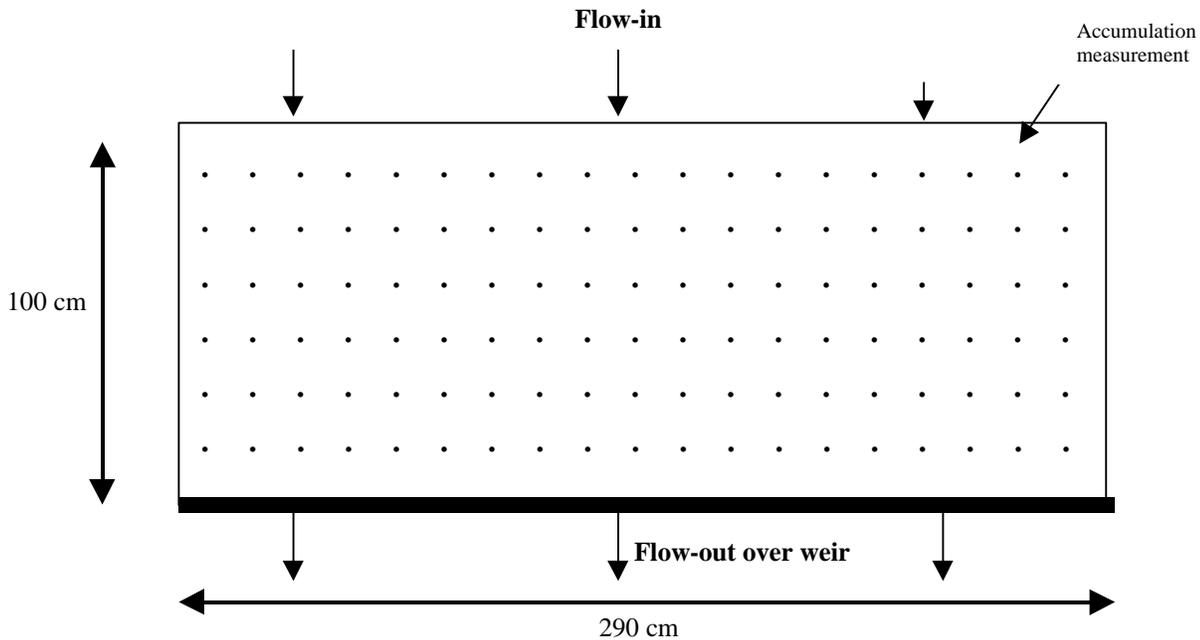
Fig. 1. Example of grid system used at Farm C for one of the sediment traps in the observed raceway.
