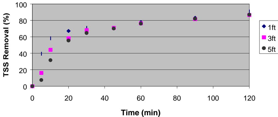
Figure 2. Type II settling results using average values from the 8-Day batch study.
