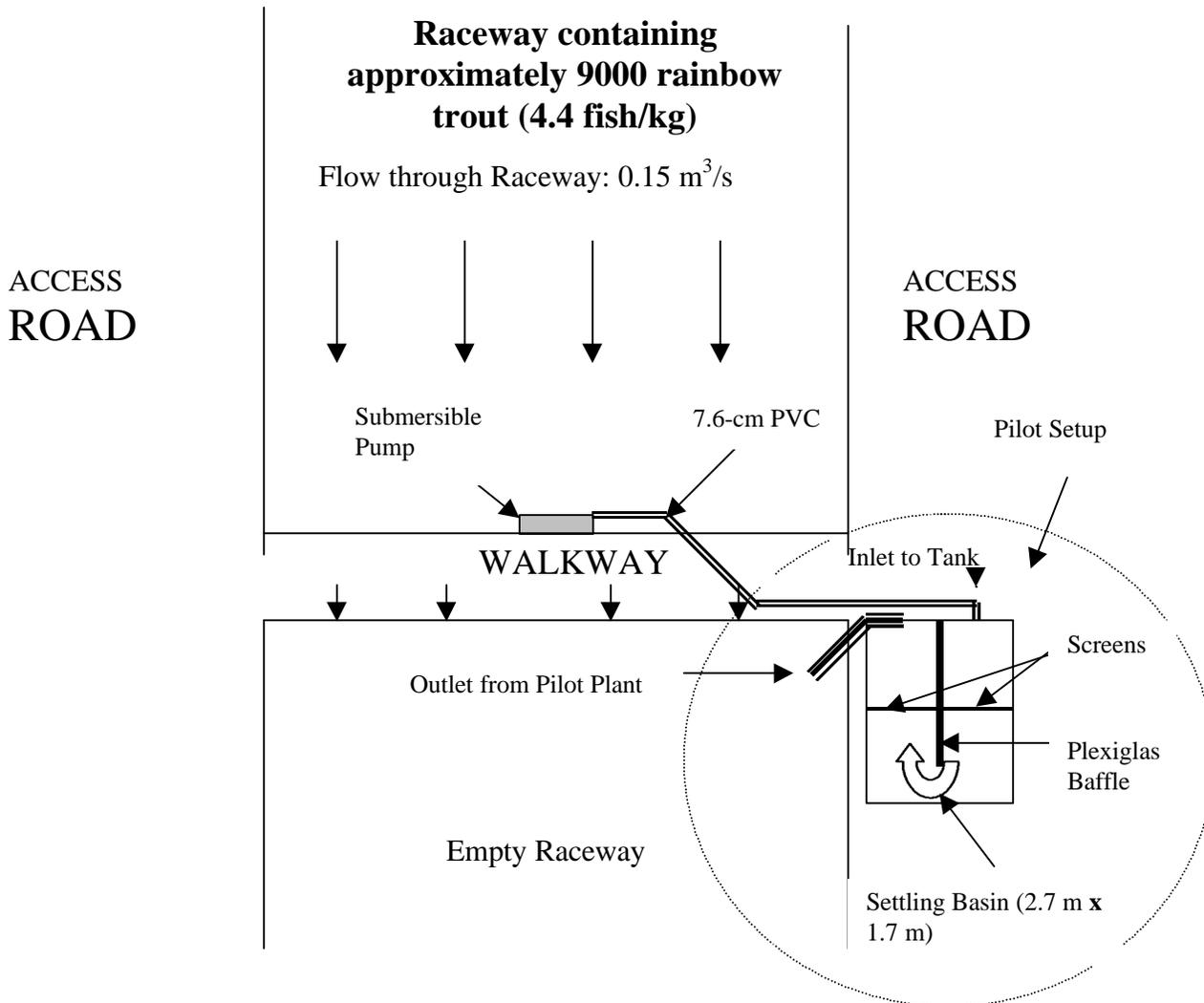
Figure 1. Pilot plant layout at Farm C.
