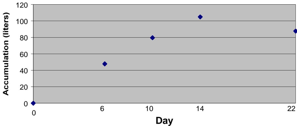
Fig. 8. Sludge accumulation at Farm C as a function of time for days 0 – 22.
