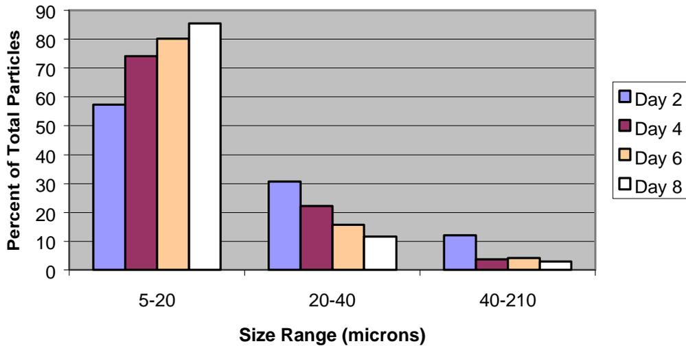
Fig. 6. Change in particle count distribution during batch study.
