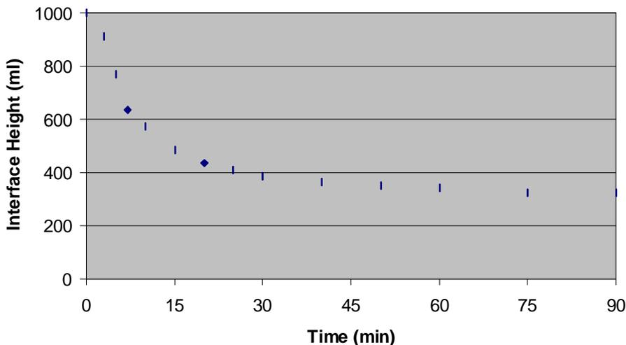
Figure 3. Type III settling results for sludges encountered during 3-week sludge accumulation experiment (average initial TSS = 25,400 mg/l).
