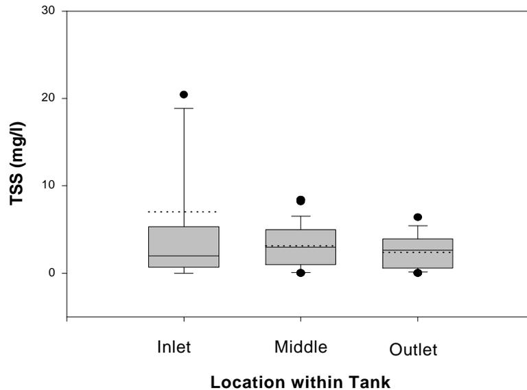
Figure 4. Pilot TSS data during 10-minute detention time trial. Note: Two inlet samples are off scale (39.4 and 79.5 mg/l).
