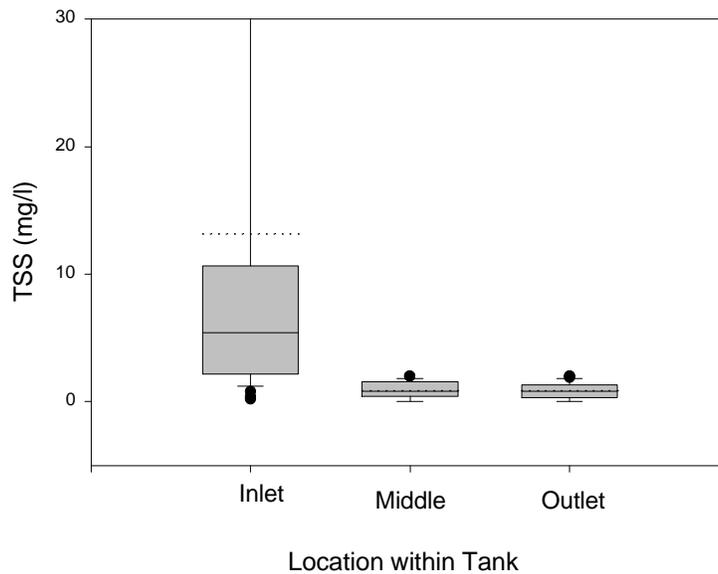
Figure 6. Pilot TSS data during 30-minute detention time trial. Note: Four inlet samples are off the scale (75.6, 90.8, 36.0, and 41.0 mg/l); also, upper whisker for inlet samples is off scale (39 mg/l).
