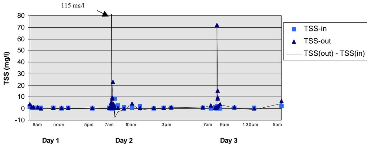
Fig. 2. TSS Concentrations for Raceway II during days 1-3 of a 1-week intensive sampling study.
