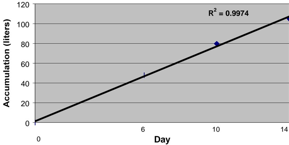
Figure 7. Sludge accumulation at Farm C as a function of time for days 0 – 14.
