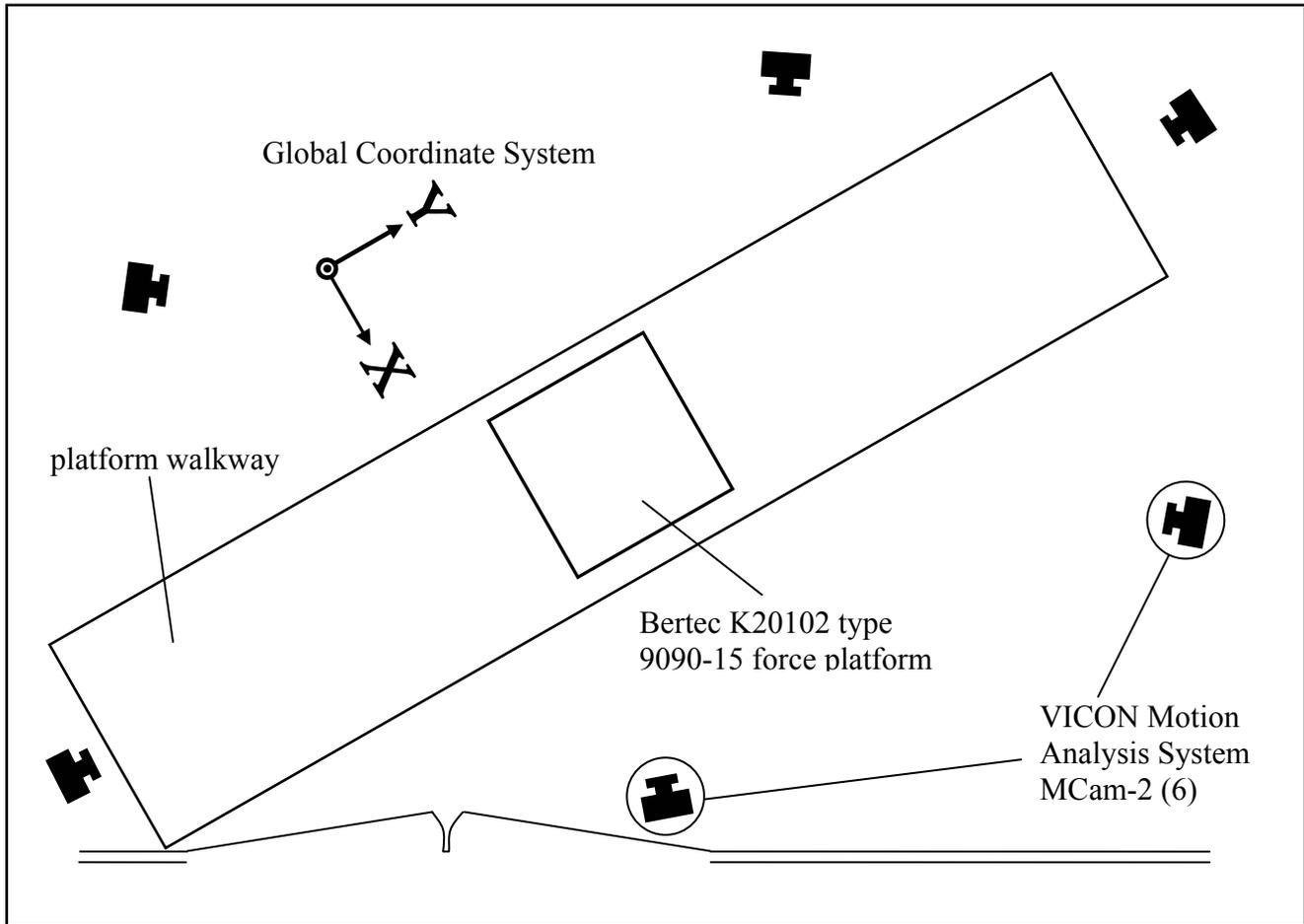
Center of pressure data was collected by Bertec K20102 type 9090-15 force platform and marker position data was collected with the VICON 460 Motion Monitoring System as seen in the configuration above.
