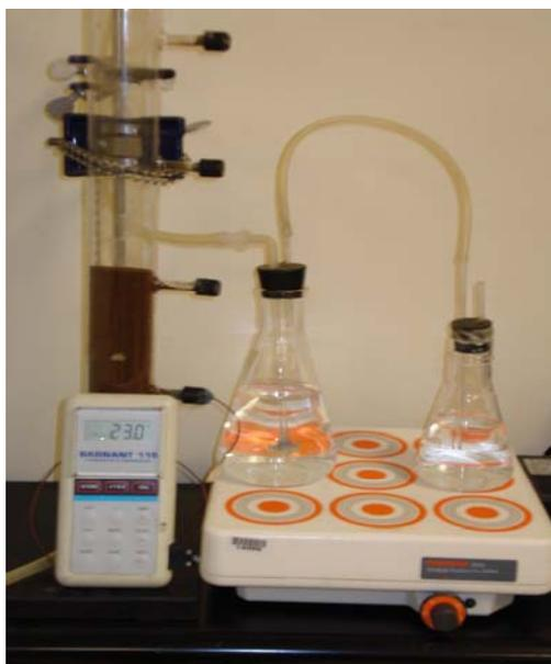
Figure 3.2 Experimental set up of ammonia adsorption in a packed bed reactor
