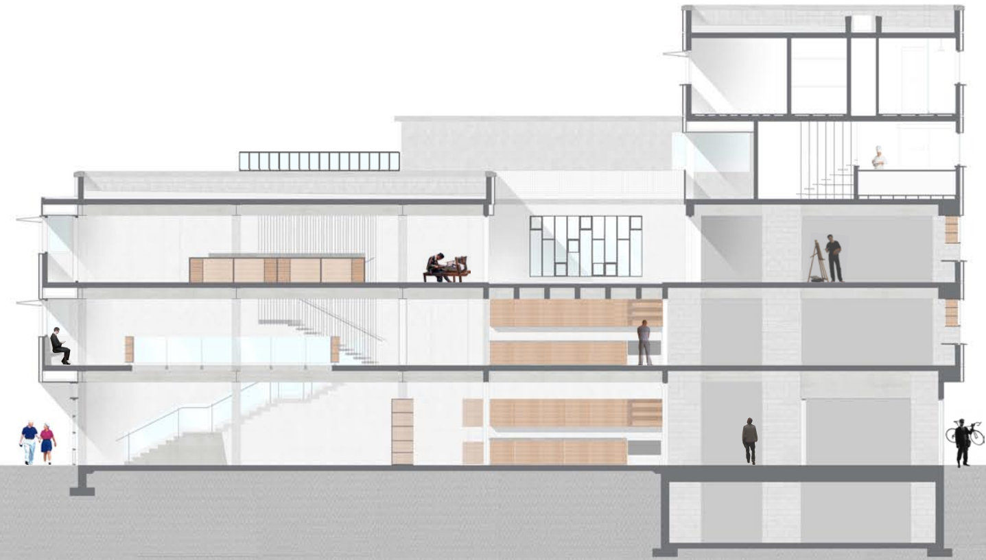
building section two - school/studios and duplex apartments
