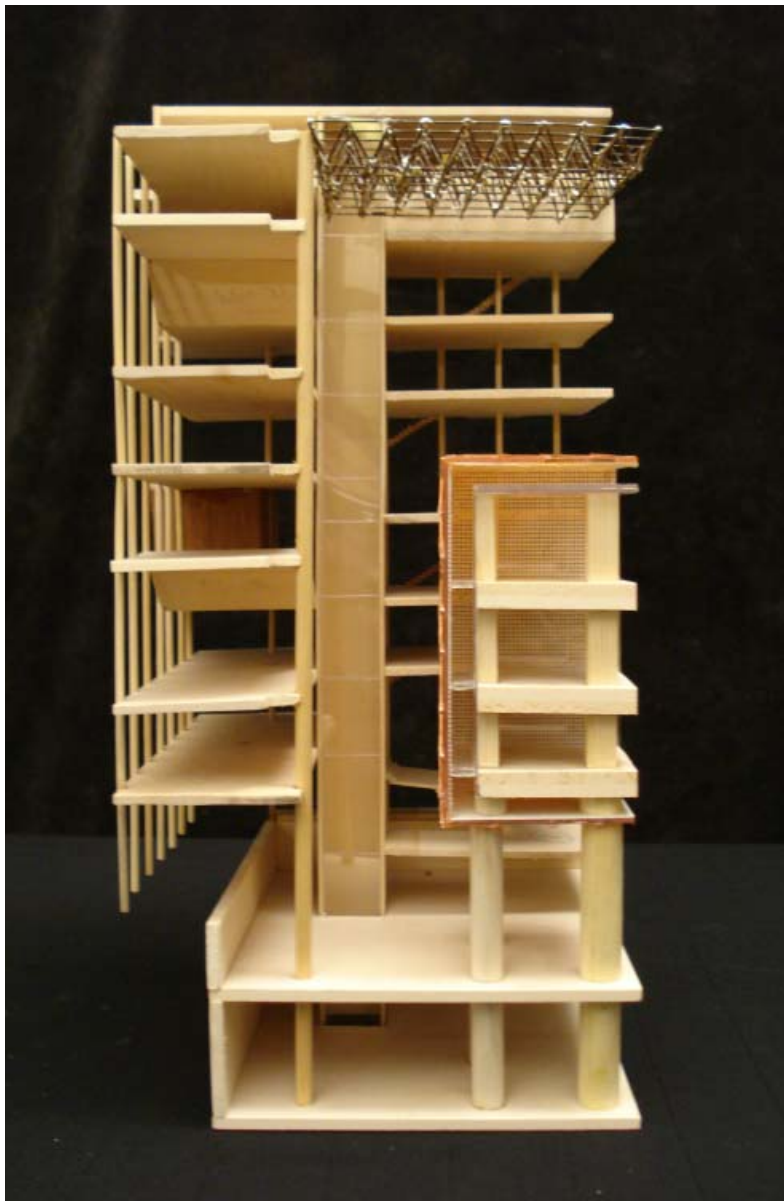
1/4" = 1'-0" MODEL PARTIAL SECTION CUT THROUGH OFFICE WING AND PART OF THE CLEANROOM. THE LABORATORIES, LIBRARY AND ELEVATOR CAN BE SEEN IN THE BACKGROUND.
