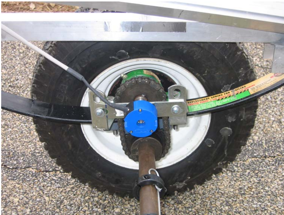
Figure 23. Placement of the encoder to measure wheel speed and position.
