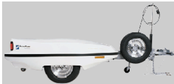
Figure 6. Superflow's TD-1200 towable dynamometer [12]
