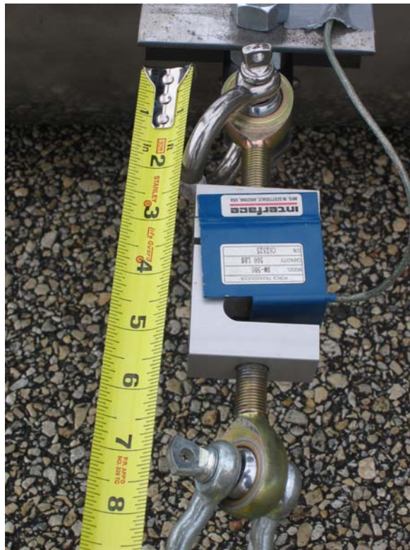
Figure 19. Close-up view of load cell connected inline the tow chain.
