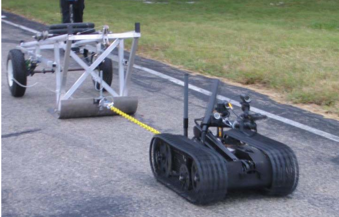
Figure 26. TALON undergoing pull test.
