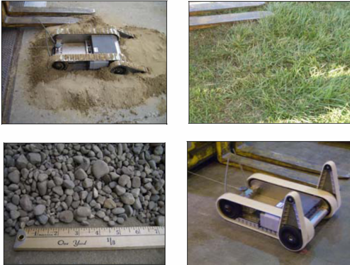
Figure 9. Packbot undergoing static drawbar tests in various terrain. [14]
