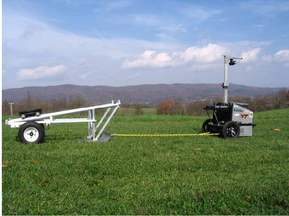
Figure 18. Johnny 5 undergoing a tow test at JOUSTER Field Day, 10-30-04
