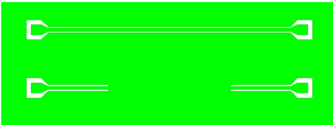
Figure 6.14: Line and Reflect (short) TRL standards used in the Mechanical Fit calibration.
