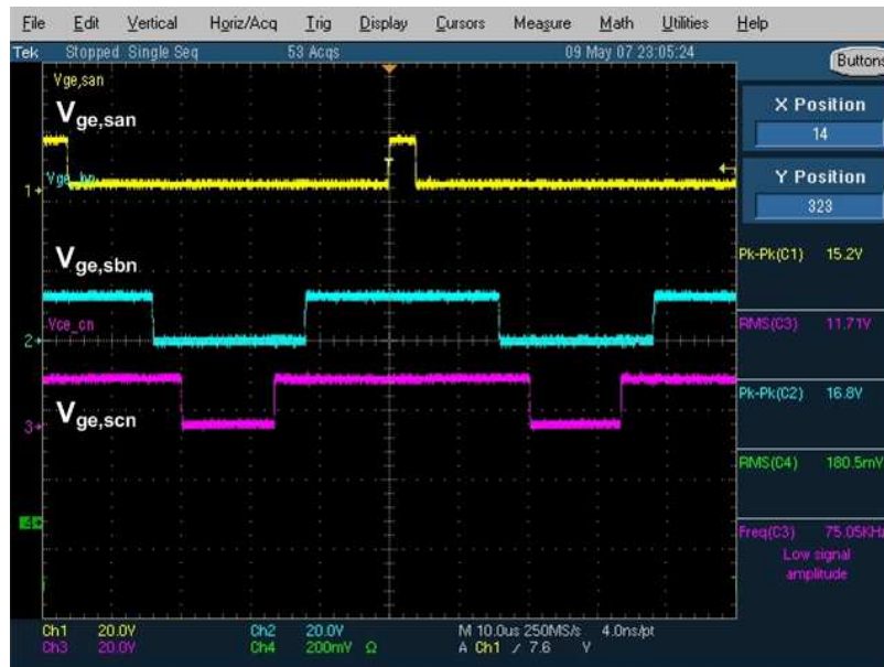
Figure 2-10: Gate drive voltages (bottom switches). 20 V/div, 10 \mu s/div
