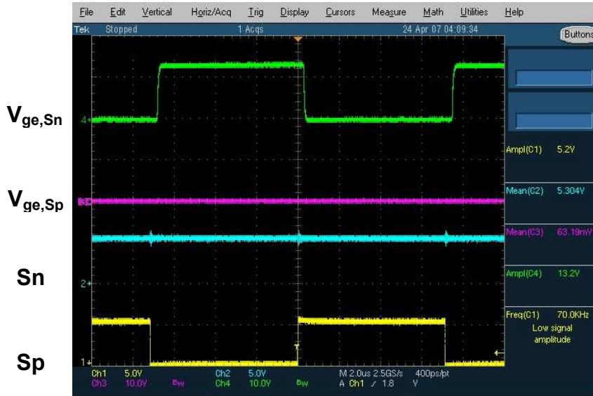
Figure 2-14: Anti-shoot-through logic test for S_n = \text{HIGH}
