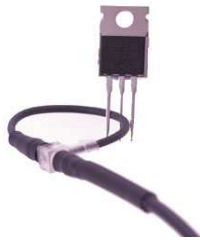
Figure 2-12: IGBT current measurement using Rogowski coil
