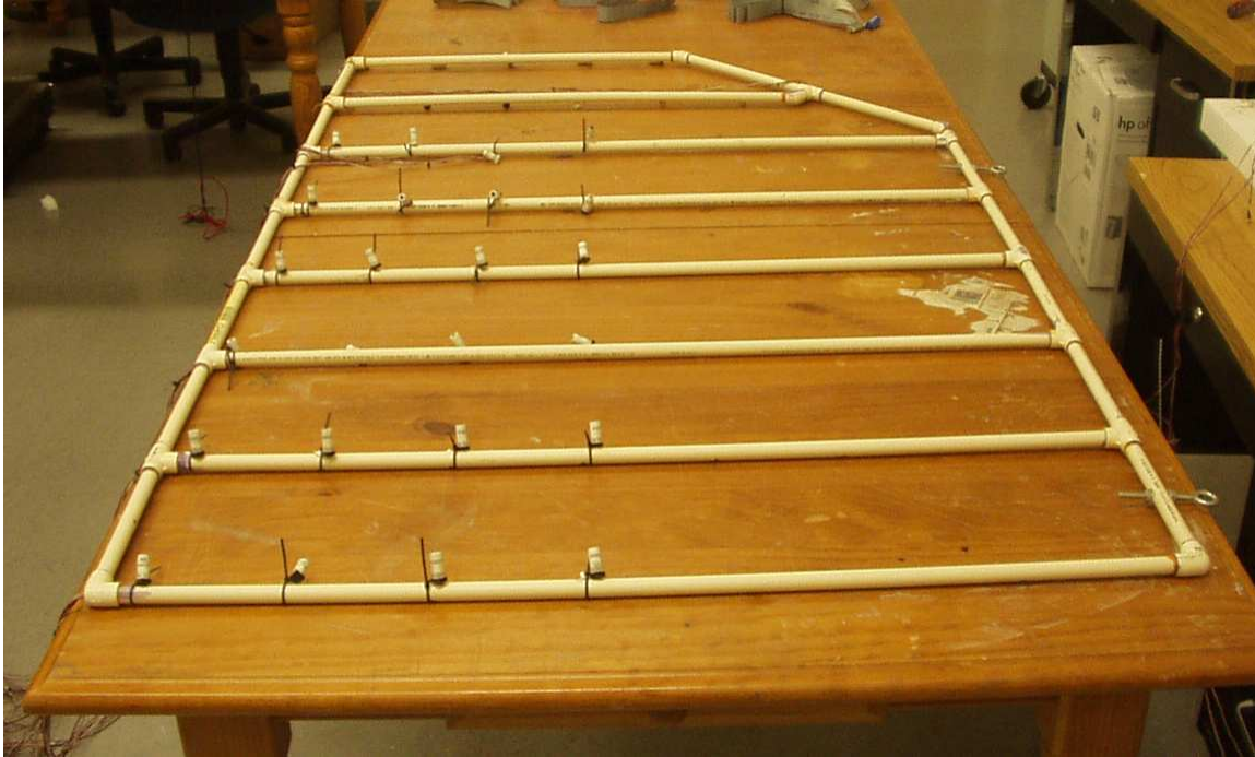
Figure 4.7. Planar microphone array. This setup allows for the rapid measurement of “microphone output per shaker input” FRFs at all locations inside the enclosure.
