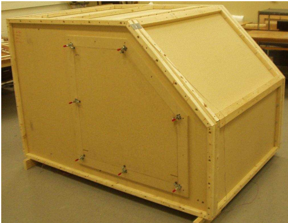
Figure 4.2. Structural acoustic test platform, complete with door. The door panel clamps into its slot from the outside, leaving a smooth interior wall.
