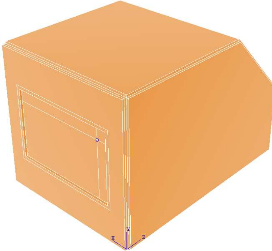
Figure 3.5. Assembly of the enclosure. The Lexan and MDF panels were sized around the acoustic space (hidden by panels), and the panel faces were mated to the faces of the acoustic space.
