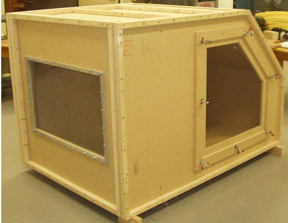
Figure 4.1. Structural acoustic test platform, complete but without door. The enclosure was constructed from six subassemblies that are all bolted together along their outside edges.
