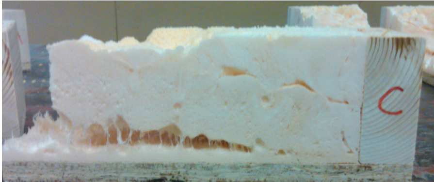
Figure 4-10: Cross section view of air gap formed between the sheathing and the spray-applied polyurethane foam within a 2x4 building enclosure.
