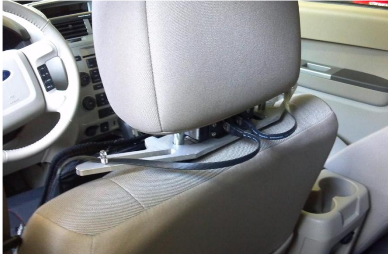
Figure 27. The headrest mount behind the driver's shoulders connects the DriveGrip's ethernet cables and allows the SpeedStrip interface to strap in rigidly to the seat
