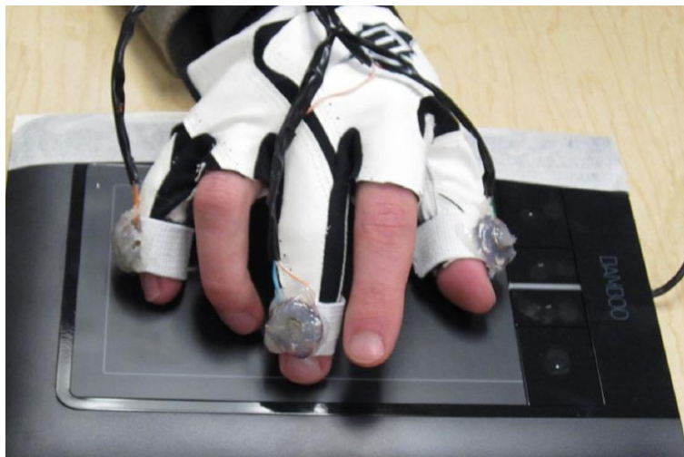
Figure 36. An early prototype of the Kinesthetic Tactile Display
