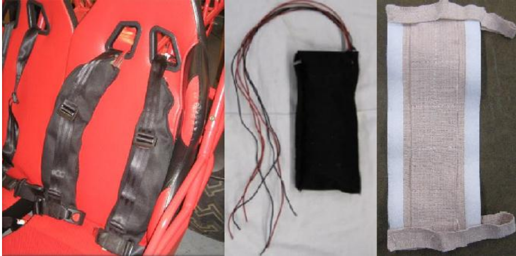
Figure 13. Speed control interfaces: integration into the seatbelt, and two interfaces attached to the driver's thigh
