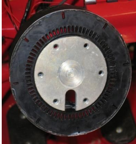
Figure 8. Click Wheel mounted on the steering column of the dune buggy
