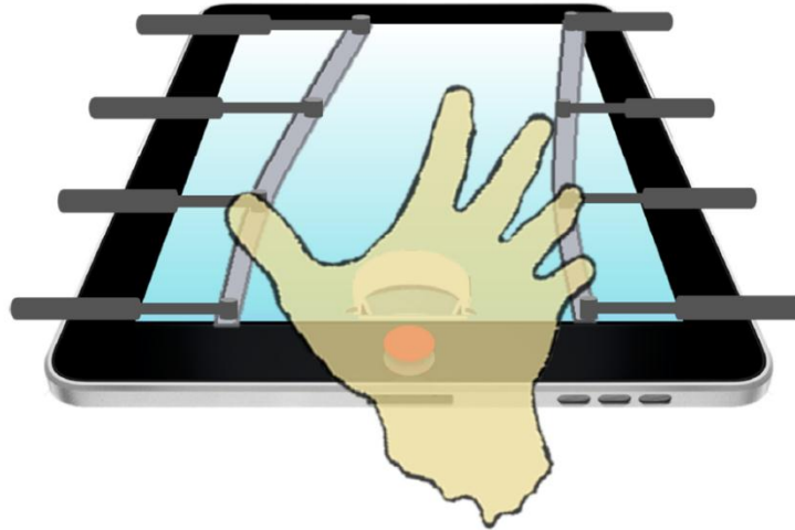
Figure 35. The concept of lane markers, shown with the static vehicle reference and signaling a right-hand curve
