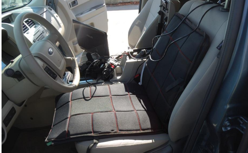
Figure 28. The SpeedStrip interface is a seat cushion with vibration motors positioned up the back and down the thighs
