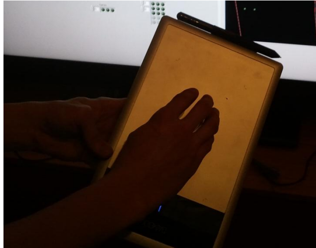
Figure 37. The second generation prototype for the Kinesthetic Tactile Display demonstrating multi-touch exploration of the two-dimensional environment
