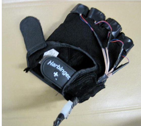
Figure 12. The final design concept for the DriveGrip interface, with vibrotactile motors on knuckles as shown
