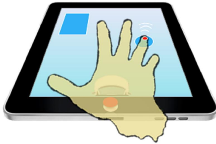
Figure 22. A touchpad interface platform is an example that may be used to provide truly active feedback to the blind driver
