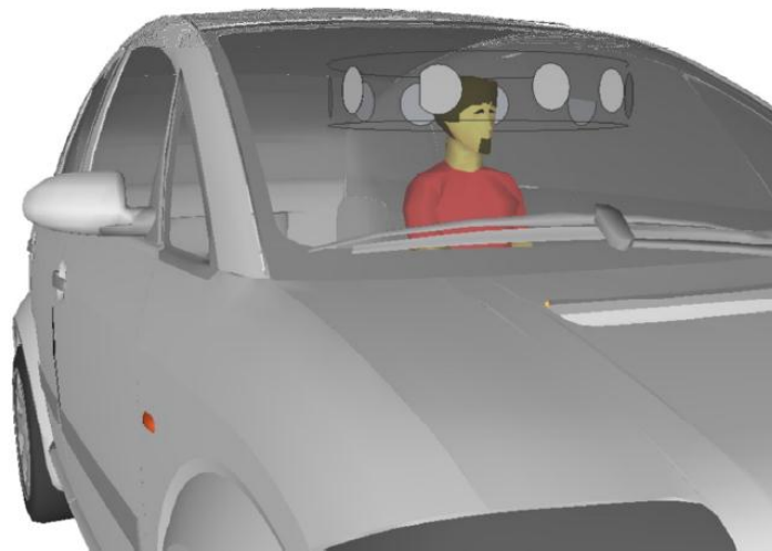
Figure 34. Representation of a possible implementation of the three-dimensional sound system
