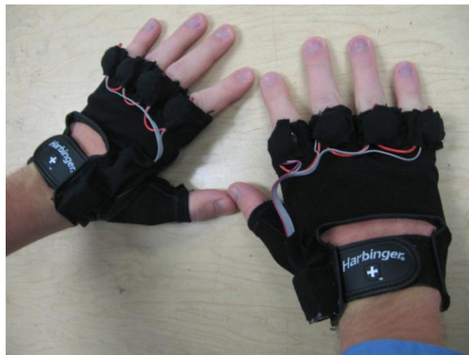
Figure 25. The DriveGrip interface is a pair of gloves with a vibration motor positioned on the base segment of each forefinger
