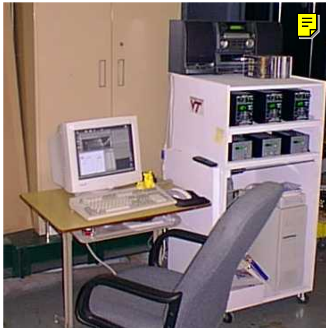
Figure 3.10: Virginia Tech DGV control cart: iodine cell stem temperature controllers on top shelf, body controllers on middle shelf, and control computer on bottom
