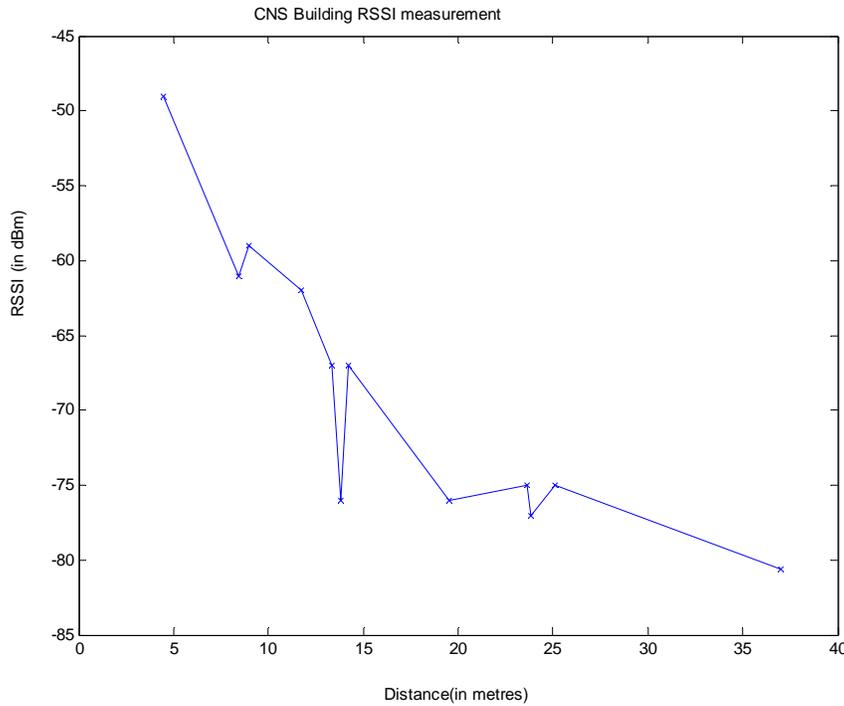
**Figure 5.5: Signal Strength at CNS Building**
