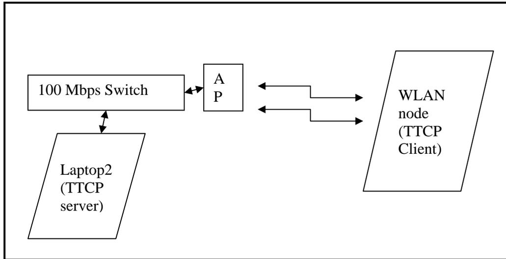
*Figure 5.1: Throughput measurement setup*
