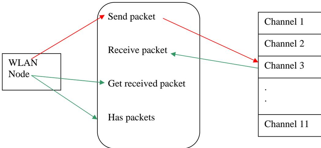
**Figure 4.2: Interaction of Channel Interface class**
