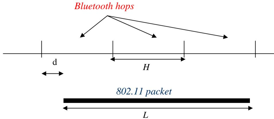
**Figure 3.1: Bluetooth and WLAN frame Collision**
