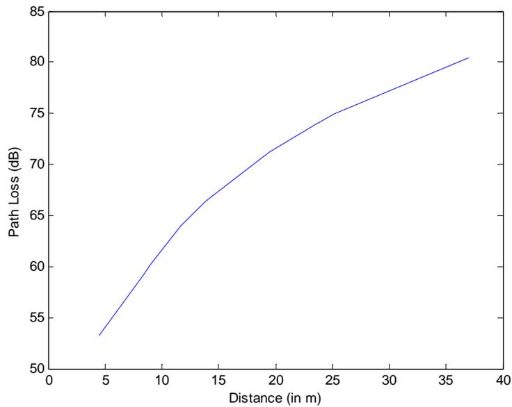
**Figure 5.6: Path Loss at CNS Building**
