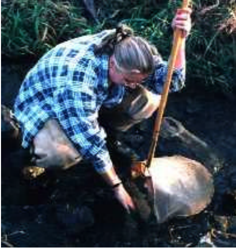
Figure 4. Professional method for sampling stream macroinvertebrates with a D-frame dip net. The net was approximately 0.3 m wide on the bottom. An area of approximately 0.1 m 2 in front of the net was disturbed with the hands for 15 sec. The sample consisted of 2 subsamples from fast current and 2 subsamples from slow current.
