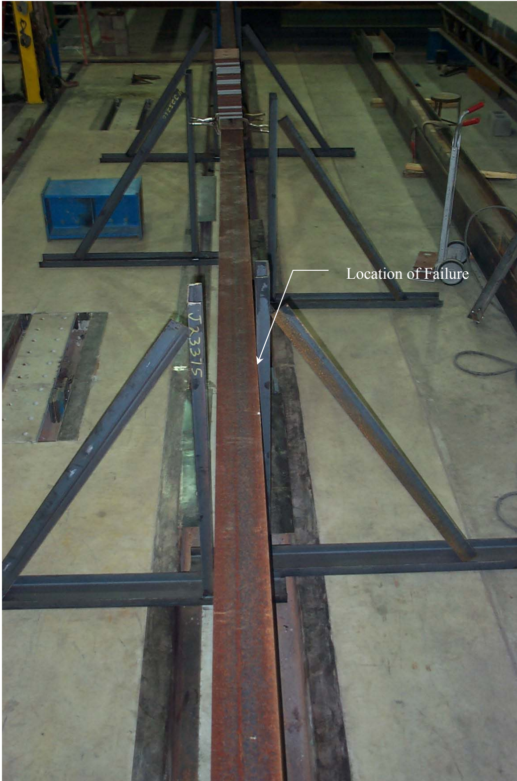
Photo of CB24x26 Specimen at failure
