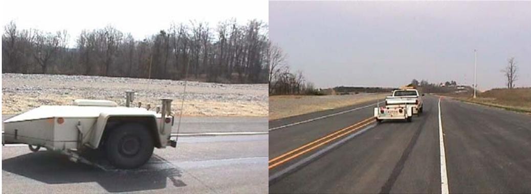
**Figure 2.1 Locked Wheel Skid Trailer.**
