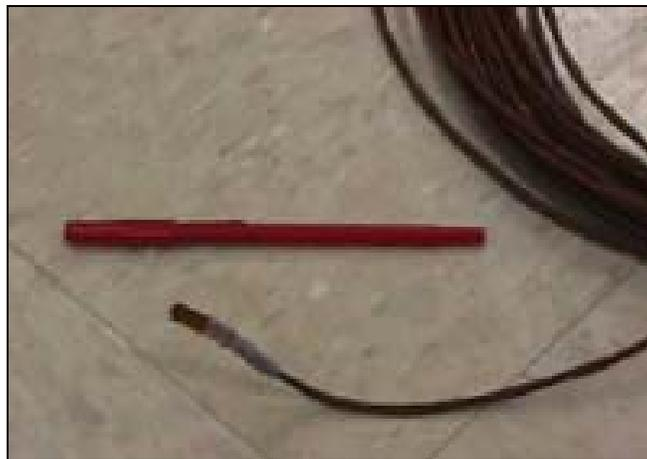
**Figure 3.2 T-shape Thermocouple**
