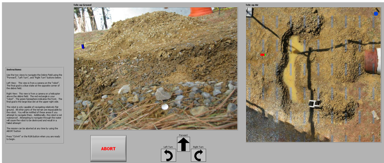
Figure 5.7: Operator Display Interface presented to user for assessment of the combined in-situ and aerial monovision systems
