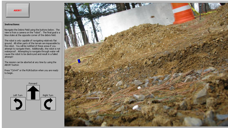
Figure 5.6: Operator Display Interface presented to user for assessment of the in-situ monovision and the aerial monovision (display similar for both systems)
