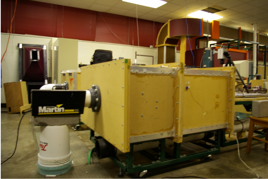
Figure 21. Photograph showing the location of the fog machine on the upstream side of the plenum.
