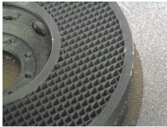
Figure 7 The interior of a fast build part being fabricated [ARC 2006].
