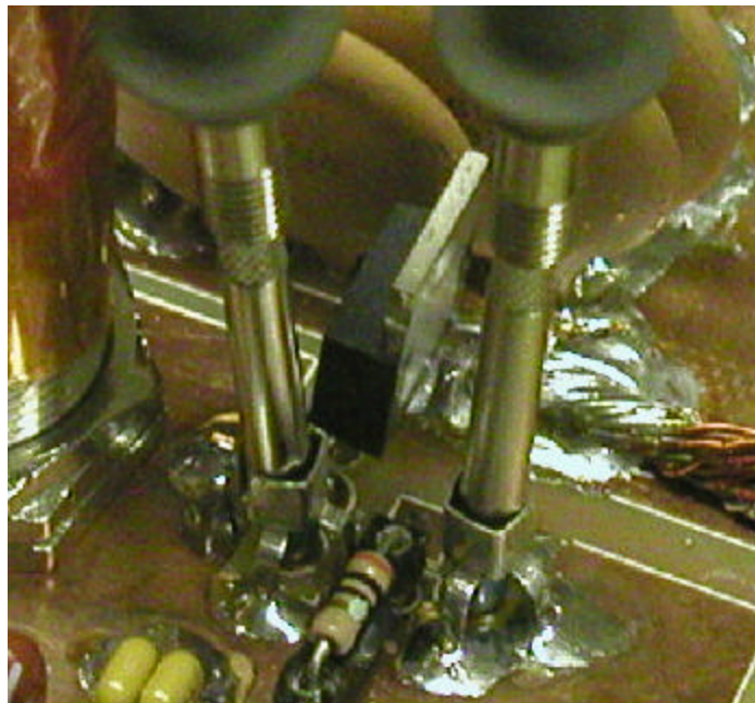
Figure 2.9. Reduced tip-to-ground loop using a probe-tip adaptor.
