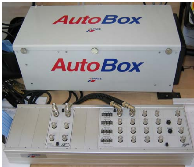
Figure 6-4 dSPACE AutoBox Control Prototyping Box
