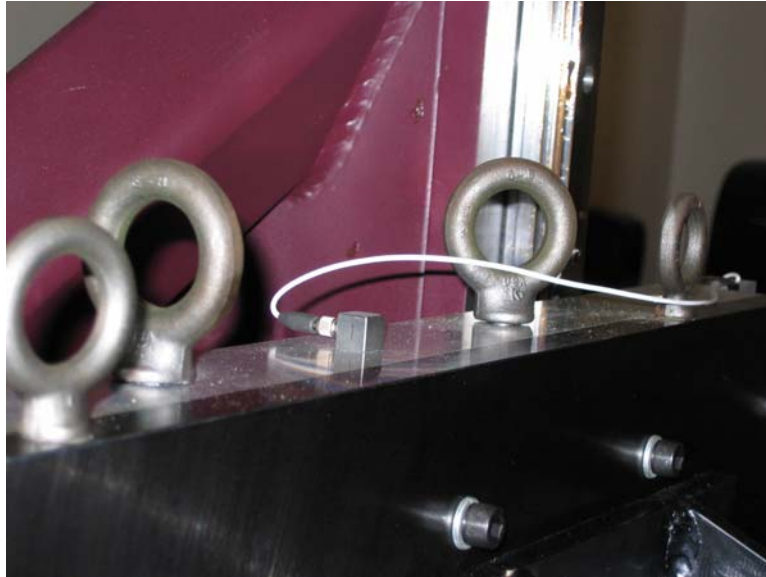
Figure 6-1 Accelerometer Installed on Sprung Mass
