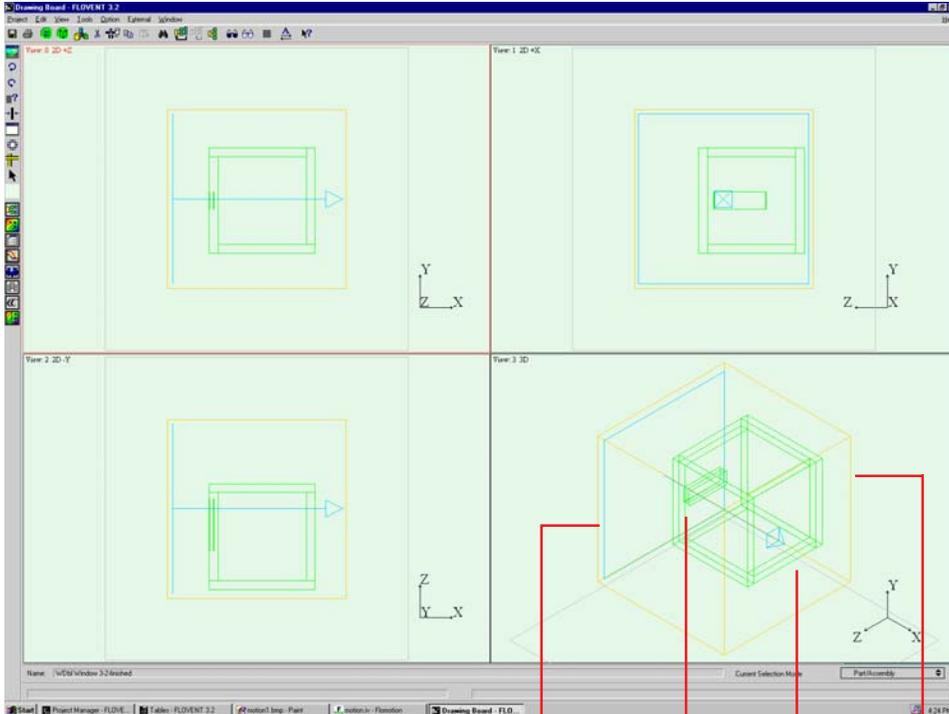
The Control Model is a 3x3x3 meter (interior dimension, the thickness of the wall and roof and floor is 0.3 meter) cubic room with a typical 0.6x1.8 meter double glass window located 1 meter above the interior floor. Two openings (0.02x0.6 meter) are at the bottom and top of outer pane.
