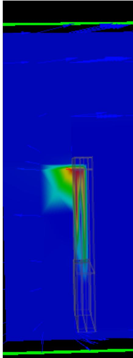
The above image shows temperature distribution across the section of a typical DGF window, where the red color represents higher temperature and the green color represents lower temperature.
