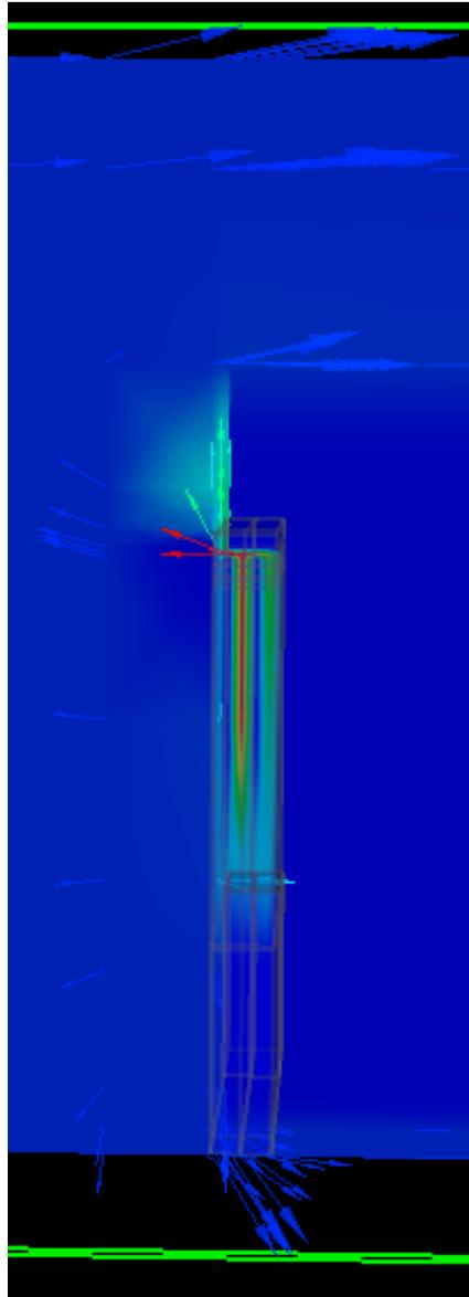
The above image shows temperature distribution across the section of a typical DGF window with wind shield, where red color represents higher temperature and green color represents lower temperature.
