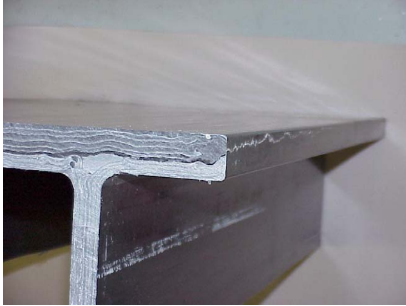
Figure 4.1: Beam Section with Crack
