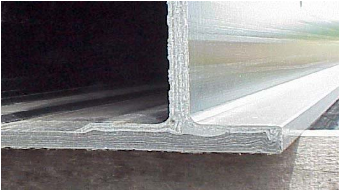
Figure 7.1: Reduced Waviness of the Second Generation Beams
