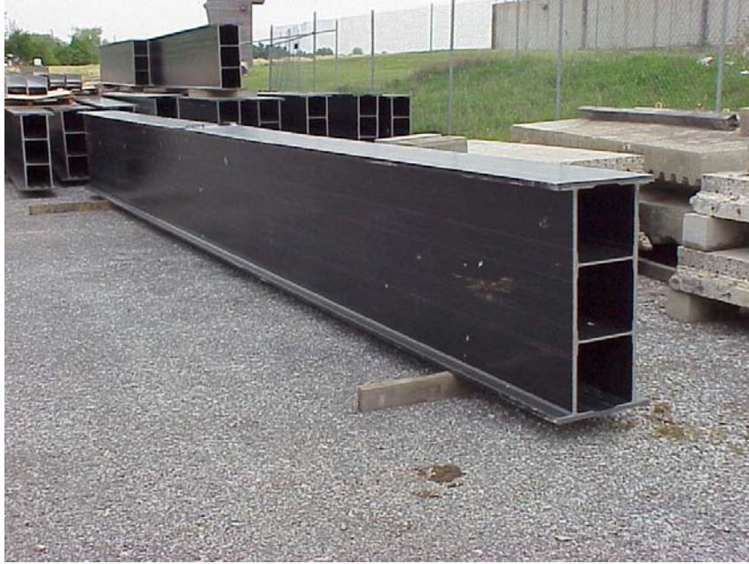
Figure 1.4: Full Length of a Failed Beam
