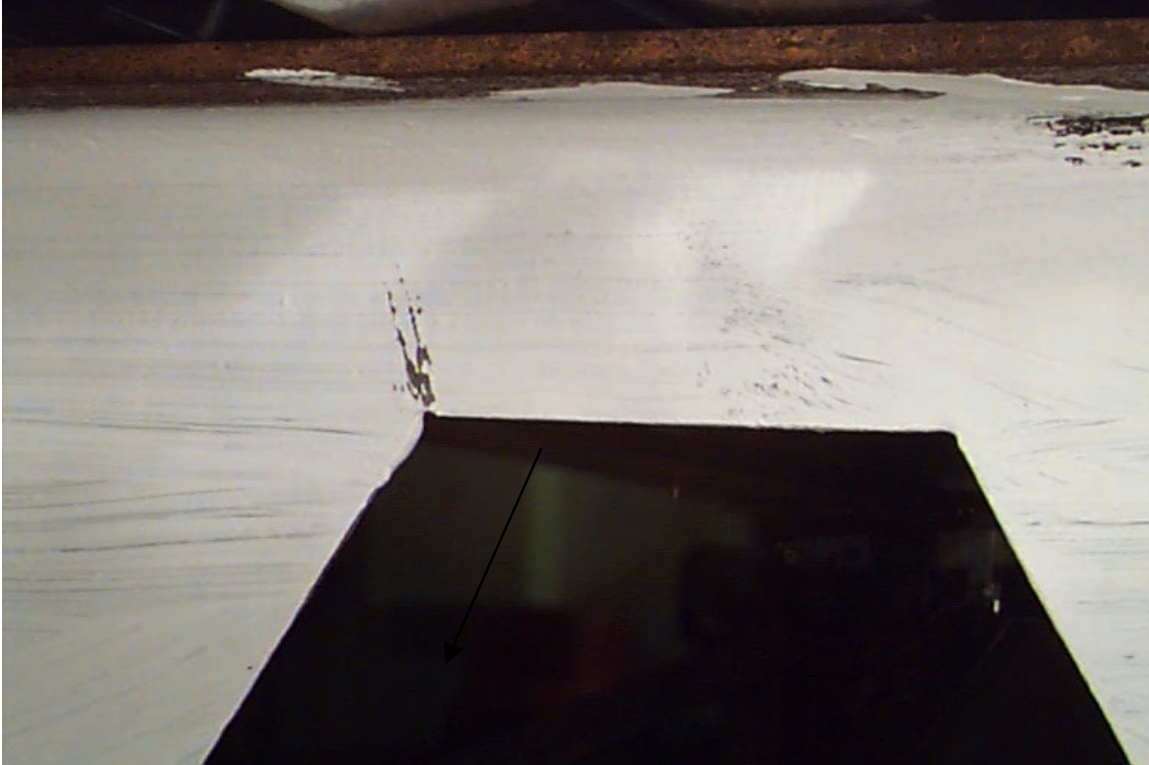
Figure 3.9 Vierendeel Bending White Wash Lines in CB12 x 13 Test
