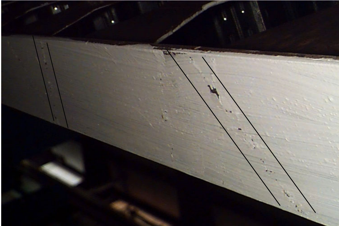
Figure 3.13 Diagonal Streaks on Bottom Flange During CB15 x 15/19 Test
