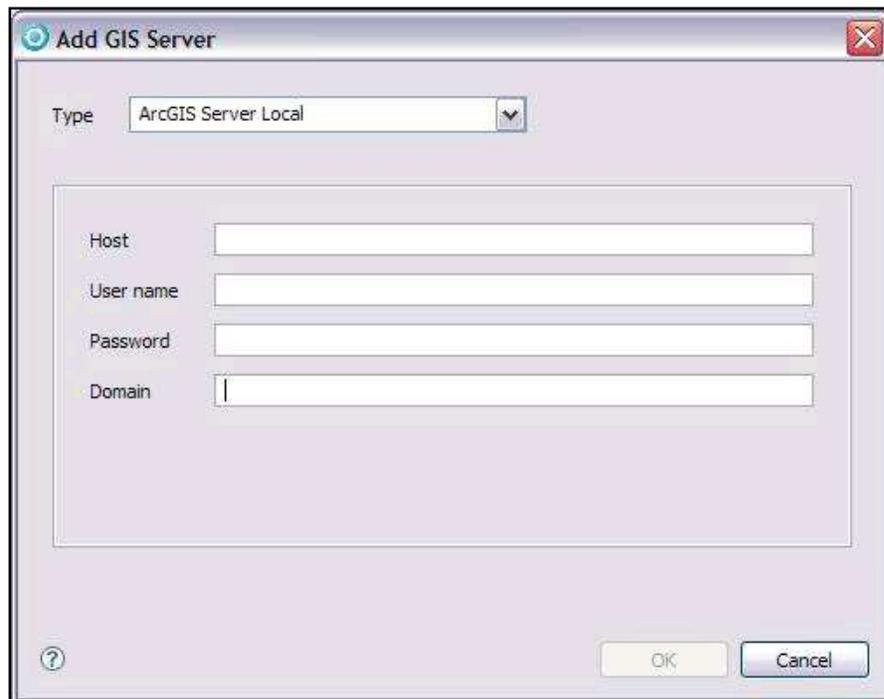
9. Click the OK button to connect to the GIS Server and see a list of valid server objects. Double click on the server object that is to be used and the object will be added under Selected Services on the right hand side. Click Finish to build the project.
