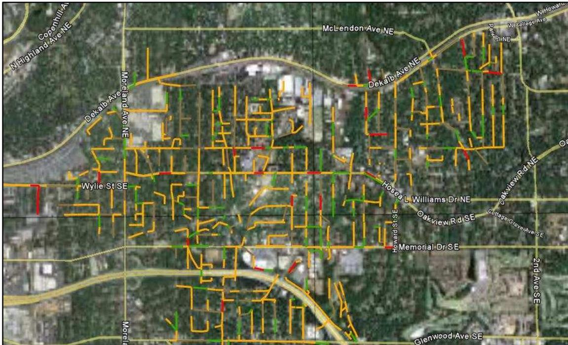
Figure 7: Overlay of risk rated pipes on Google Earth
