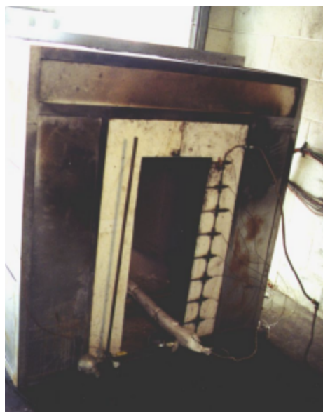
Figure 3.4 Assembled compartment with instrumentation
