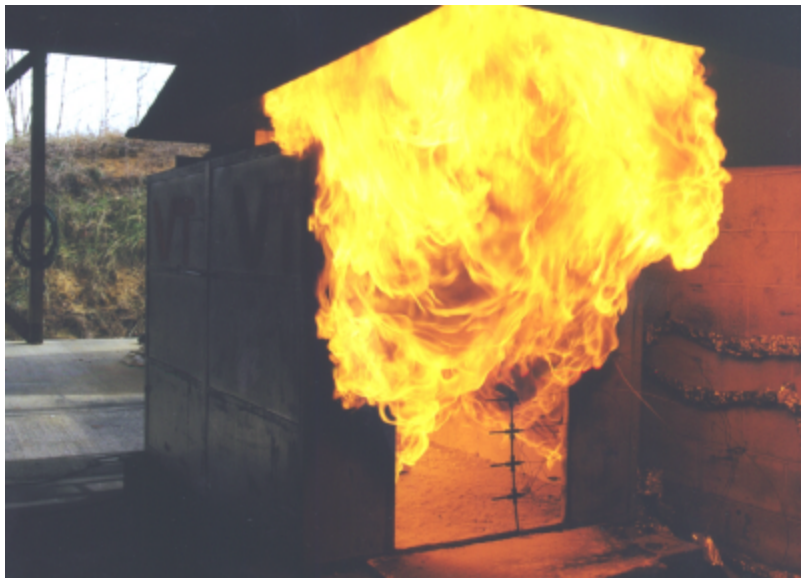
Figure 4.22 Fully developed compartment fire, \phi = 1.28 , showing doorway neutral plane and upper-layer depth
