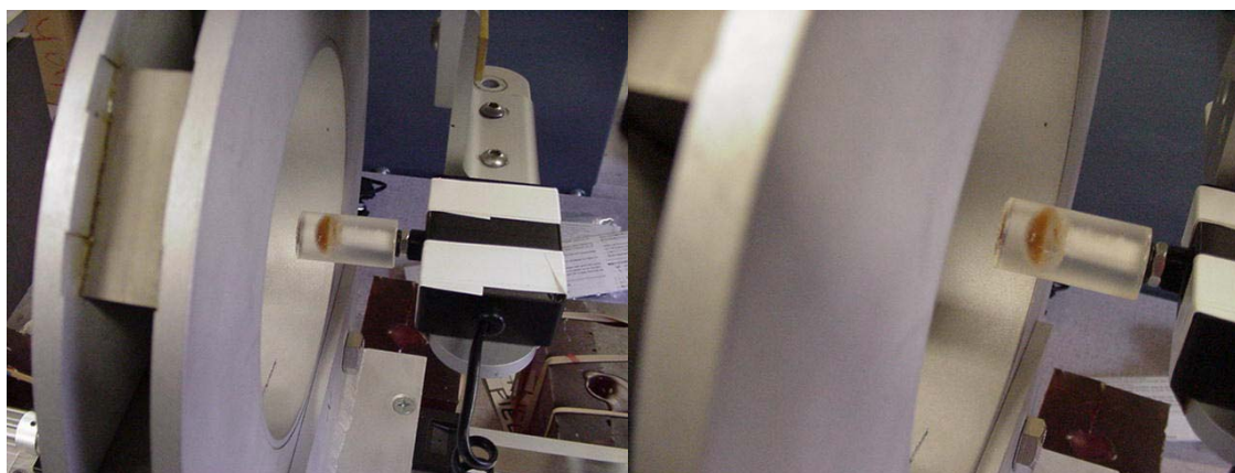
Figure 37. Suspended solution of Dynabeads product 142.04 under static flow conditions.
