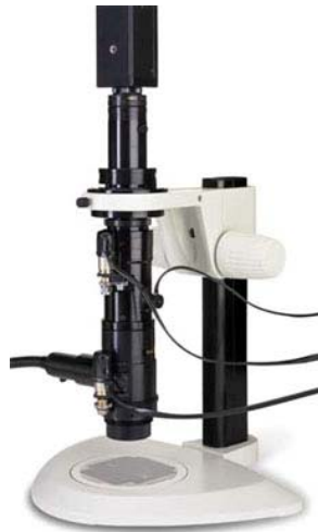
Figure 45. Zoom 160 Optical System modified with non-ferric components capable of micrometer resolution within the magnetic workspace.
