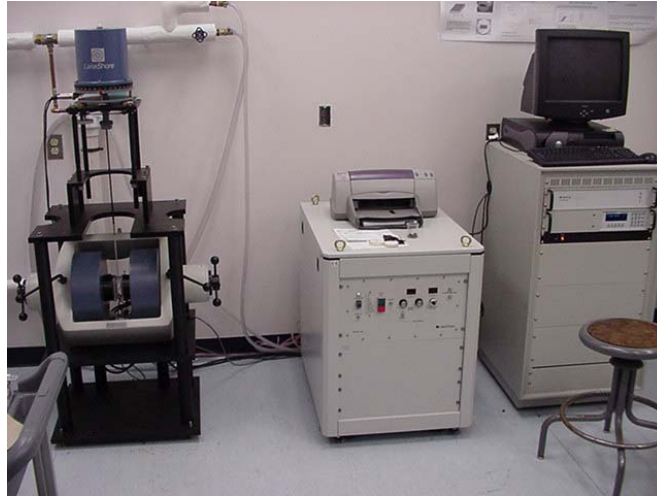
Figure 31. The LakeShore 7300 Vibrating Sample Magnetometer.
