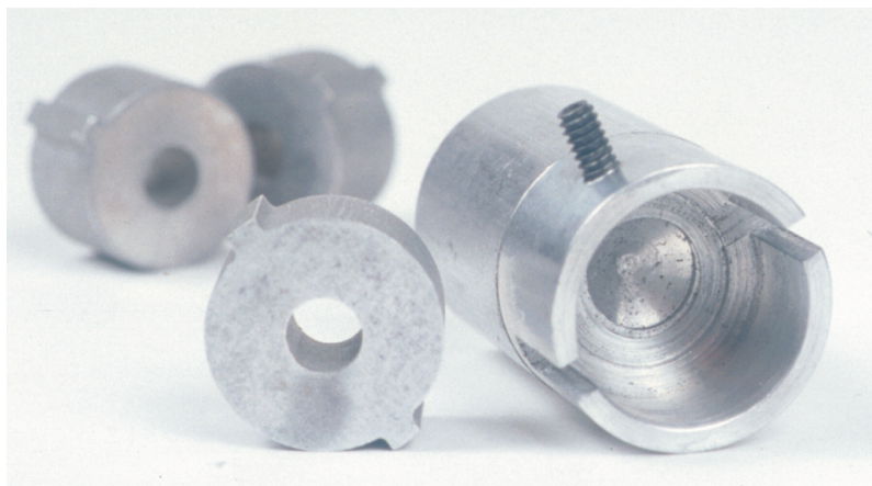
Fixture for machining bearing sleeves and inserts
