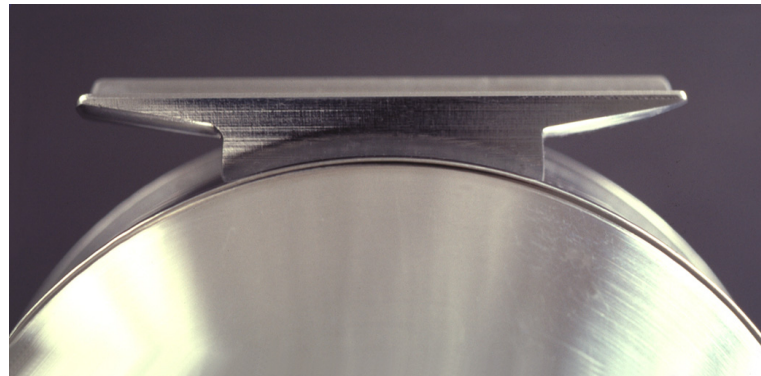
Hand formed taper on reel seat
