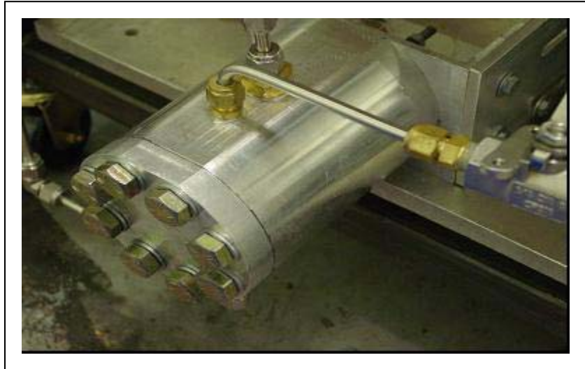
Figure 5.61 Proportional throttling valve used to modulate fuel
