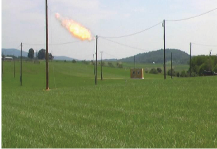
Figure 3.13: Picture of linear charge being detonated to simulate a sonic boom propagating towards the single room structure.
