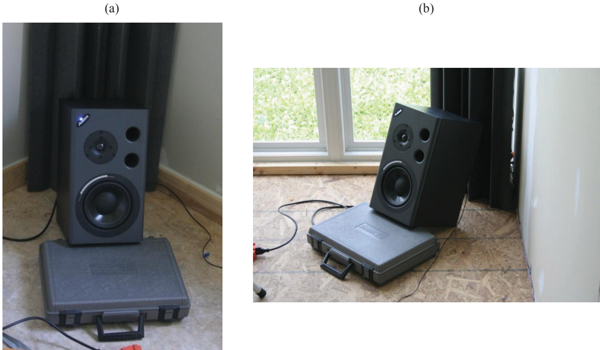
Figure 4.9: Picture of (a) original structure room speaker setup and (b) addition structure room speaker setup used in acoustic modal testing.
