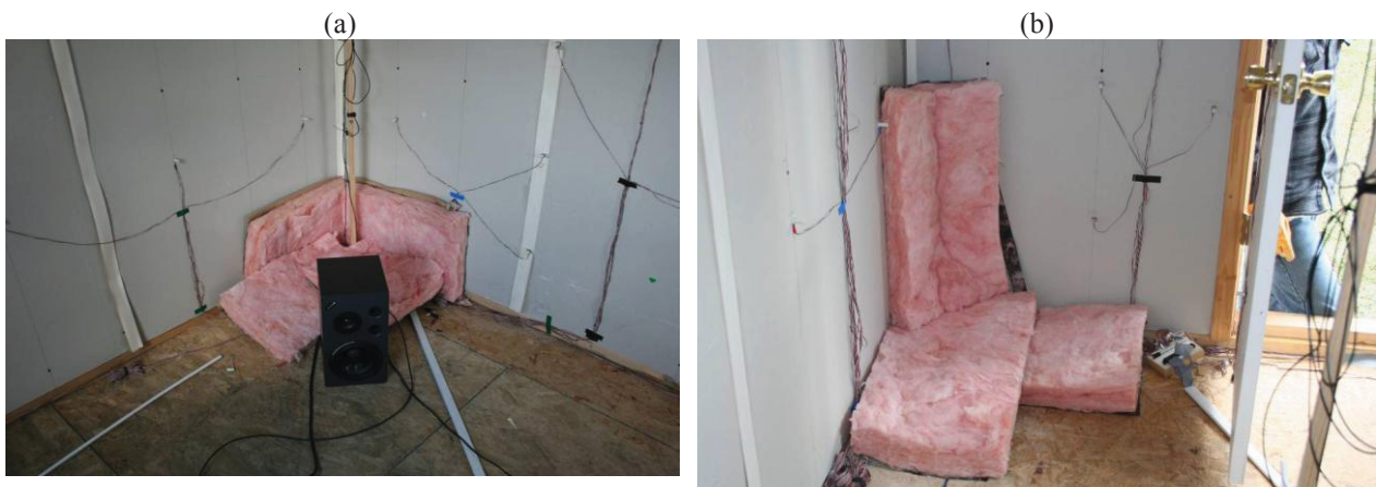
Figure 4.3: Speaker, microphone pole, and insulation damping setup used in acoustic modal testing.
