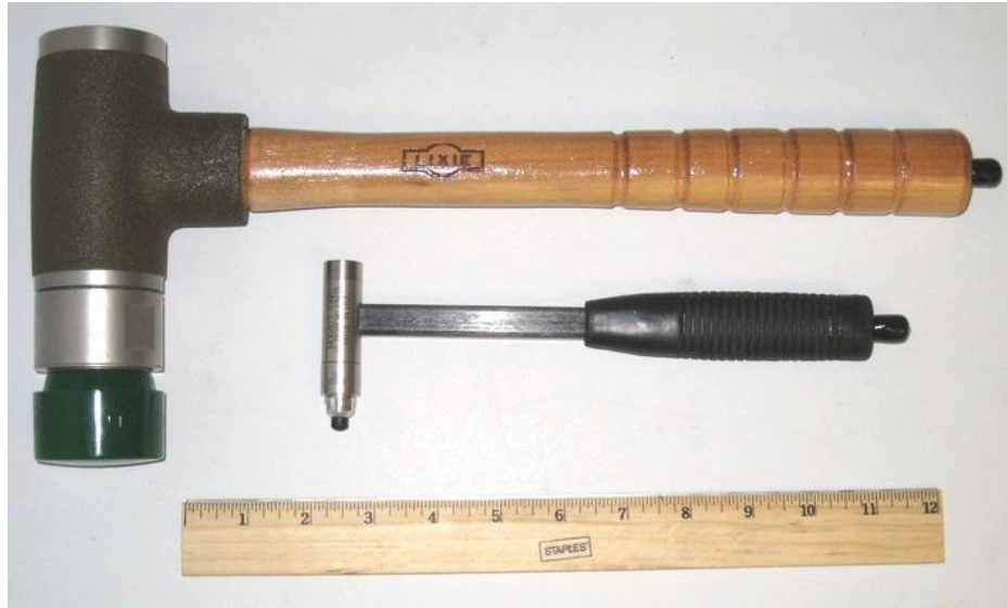
Figure 3.4: Large Brüel and Kjær Modal Sledge Hammer (Type 8208) used to provide impulsive excitation of the test structure's walls and and small PCB Impact Hammer (086C03) used to provide impulsive excitation to the windows and doors of the test structure.
