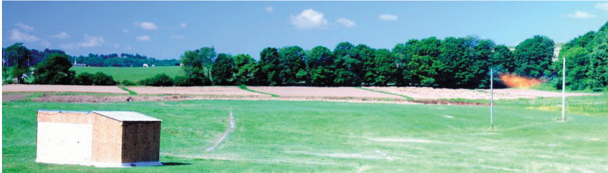
Figure 3.23: Picture of linear charge being detonated to simulate a sonic boom to propagate towards and excite the two room structure.
