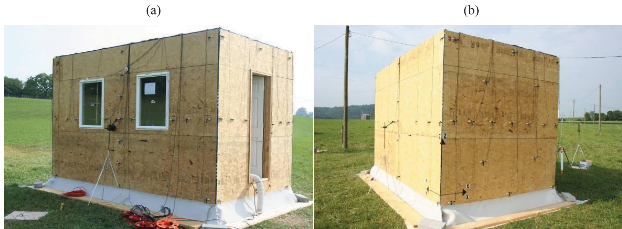
Figure 3.1: (a) Front and (b) back sides of the completely assembled and instrumented single room structure .
