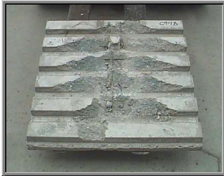
Figure 3.6 Typical Cone Pullout Failure
