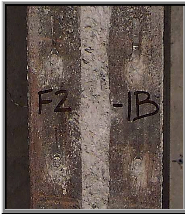
Figure 4.39 Typical Fiction Key Observed in Solid Slab Tests
