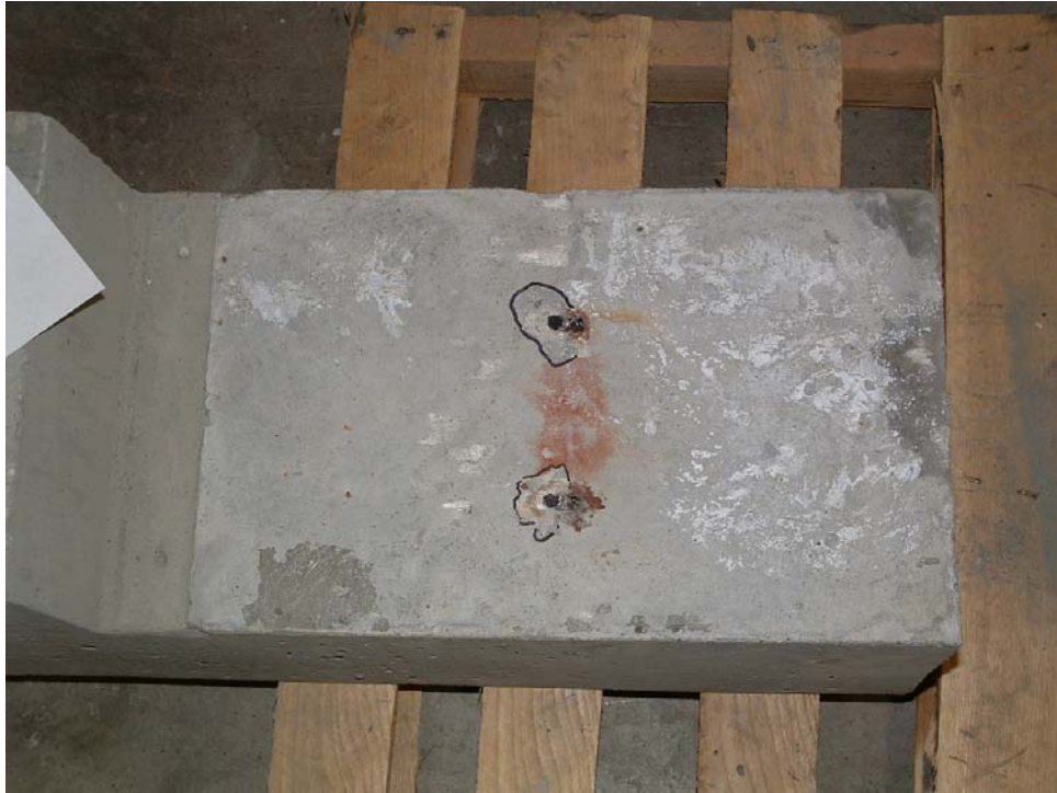
Figure 4.16 Lightweight Side of Double Leg Specimen (After Testing)
