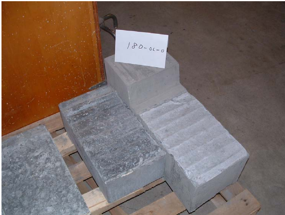
Figure 4.8 Deformed Surface Specimen (After Testing)
