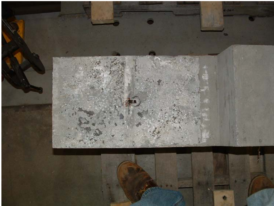
Figure 4.13 Lightweight Side of Single Leg Specimen (After Testing)
