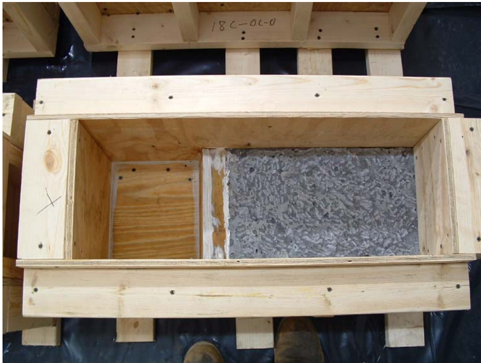
Figure 3.5 Chipped Surface Treatment
