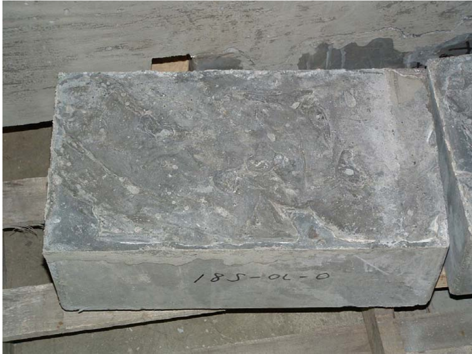
Figure 4.2 Ductal® Side of Smooth Surface Specimen (After Testing)
