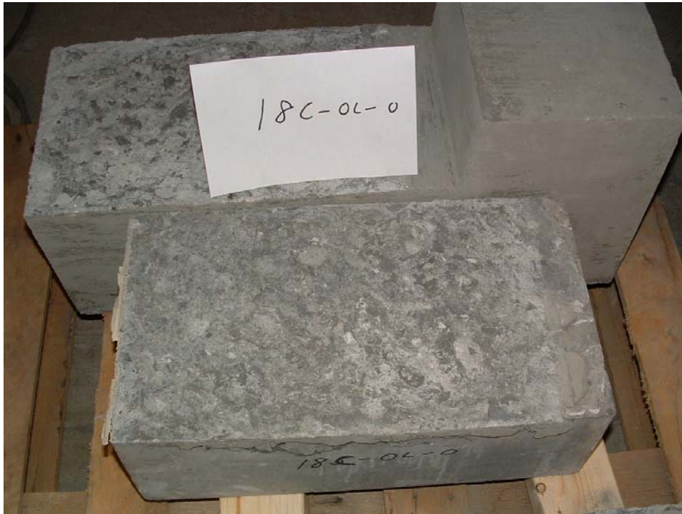
Figure 4.4 Ductal® Side of Chipped Surface Specimen (After Testing)
