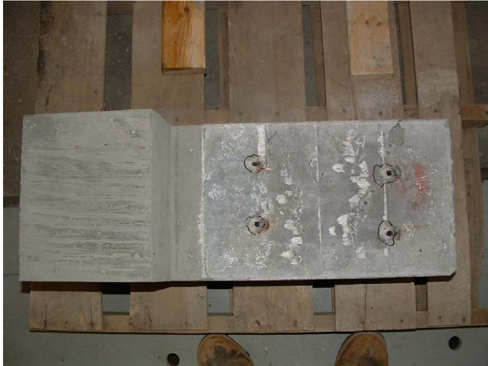
Figure 4.22 Lightweight Side of Four Leg Specimen (After Testing)
