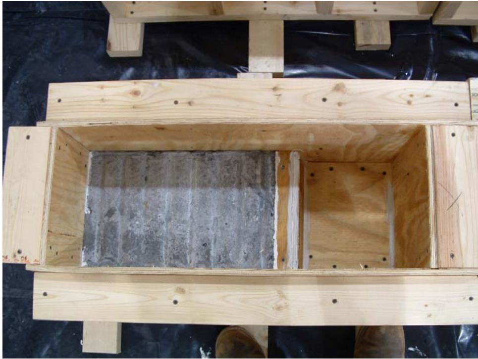
Figure 3.4 Deformed Surface Treatment
