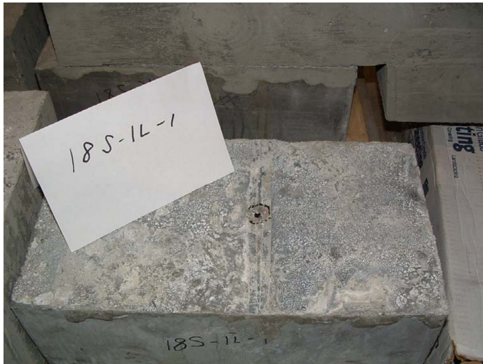
Figure 4.15 Ductal® Side of Single Leg Specimen (After Testing)
